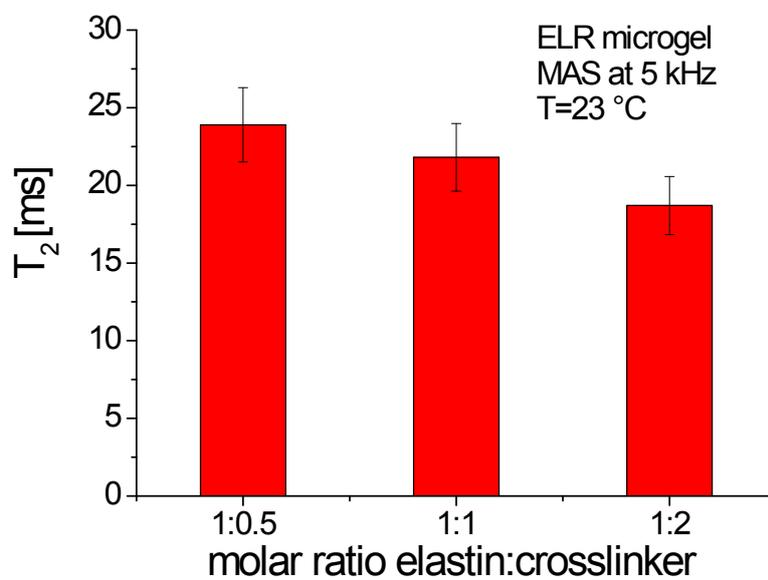
Figure S4. The dependence of transverse magnetization relaxation  $T_2$  upon the molar ratio ELR : PEG-DGE crosslinker. The errors are of the order of 5%.
