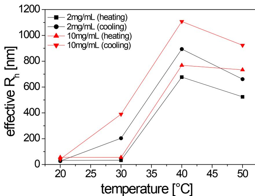
Figure S2. The temperature dependence of the effective hydrodynamic radius  $R_h$ , measured by DLS for ELR microgels with 2 mg/mL and 10 mg/mL concentration. The data for heating and cooling temperatures are connected by continuous lines. The incubation time between successive temperatures was 45 minutes.
