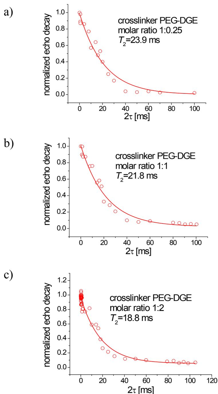
Figure S3. Normalized spin-echo decays for ELR microgels with different molar ratios of ELR : PEG-DGE crosslinker: a) 1:0.25, b) 1:1, and c) 1:2. The measurements were made at 25 °C for a microgel concentration of 5 mg/mL in  $\text{D}_2\text{O}$ . The data points are represented by the  $^1\text{H}$  HRMAS integral intensity of the aliphatic region (0-4.6 ppm) edited by the spin-echo measured under 5 kHz sample rotation at magic angle. The best fit of the data points was
