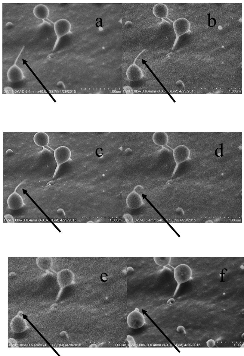
Figure S1. Cryo-FESEM micrographs of ELR microgel with concentration of 2 mg/mL in water incubated at 60 °C for 5 h. The filaments indicated by the arrows are polypeptide fibrils attached to the ELR microgels. The folding behaviour of these filaments after irradiation with the electronic beam for several minutes (5-7min) are shown at successive times in Figures S1 a)-f).
