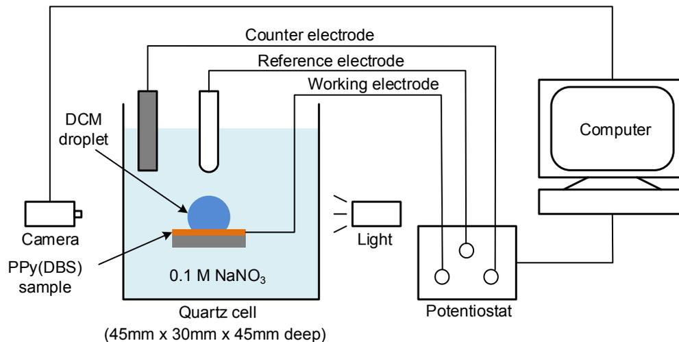
**Fig. S1** Schematic of the experimental setup. The PPy(DBS) samples were placed in a quartz cell filled with 0.1 M NaNO<sub>3</sub>. A copper tape was used as the counter electrode, and a saturated calomel electrode (SCE) was used as the reference electrode. The voltage was applied by using a potentiostat. The organic droplet was monitored through the camera of the goniometer.
