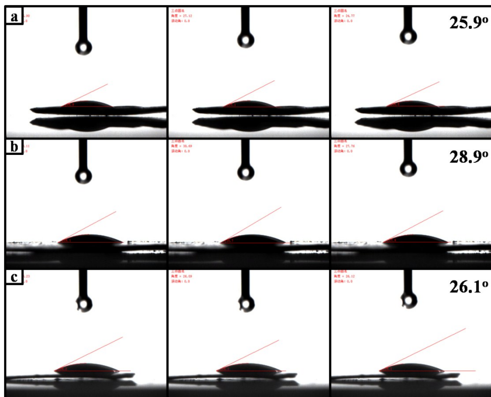
Figure S13. Photographs of contact angle of Ni-BDC (a), Cu-BDC (b) and Zn-BDC (c).
