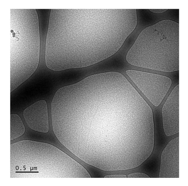
Figure 2: Cryo-TEM image of lact oferrin strings at protein concentration of 80 mg/mL at ionic strength 35 mM and pH 7.
