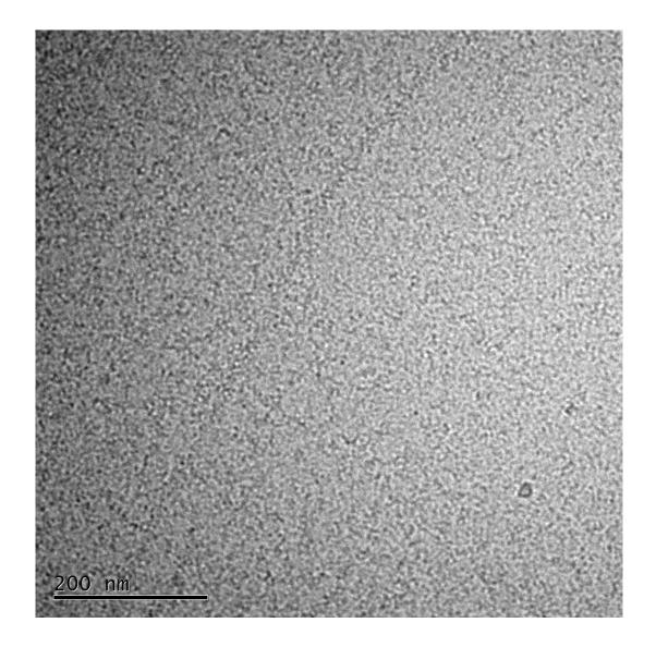
Figure 1: Cryo-TEM image of lactoferrin strings at protein concentration of 80 mg/mL at ionic strength 35 mM and pH 7.
