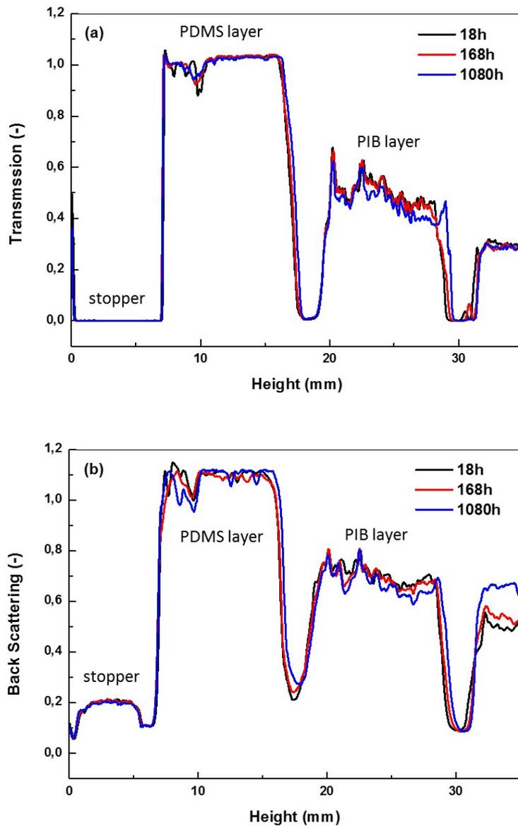
Figure S3. Transmssion (a) and back scattering (b) of PDMS and PIB-particle layers versus sample height at different residence times. Height 0 corresponds to the bottom of the tube.
