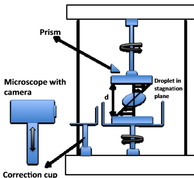
Figure S1. Scheme of counter rotating device.
