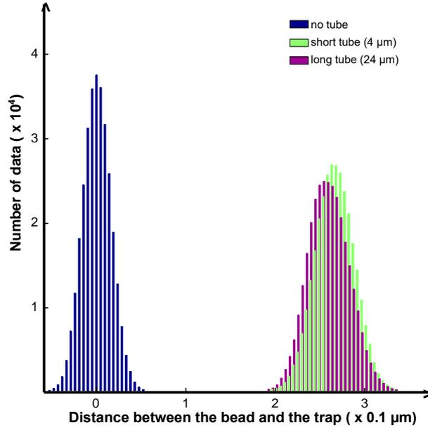
**Figure S3: Distributions of the position of the bead** recorded by the QPD in 5 seconds for different lengths of the same tube. Slopes are measured at  $(-0.28 \pm 0.01) \text{ V} \cdot \mu\text{m}^{-1}$  for the bead not attached to a tube,  $(-0.29 \pm 0.01) \text{ V} \cdot \mu\text{m}^{-1}$  for the bead attached with the short tube, and  $(-0.26 \pm 0.01) \text{ V} \cdot \mu\text{m}^{-1}$  for the long tube.  $k_{\text{trap}} = 35 \pm 2 \text{ pN} \cdot \mu\text{m}^{-1}$ .
