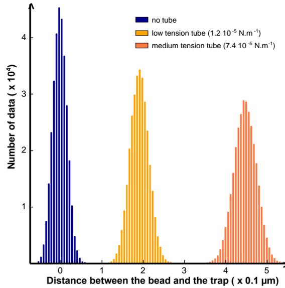
**Figure S4: Distributions of the position of the bead** recorded by the QPD in 5 seconds for different tensions of the same tube. Slopes are measured at  $(-0.24 \pm 0.01) \text{ V} \cdot \mu\text{m}^{-1}$  for the bead not attached to a tube,  $(-0.21 \pm 0.01) \text{ V} \cdot \mu\text{m}^{-1}$  for the bead attached with the low tension tube, and  $(-0.23 \pm 0.01) \text{ V} \cdot \mu\text{m}^{-1}$  for the medium tension tube.  $k_{\text{trap}} = 37 \pm 2 \text{ pN} \cdot \mu\text{m}^{-1}$ .
