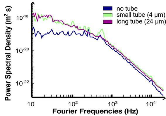
**Figure S7: Effect of tube length on the PSD.** PSD of a free bead (blue) compared to the PSDs of the same bead attached to tube at different length. Slopes are measured at  $(-0.28 \pm 0.01) \text{ V.}\mu\text{m}^{-1}$  for the bead not attached to a tube, and  $(-0.26 \pm 0.01) \text{ V.}\mu\text{m}^{-1}$  for the long tube.  $k_{\text{trap}} = 35 \pm 2 \text{ pN.}\mu\text{m}^{-1}$ .
