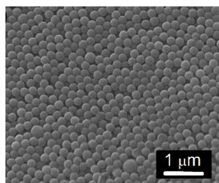
Fig S1 Dried state SEM image showing carboxylate modified latex (CML) particles with 200 nm diameter.
