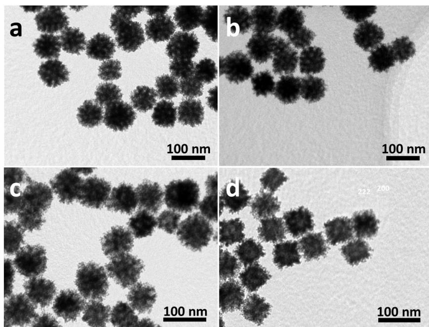
**Fig. S2** TEM images of the nanoporous (a) Pd<sub>21</sub>@Pt<sub>79</sub>, (b) Pd<sub>27</sub>@Pt<sub>73</sub>, (c) Pd<sub>38</sub>@Pt<sub>62</sub>, and (d) Pd<sub>55</sub>@Pt<sub>45</sub> particles.
