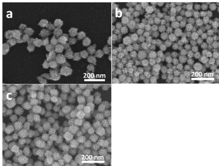
**Fig. S7** SEM images of  $\text{Pd}_{27}@\text{Pt}_{73}$  particles prepared by different amount of KBr ((a) 0 mg, (b) 100 mg, and (c) 300 mg).
