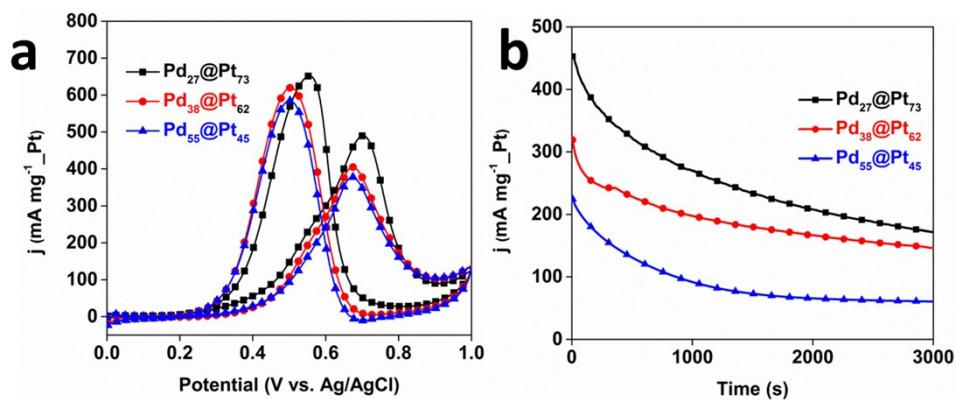
**Fig. S8** (a) Cyclic voltammograms and (b) chronoamperometric curves (recorded at 0.6 V) of the nanoporous  $\text{Pd}_{27}@\text{Pt}_{73}$ ,  $\text{Pd}_{38}@\text{Pt}_{62}$ ,  $\text{Pd}_{55}@\text{Pt}_{45}$  particles obtained in 0.5 M  $\text{H}_2\text{SO}_4$ +0.5 M  $\text{CH}_3\text{OH}$ .
