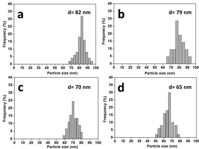
**Fig. S1** Histograms showing the particle size distributions of nanoporous (a) Pd<sub>21</sub>@Pt<sub>79</sub>, (b) Pd<sub>27</sub>@Pt<sub>73</sub>, (c) Pd<sub>38</sub>@Pt<sub>62</sub>, and (d) Pd<sub>55</sub>@Pt<sub>45</sub> particles.
