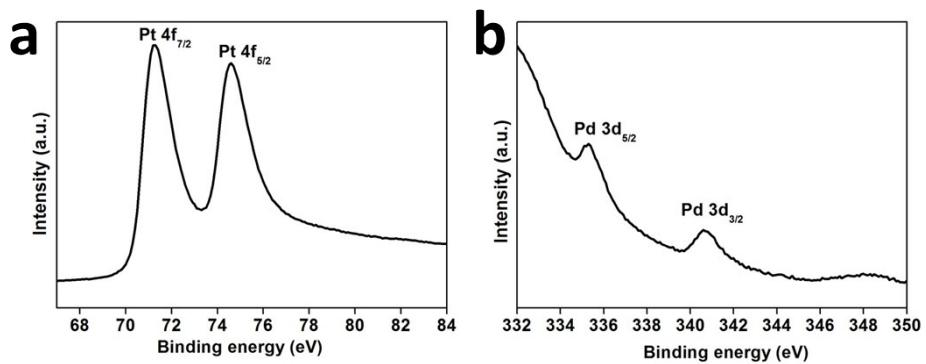
**Fig. S3** High resolution XPS spectra of nanoporous Pd<sub>27</sub>@Pt<sub>73</sub> particles on (a) Pt 4f and (b) Pd 3d.
