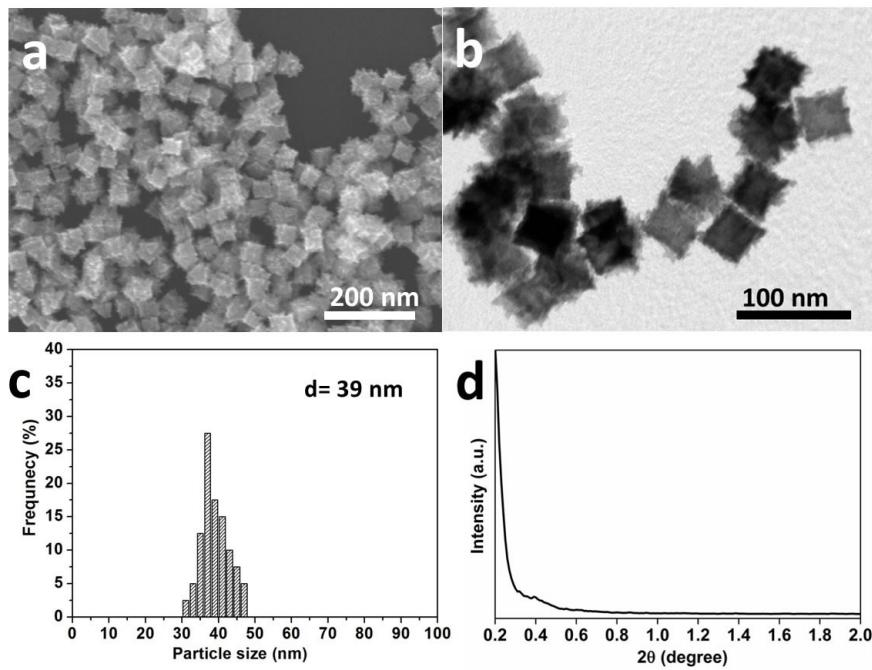
**Fig. S5** (a) SEM image, (b) TEM image, (c) histogram of particle size distribution, and (d) low-angle pattern of  $\text{Pd}_{73}@\text{Pt}_{27}$  particles prepared at a molar ratio of  $\text{Pd}/\text{Pt}=67/33$ . Inset image in the panel (b) shows SAED pattern of the individual particle.
