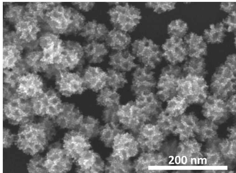
**Fig. S6** SEM image of nanoporous Pt particles prepared in the absence of Pd precursor.
