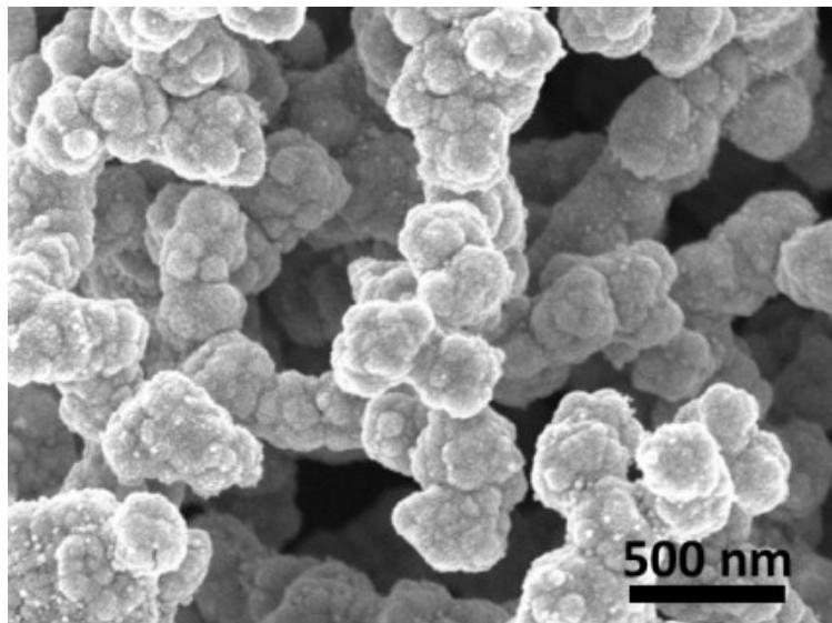
**Fig. S4** SEM image of the sample prepared in the absence of F127.
