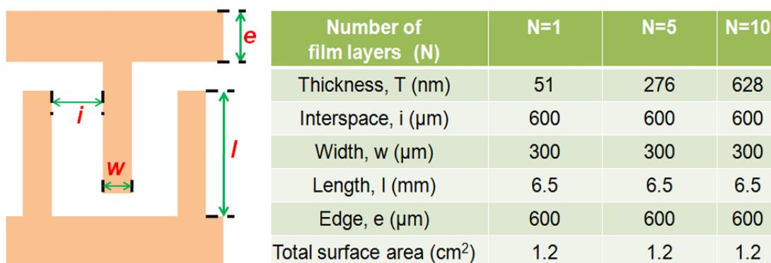
**Fig. S5** Dimensions of the paper-based PEDOT: PSS-CNTs/Ag MSCs produced with the different film layer number (1 layer, 5 layers and 10 layers).
