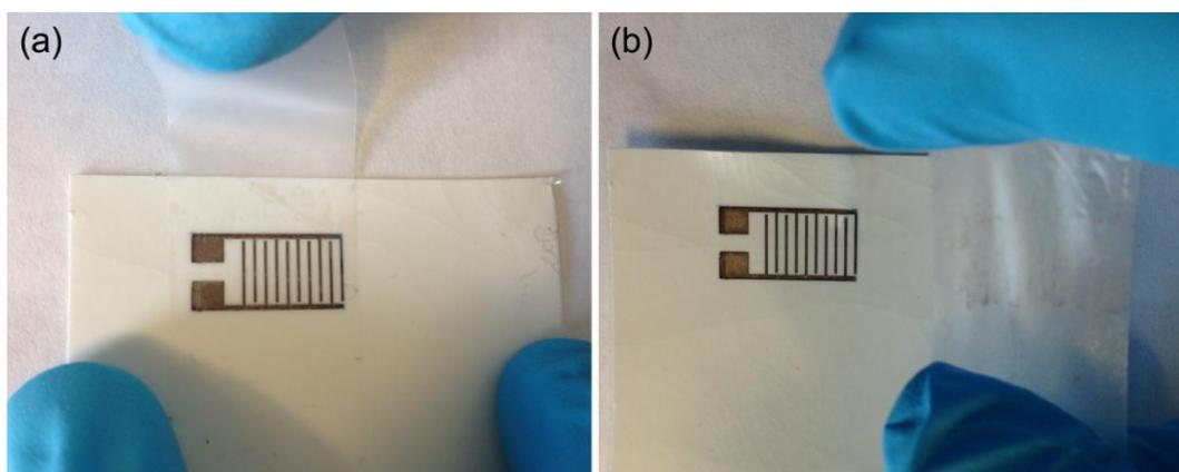
**Fig. S3** ‘Scotch Tape test’ on the paper-based PEDOT: PSS-CNTs/Ag MSCs. The tape before (a) and after (b) peeling demonstrates the strong adhesion between PEDOT: PSS-CNTs/Ag film and paper substrate.
