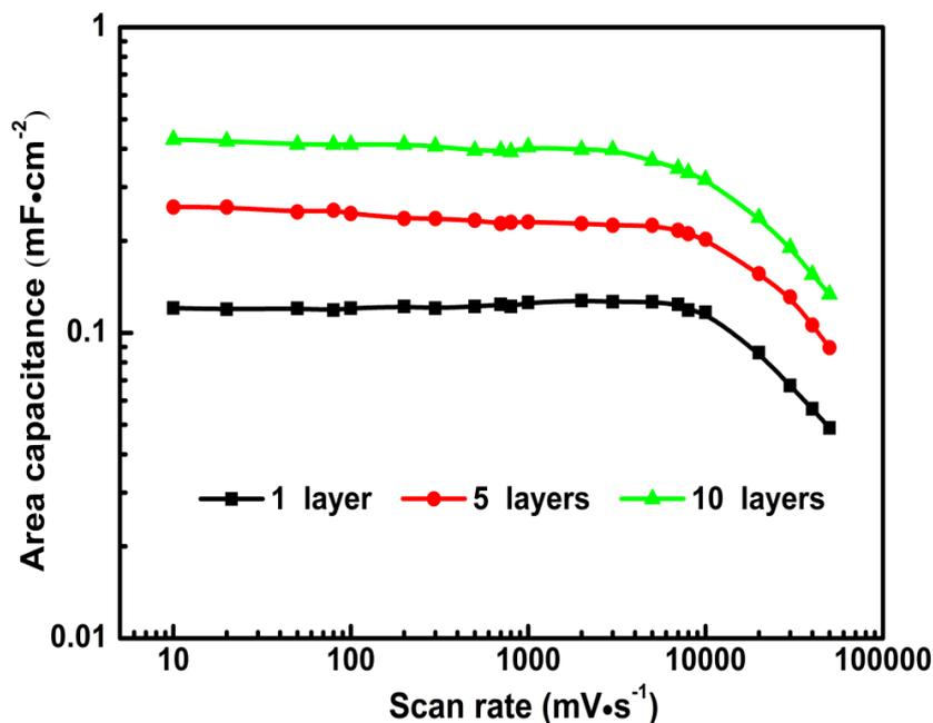
**Fig. S6** Evolution of the area capacitance of paper-based PEDOT: PSS-CNTs/Ag MSCs versus scan rate.
