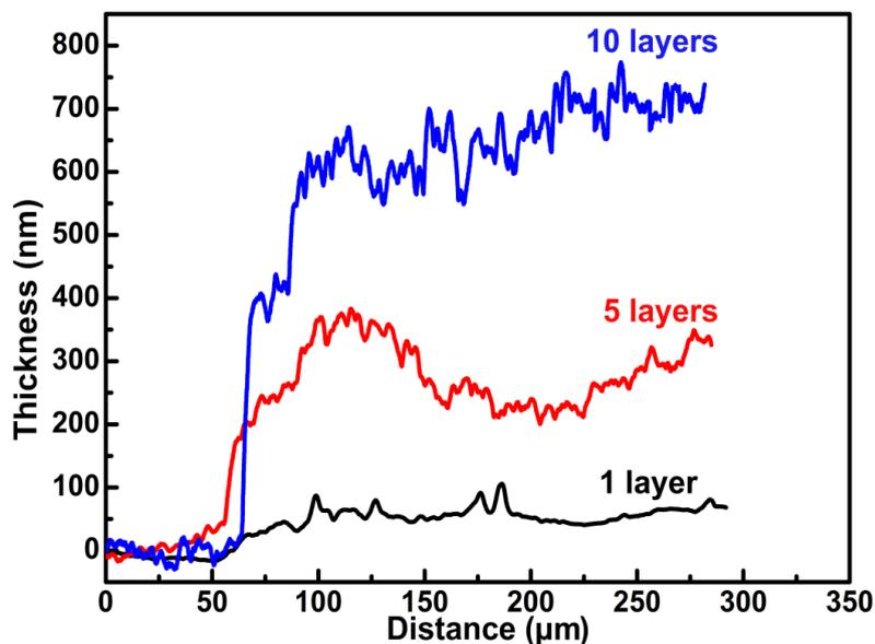
**Fig. S4** Thickness of the paper-based PEDOT: PSS-CNTs/Ag MSCs produced with the different film layer number (1 layer, 5 layers, and 10 layers).
