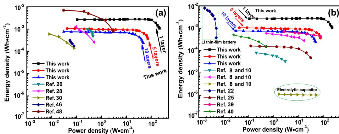
**Fig. S7** Ragone plots showing energy and power densities of paper-based PEDOT: PSS-CNTs/Ag MSCs in comparison to those of (a) reported paper-based MSCs (or SCs) and (b) other micro-supercapacitors and commercially available energy storage devices.
