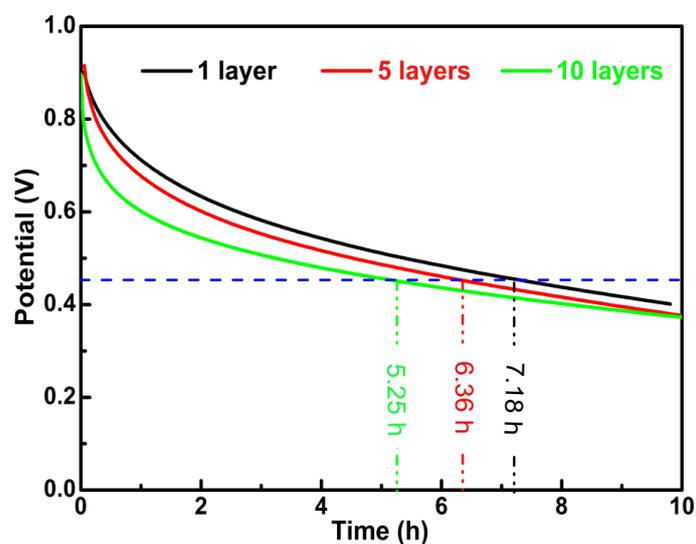
**Fig. S8** Self-discharge curves (open-circuit potential versus time) of paper-based PEDOT: PSS-CNTs/Ag MSCs with different PEDOT: PSS-CNTs film layer number obtained immediately after pre-charged to  $V_{\max}$ .
