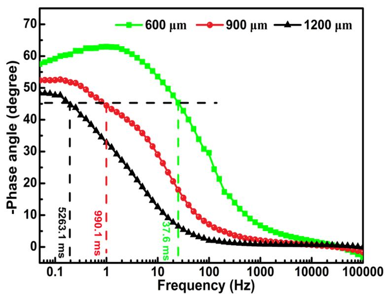
**Fig. S10** Impedance phase angle as a function of frequency ranging from 100 kHz to 0.05 Hz for paper-based PEDOT: PSS-CNTs/Ag MSCs with different inter-space between the adjacent fingers.
