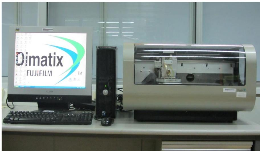
**Fig. S2** The digital photograph of Dimatix DMP-2800 inkjet printer used in this work.
