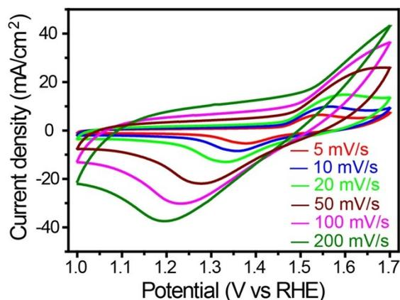
**Figure S6.** CV curves of TiN@Ni<sub>3</sub>N between 1.0 and 1.7 V (vs. RHE) measured at a scan rate of 5 - 200 mV/s in 1 M KOH.
