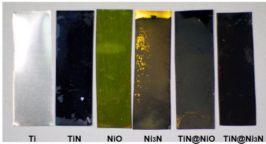
**Figure S3.** Photographs of the as-synthesized samples grown in Ti foils.
