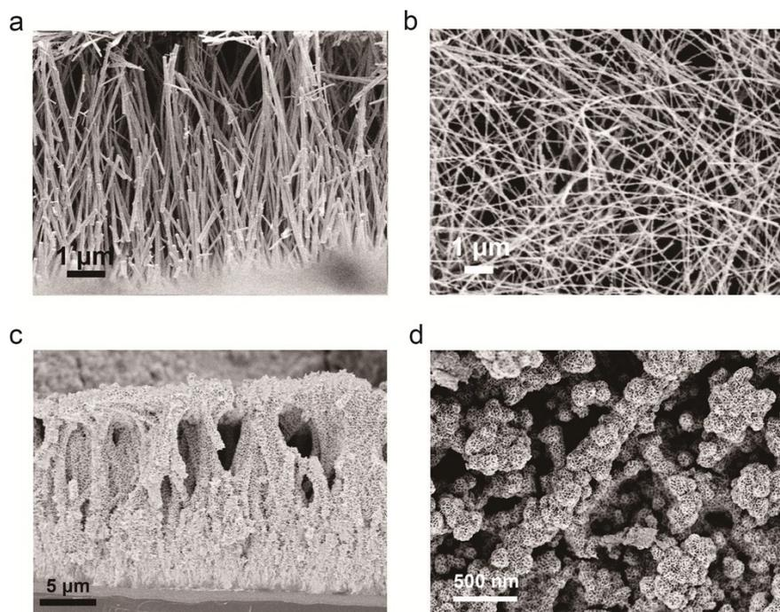
**Figure S1.** SEM images of (a, b) pure TiN nanowires and (c, d) TiN@NiO nanowires.
