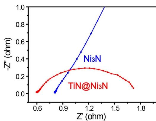
**Figure S8.** Nyquist plots of the TiN@Ni<sub>3</sub>N nanowire arrays and the Ni<sub>3</sub>N nanosheets with enlarged scale.
