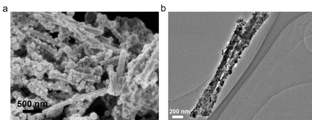
**Figure S9.** (a) SEM and (b) TEM images of the TiN@Ni<sub>3</sub>N nanowires after 10 h of electrocatalytic reaction.
