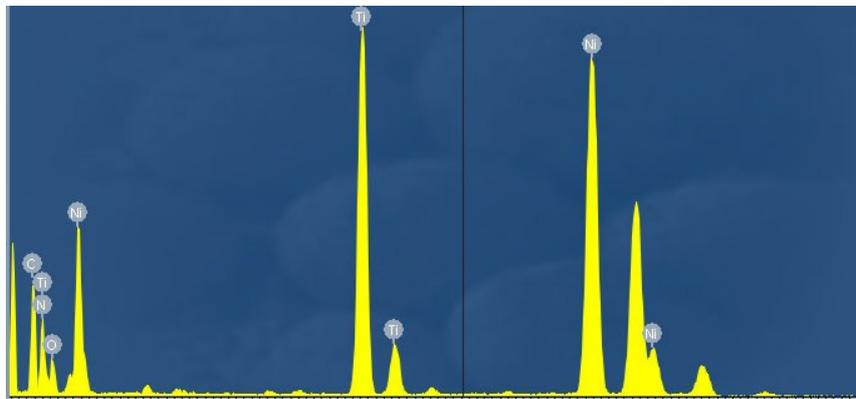
**Figure S4.** EDS spectrum of the TiN@Ni<sub>3</sub>N nanowire arrays.
