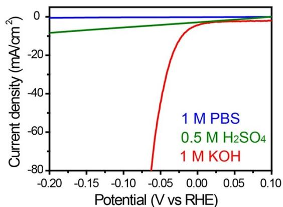
**Figure S7.** LSV curves of TiN@Ni<sub>3</sub>N in neutral electrolyte (blue curve), acid electrolyte (green curve) and alkaline electrolyte (red curve).
