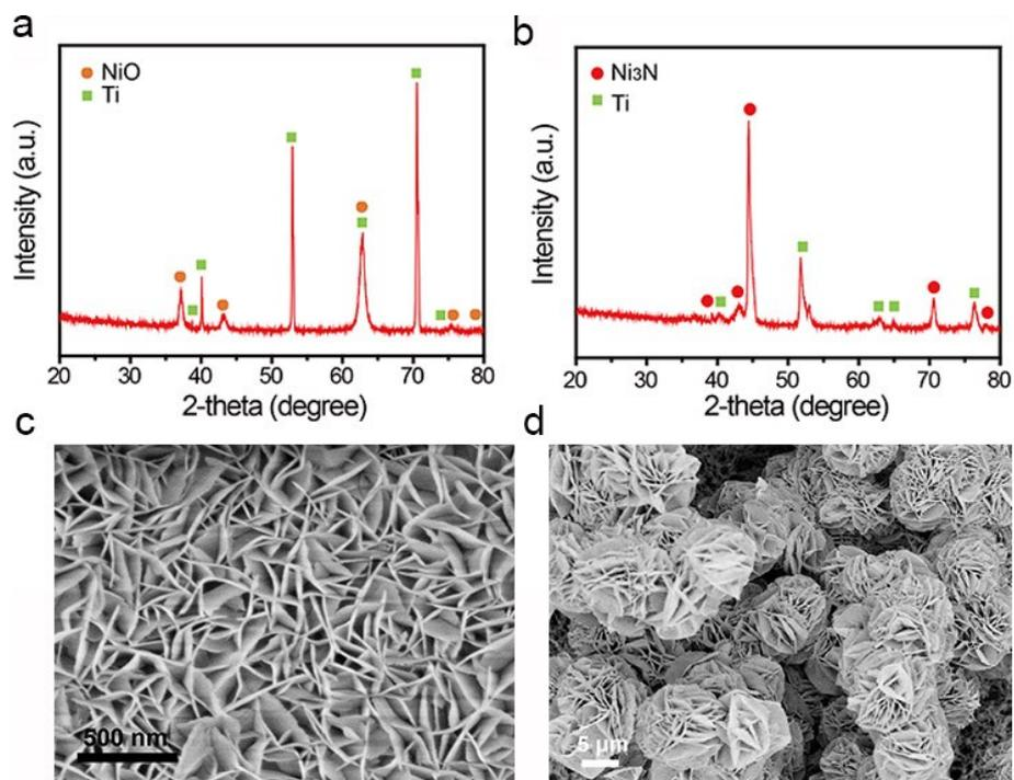
**Figure S2.** XRD patterns of (a) NiO nanosheets (PDF No. 71-1179) and (b) Ni<sub>3</sub>N nanosheets (PDF No. 10-0280), along with the Ti foil substrate. SEM images of (c) NiO nanosheets and (d) Ni<sub>3</sub>N nanosheets grown directly on Ti foil.
