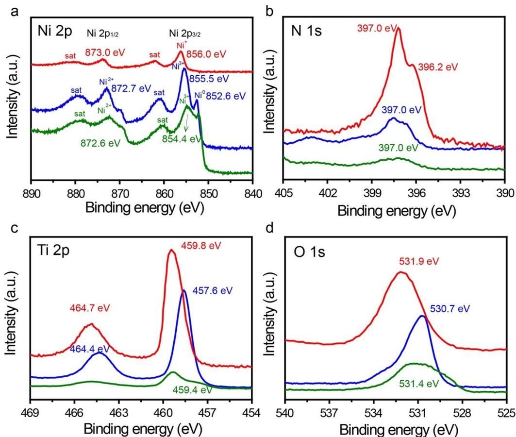
**Figure S5.** High-resolution XPS spectra of (a) Ni 2p, (b) N 1s, (c) Ti 2p and (d) O 1s. Red curves correspond to the as-prepared samples. Blue curve correspond to the post-HER samples. Green curves correspond to the post-OER samples.
