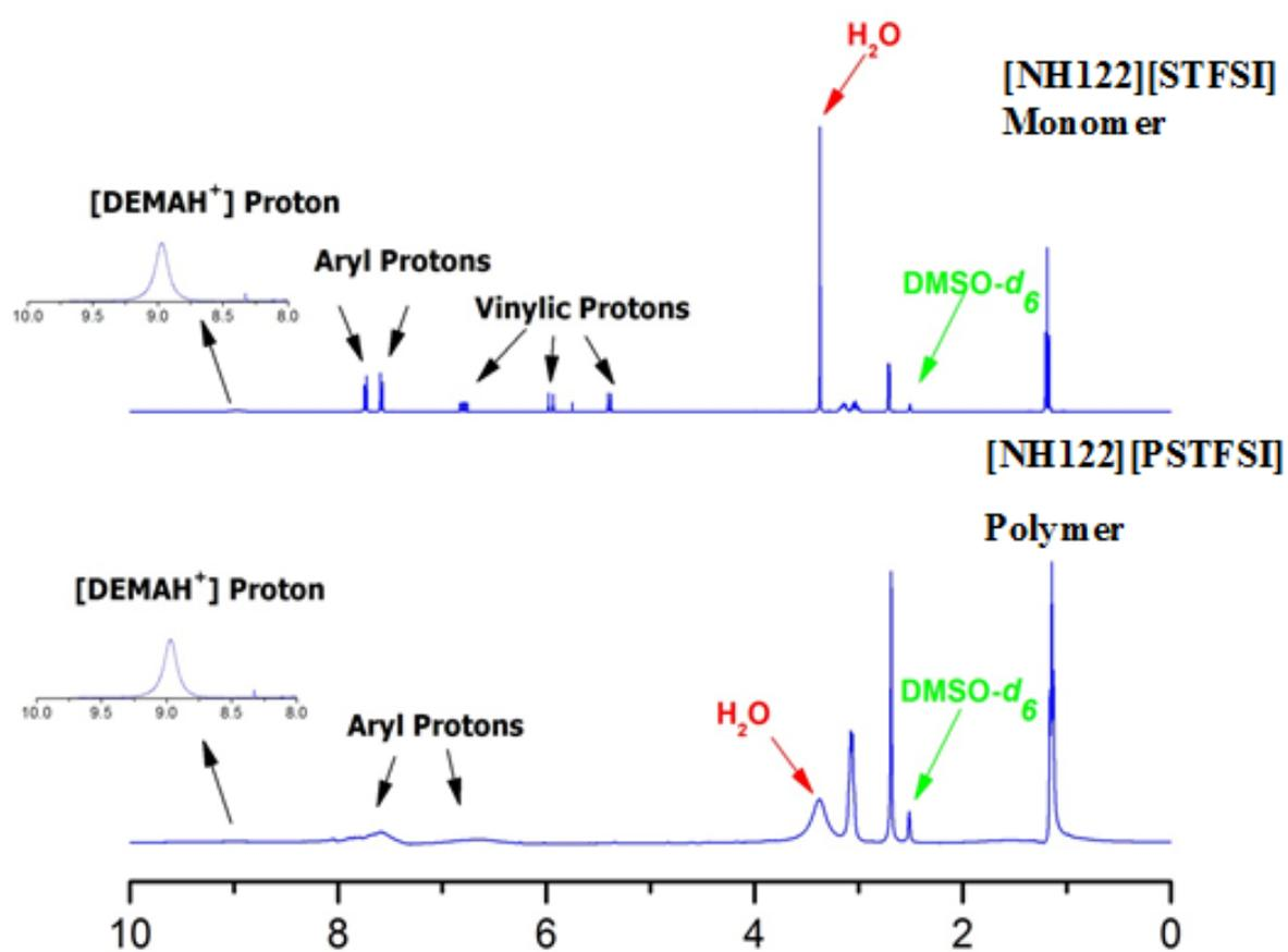
**Fig. S3** Comparison of the solution NMR of the monomer [NH122][STFSI] and poly[NH122][STFSI].
