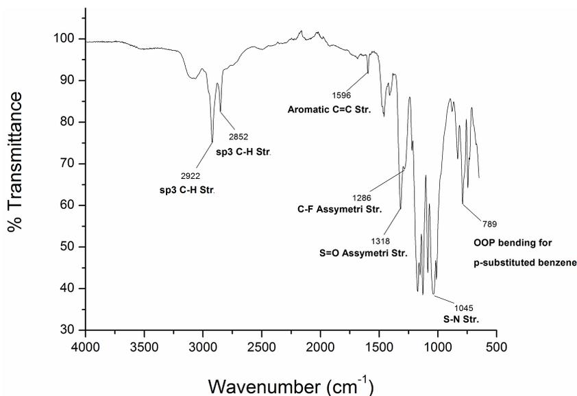
**Fig. S2** ATR-FTIR spectrum of poly([NH122][STFSI]).
