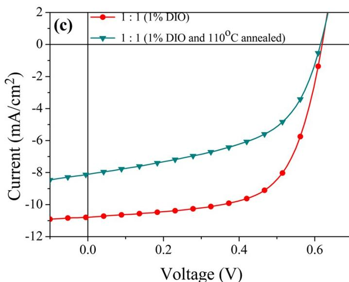
**Fig. S4.**  $J$ - $V$  characteristics of the TPADPP<sub>2</sub>Py/PC<sub>71</sub>BM based OPV cells under AM.1.5G illumination (100 mW/cm<sup>2</sup>): (a) D/A ratio optimization; (b) DIO optimization; (c) annealing temperature optimization. The optimized condition is D/A ratio of 1:1 with 1% DIO without annealing.
