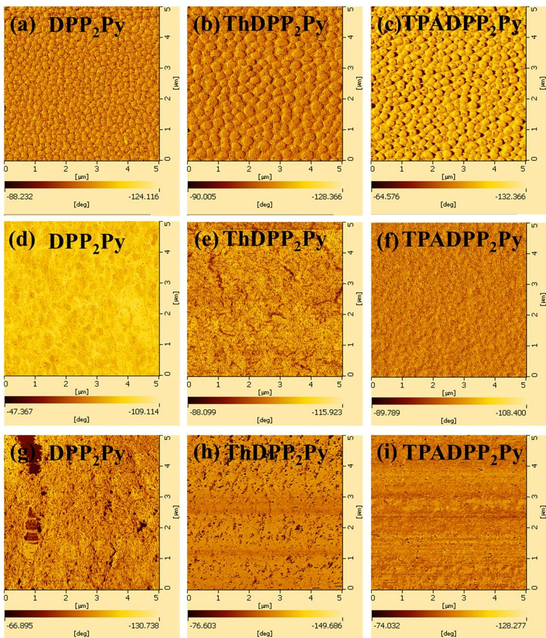
**Fig. S6.** AFM phase images (5×5 μm) of the SMs/PC<sub>71</sub>BM (1:1) blend films (a-c); SMs/PC<sub>71</sub>BM (1:1) with 1% DIO (d-e); SMs/PC<sub>71</sub>BM (1:1) with 1% DIO and annealed at 110 °C for 10 minutes (g-i); respectively.
