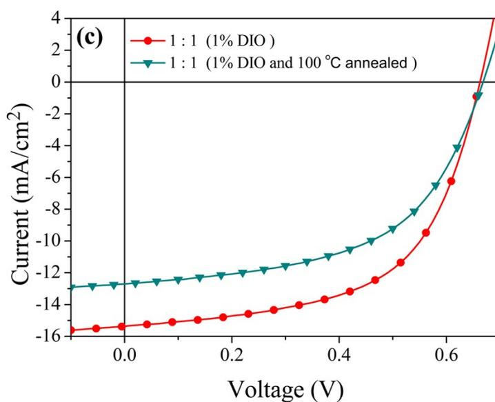
**Fig. S3.**  $J$ - $V$  characteristics of the ThDPP<sub>2</sub>Py/PC<sub>71</sub>BM based OPV cells under AM.1.5G illumination (100 mW/cm<sup>2</sup>): (a) D/A ratio optimization; (b) DIO optimization; (c) annealing temperature optimization. The optimized condition is D/A ratio of 1:1 with 1% DIO without annealing.
