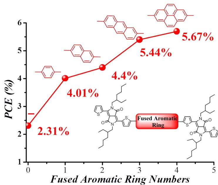
**Fig. S5.** Graphical comparison of DPP<sub>2</sub>Py/PC<sub>71</sub>BM and other DPP<sub>2</sub>Ar/PC<sub>71</sub>BM based OPV cells
