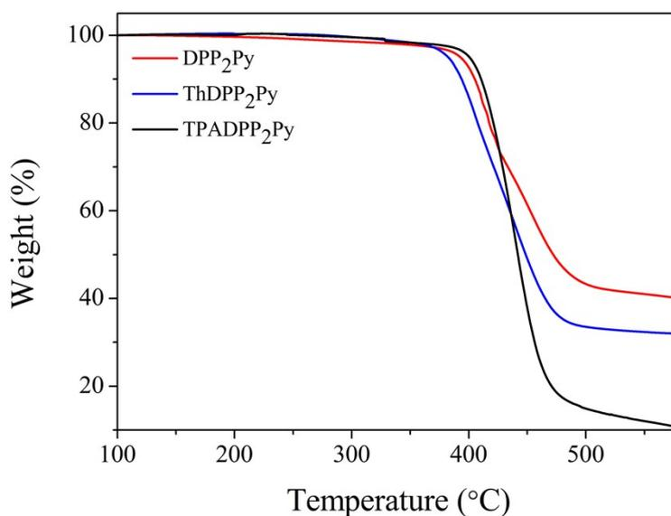
**Fig. S1.** The TGA curves of DPP<sub>2</sub>Py, ThDPP<sub>2</sub>Py and TPADPP<sub>2</sub>Py.
