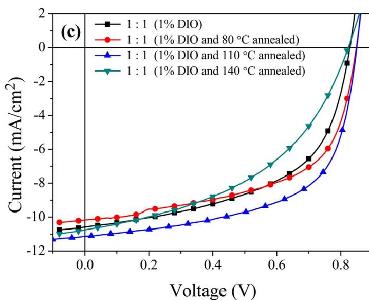
**Fig. S2.**  $J$ - $V$  characteristics of the DPP<sub>2</sub>Py/PC<sub>71</sub>BM based OPV cells under AM.1.5G illumination (100 mW/cm<sup>2</sup>): (a) D/A ratio optimization; (b) DIO optimization; (c) annealing temperature optimization. The optimized condition is D/A ratio of 1:1 with 1% DIO and annealed at 110 °C for 10 minutes.
