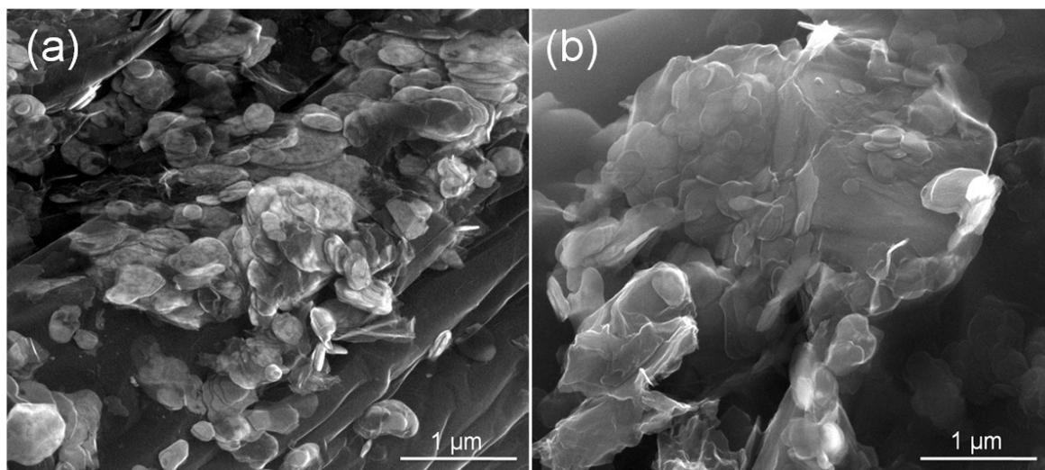
**Figure S5.** Comparative SEM images of GOBN5-750 electrocatalyst (a) before and (b) after durability test at 10000 cycles.
