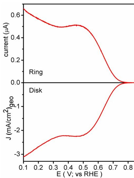
**Figure S3.** Disk current (bottom) and the corresponding ring current (top) for GOBN5-750 catalyst using RRDE at 1600 rpm in  $\text{O}_2$ -saturated 0.1 M KOH solution; (geo: geometric current density, sweep rate 10 mV/s).
