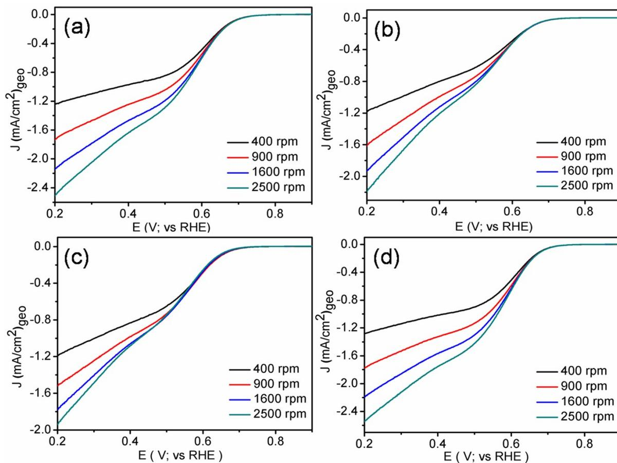
**Figure S4.** ORR polarization curves for (a) GO-750, (b) GOBN3-750, (c) GOBN7-750 and (d) GOBN10-750, in presence of  $\text{O}_2$ -saturated 0.1 M KOH at 25°C. (geo: geometric current density, sweep rate 10 mV/s).
