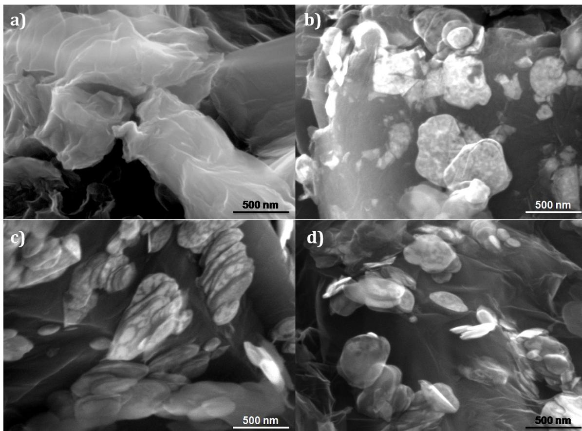
**Figure S1.** (a-d) A typical SEM images comparison of GO-750, GOBN3-750, GOBN7-750 and GOBN10-750 respectively.
