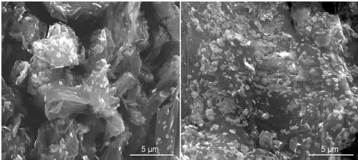
**Figure S2.** A low-magnification SEM image comparison of GOBN5 nanocomposite, before (left) and after (right) heat treatment at 750°C.
