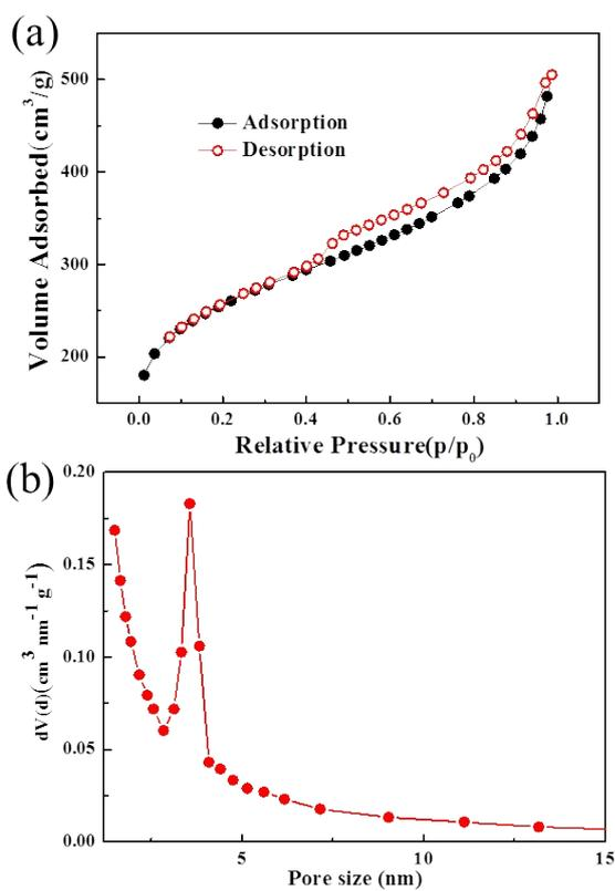
**Fig. S4**  $N_2$  adsorption-desorption isotherms (a) and corresponding pore size distribution calculated from desorption branch by the BJH method (b) of the as-prepared  $B_2O_3$ /carbon microtubes composite.
