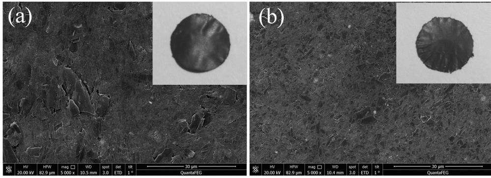
**Fig. S13** SEM images of the compressing pieces of interlayer. (a)  $B_2O_3$ /carbon microtubes composite; (b) carbon microtubes.
