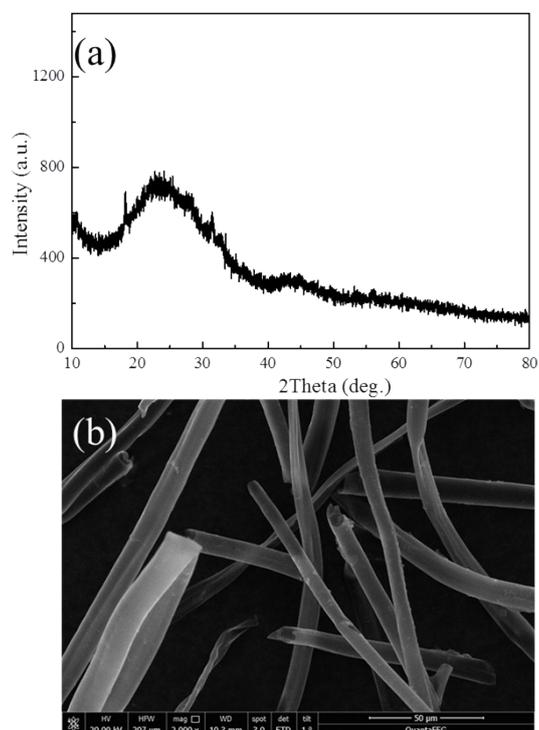
**Fig. S12** XRD pattern (a) and SEM image (b) of the B<sub>2</sub>O<sub>3</sub>/carbon microtubes composite after washing B<sub>2</sub>O<sub>3</sub>.
