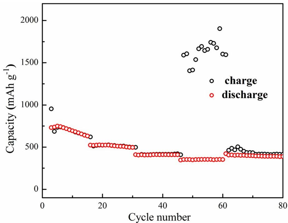
**Fig. S11.** Cycle performance of sulfur cathode at various rates with pure carbon microtubes interlayer (1<sup>st</sup>-15<sup>th</sup>: 0.5C; 16<sup>th</sup>-30<sup>th</sup>: 1C; 31<sup>th</sup>-45<sup>th</sup>: 2C; 46<sup>th</sup>- 60<sup>th</sup>: 4C; 60<sup>th</sup>-80<sup>th</sup>: 2C).
