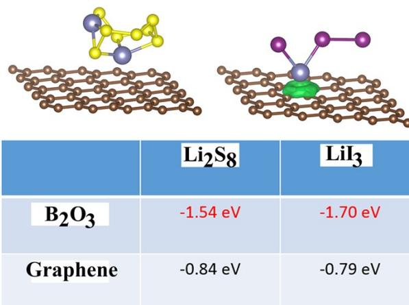
**Fig. S1.** The view of  $\text{Li}_2\text{S}_8$  and  $\text{LiI}_3$  adsorbed on graphene carbon materials and the calculated adsorption energy.
