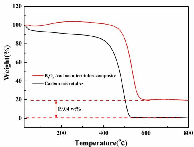
**Fig. S6** TGA curves of prepared  $B_2O_3$ /carbon microtubes composite and pure carbon microtubes.
