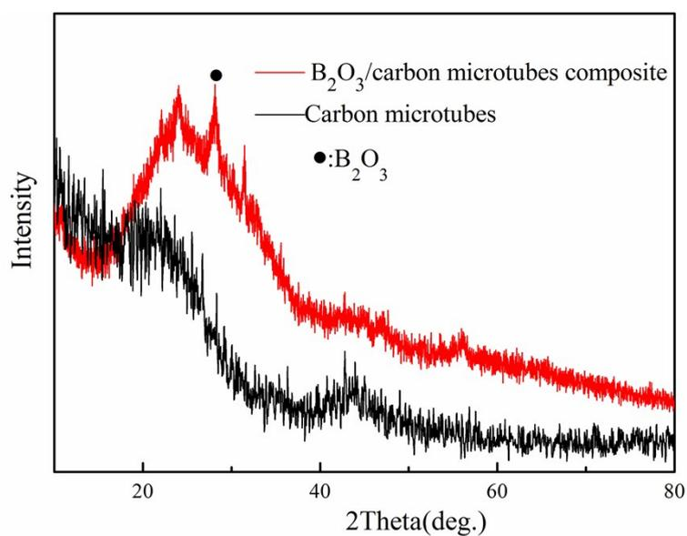
**Fig. S2.** XRD patterns of the prepared  $\text{B}_2\text{O}_3$ /carbon microtubes composite and pure carbon microtubes.
