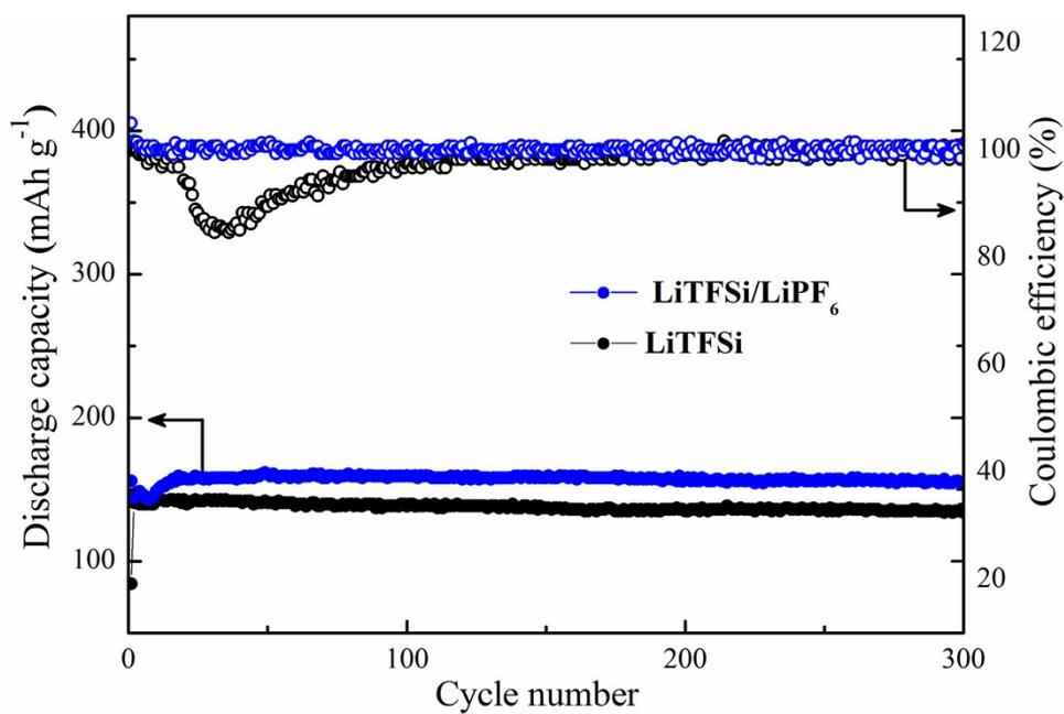
**Fig. S7.** Cycle performance of iodine cathodes in different electrolytes at the rate of 20 C.
