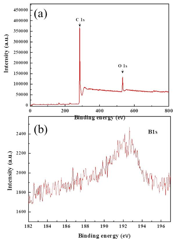
**Fig. S5** XPS survey scan (a) and high resolution scan of B 1s of  $B_2O_3$ /carbon microtubes composite.
