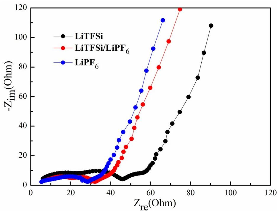
**Fig. S8.** The Nyquist plots of the Li-I<sub>2</sub> batteries in different electrolytes after 300 cycles at the rate of 20 C.
