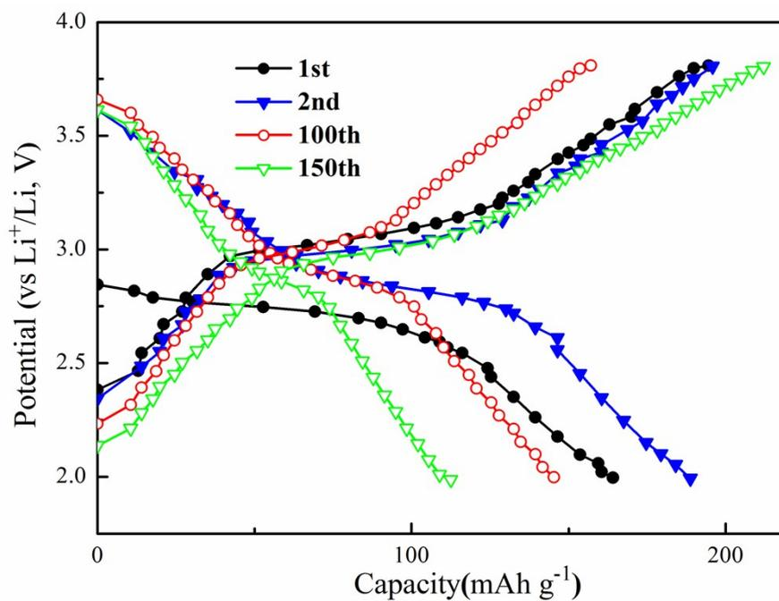
**Fig S10.** The discharge-charge curves of I<sub>2</sub>/B<sub>2</sub>O<sub>3</sub> modified carbon microtubes composite at the rate of 20 C.
