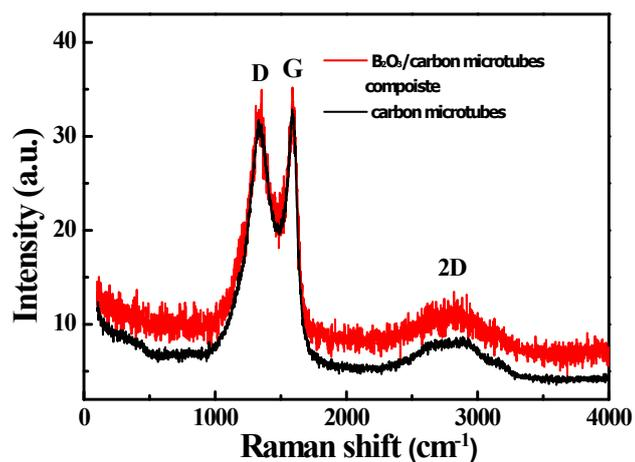
**Fig. S3** Raman spectra of the the prepared  $B_2O_3$ /carbon microtubes composite and pure carbon microtubes.
