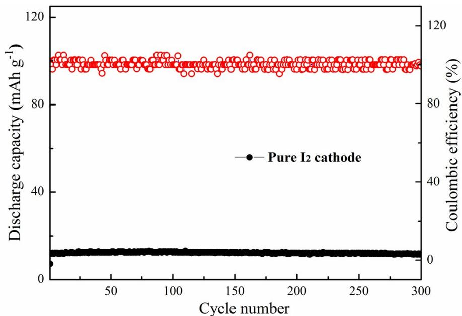
**Fig. S9.** Cycle performance of iodine cathode without interlayer at the rate of 20C.
