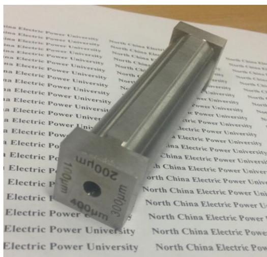
**Figure S1.** The picture of ZBQ four sides wet-film preparation device
