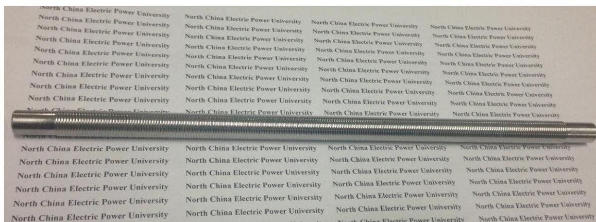
**Figure S2.** The picture of OSP-100 scraping ink bar
