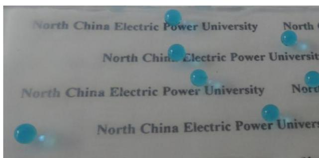
**Figure S3.** Photograph of a FTSN coated glass slide when the ratio of nanoparticles to ethanol is 1:10(w:w). The coated glass slide was placed on a printed paper.
