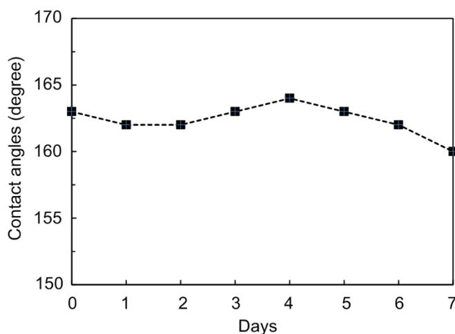
**Figure S5.** Changes in water contact angles under outdoor exposure test for FTSN deposited glass substrate.
