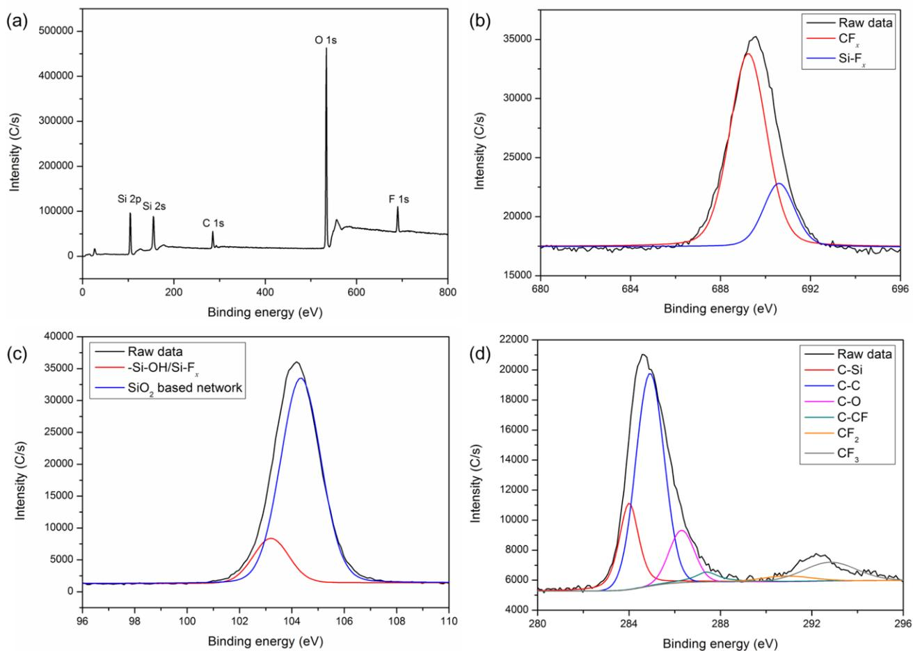
**Figure S6.** (a) Survey XPS spectrum of the FTSN deposited glass substrate; (b) F 1s, (c) Si 2p and (d) C 1s XPS spectrum of the sample.
