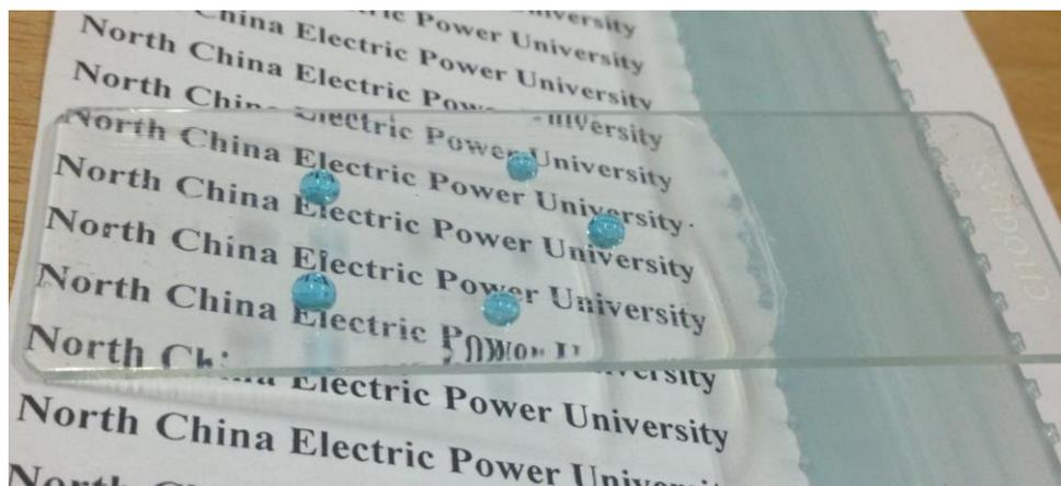
**Figure S4.** Photograph of water droplets on a FTSN coated glass slide after half cycle of abrasion test when the ratio of nanoparticles to ethanol is 1:100(w:w).
