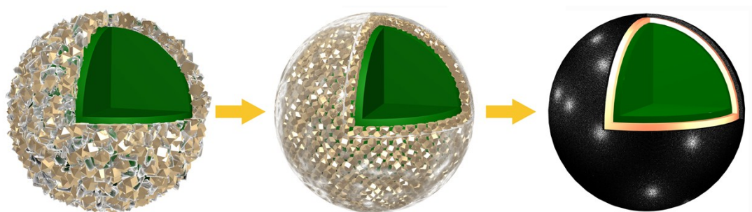
Fig. S1 Schematic formation of the phase separation on the surface of the \text{TiP}_2\text{O}_7 matrix.
