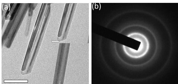
**Fig. S2** (a) TEM micrograph of the MoO<sub>3</sub> nanotubes, and (b) SAED pattern for PPy layer. Scale bar, 200 nm (a), 100nm (inserted in a)
