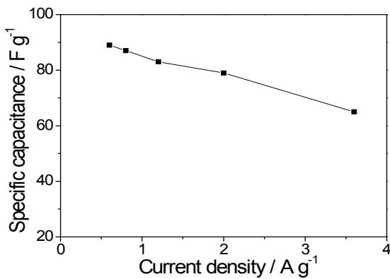
**Fig. S7** Change of capacitance with current densities for the Al-ion capacitor (PPy@MoO<sub>3</sub>//AC). The capacitance and energy density were calculated based on the total mass of cathode and anode materials.
