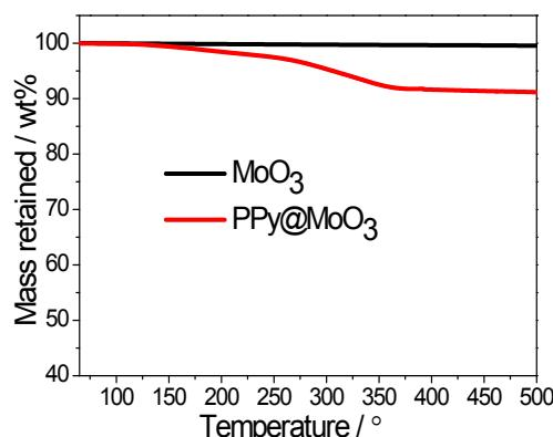
**Fig. S1** Thermogravimetic analysis of the MoO<sub>3</sub> nanotubes under air.
