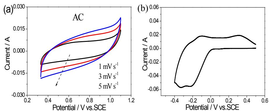
**Fig. S3** CV curves of (a) AC at different scan rate and (b) MoO<sub>3</sub> nanotubes in 0.5 mol l<sup>-1</sup> Al<sub>2</sub>(SO<sub>4</sub>)<sub>3</sub> electrolyte at 5 mV s<sup>-1</sup>.
