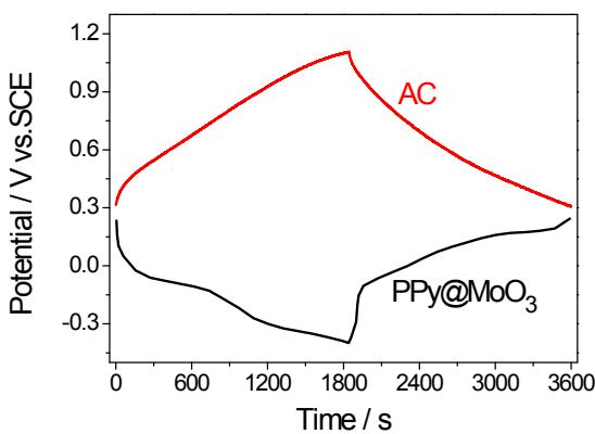
**Fig. S6** Typical charge/discharge curves of the individual electrode (AC and PPy@MoO<sub>3</sub>).
