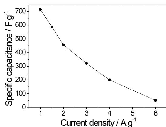
**Fig. S4** Change of capacitance with current densities for MoO<sub>3</sub> nanotubes.
