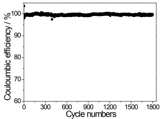
**Fig. S8** The Coulombic efficiency of the Al ion capacitor based on PPy@MoO<sub>3</sub> as the anode at 2 A g<sup>-1</sup>.
