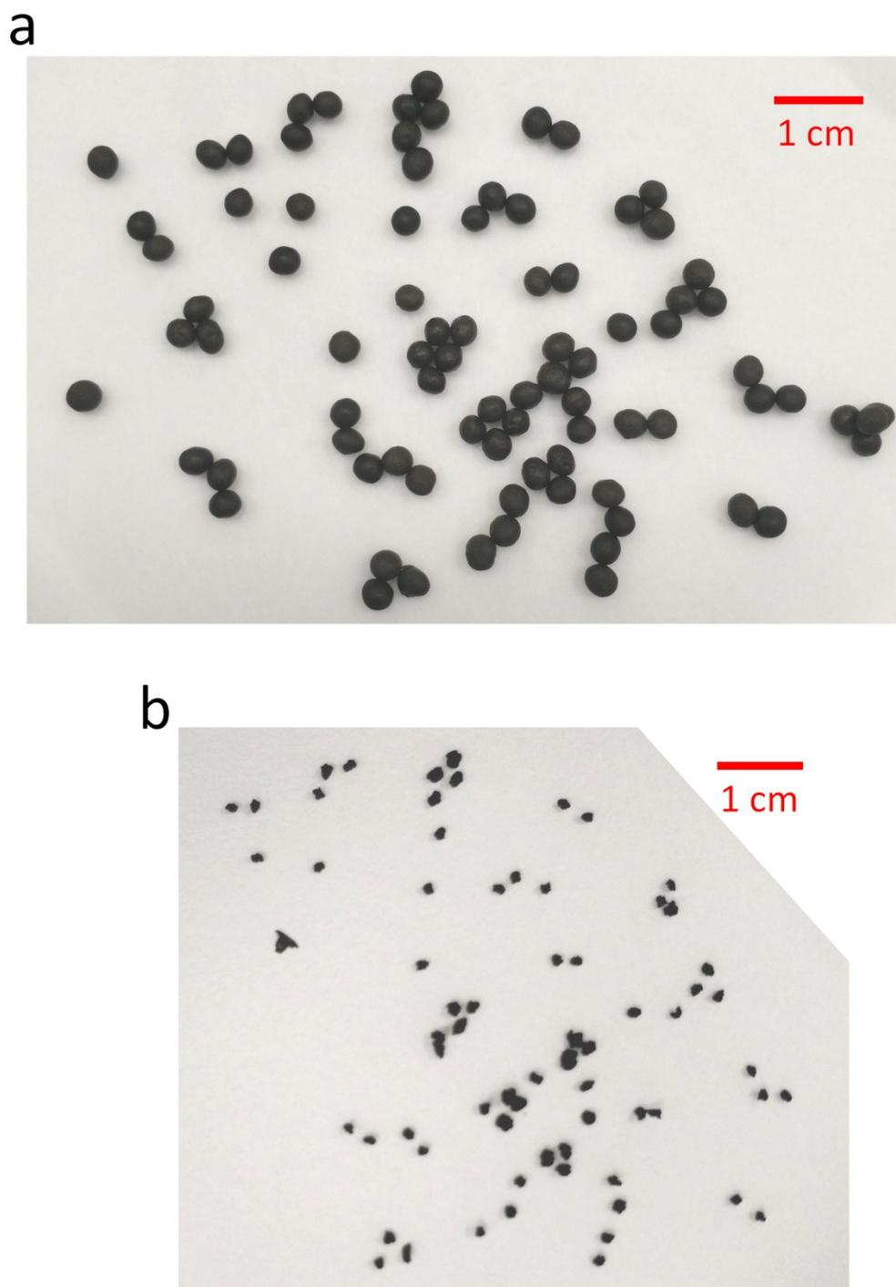
**Fig. S11.** GO beads (a) before and (b) after dried in a blast oven at 80 °C for 30 min. Obvious shrinkage occurred due to the loss of water from the core of beads.
