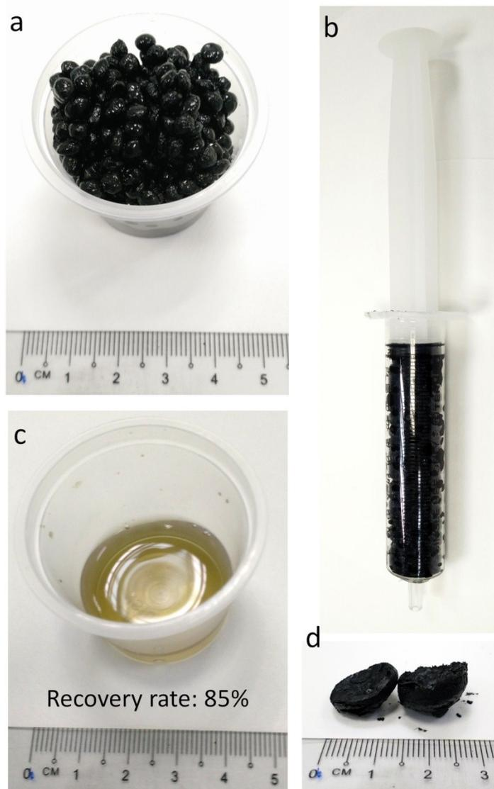
**Fig. S15.** Recovery of sulfuric acid by squeezing GO beads. (a) GO beads after absorbing concentrated sulfuric acid for 10 min. (b) The GO beads were squeezed using a syringe. (c) The collected sulfuric acid. About 85% of the absorbed sulfuric acid was recovered. (d) The GO beads after squeezing, which were compressed tightly and could not recover to spherical beads.
