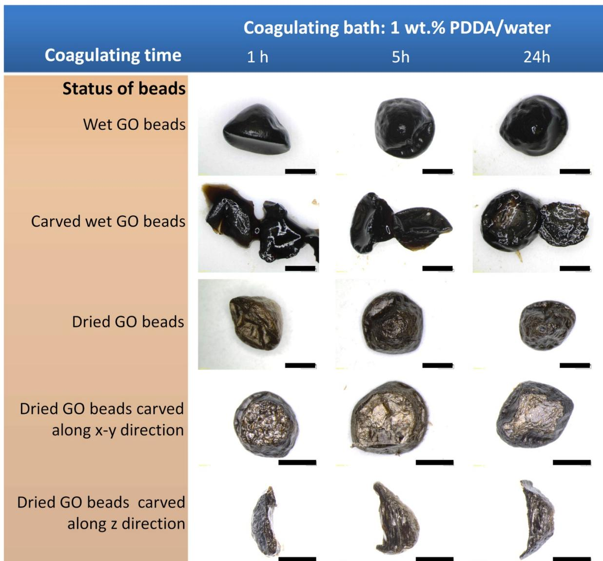
**Fig. S6.** Optical microscope images of the GO beads coagulated using 1 wt.% PDDA/water bath. Scale bars 2 mm.
