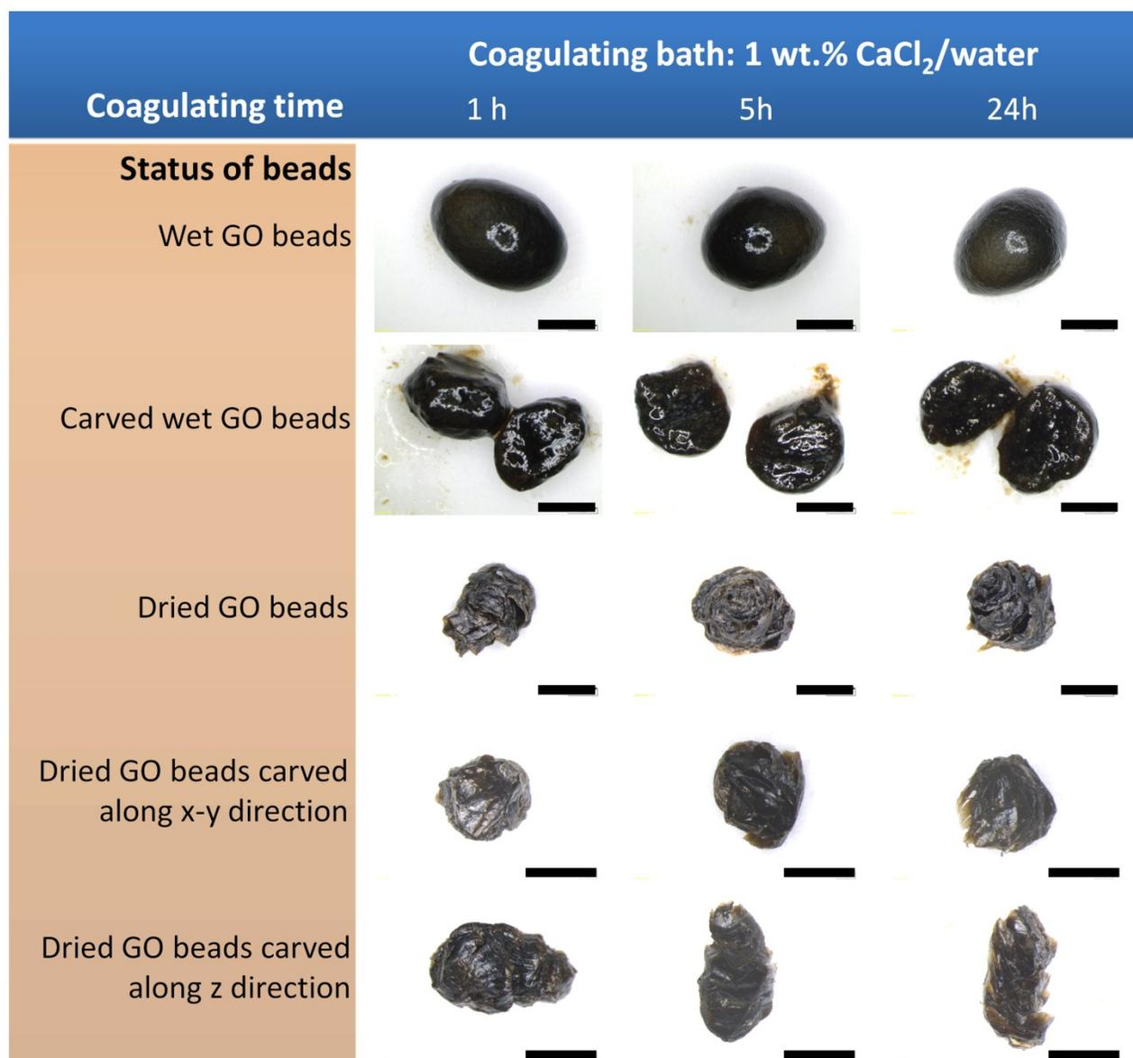
**Fig. S3.** Optical microscope images of the GO beads coagulated using 1 wt.% CaCl<sub>2</sub>/water bath. Scale bars 2 mm.
