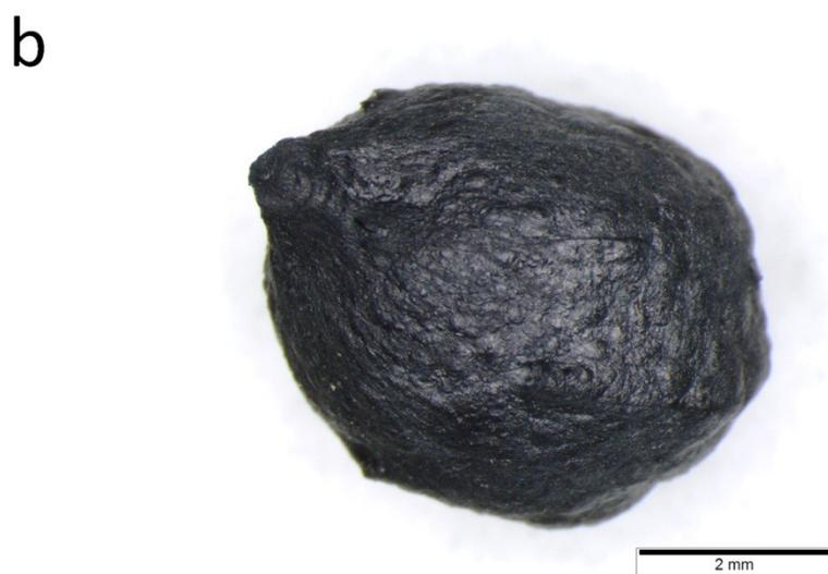
**Fig. S14.** (a) SEM images of MMT. (b) Optical microscope of a MMT/GO bead.
