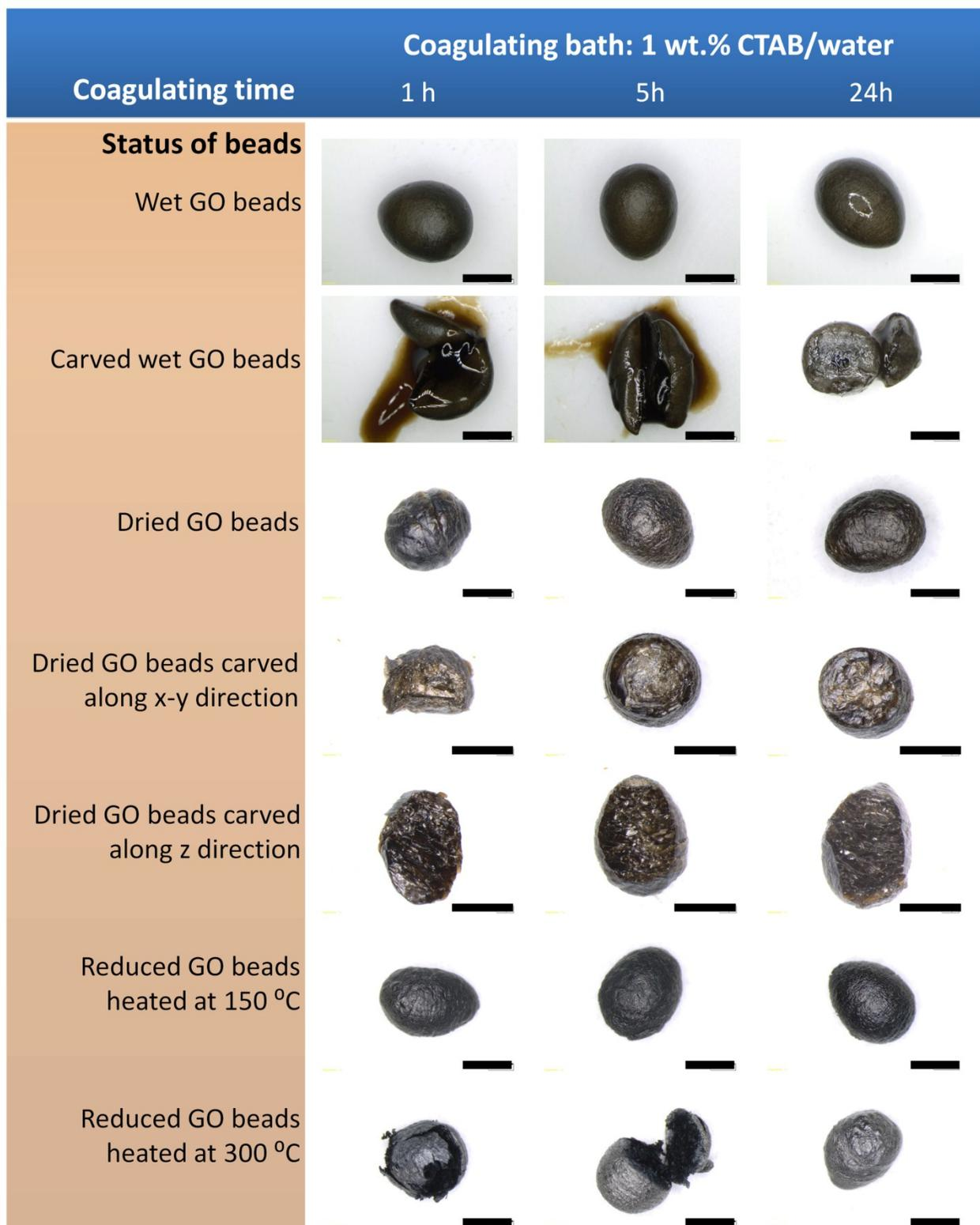
**Fig. S4.** Optical microscope images of the GO beads coagulated using 1 wt.% CTAB/water bath. Scale bars 2 mm.
