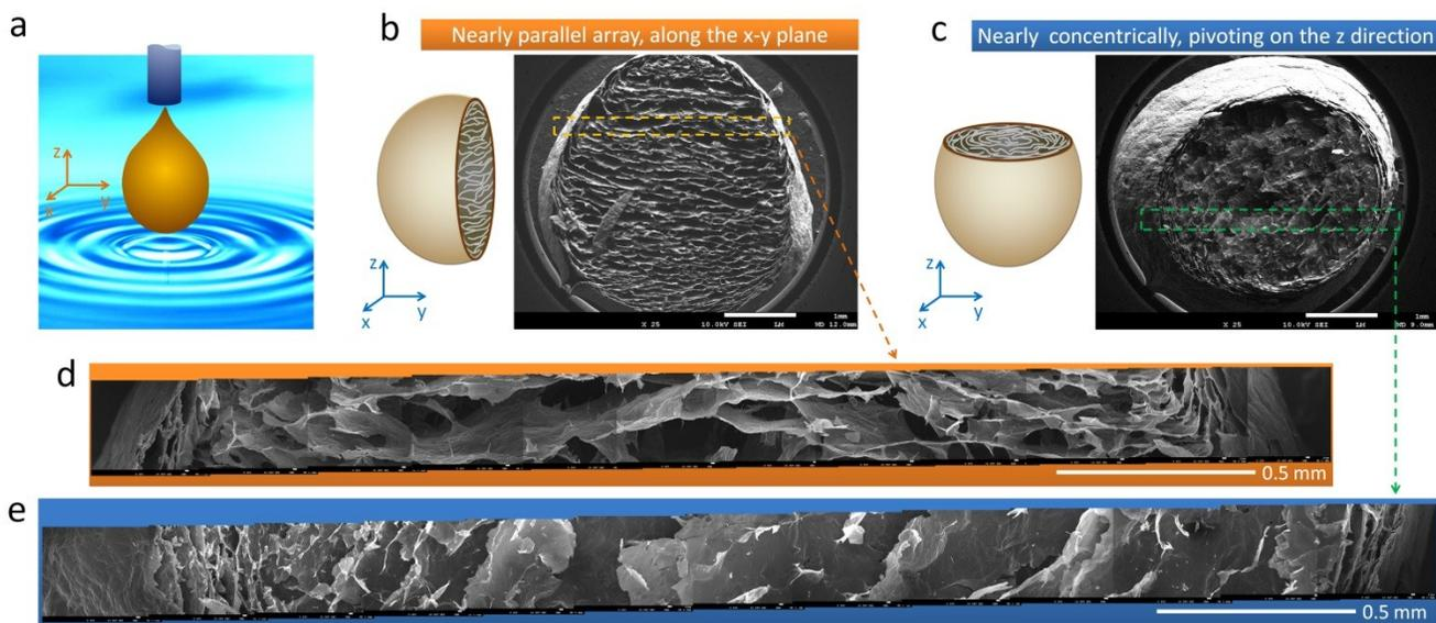
**Fig. S7.** Micro structures of GO beads PEI-24 h-150 °C. (a) Coordinate axis is designed according to the dripping direction of GO/water droplets. (b, c) SEM images of the cross sections of a typical bead. The inner cores present anisotropic porous structures. GO sheets mostly order along the x-y plane. (d, e) Enlarged sections in (b) and (c), respectively. The broad images are spliced from high magnification SEM images (Fig. S8 and S9).
