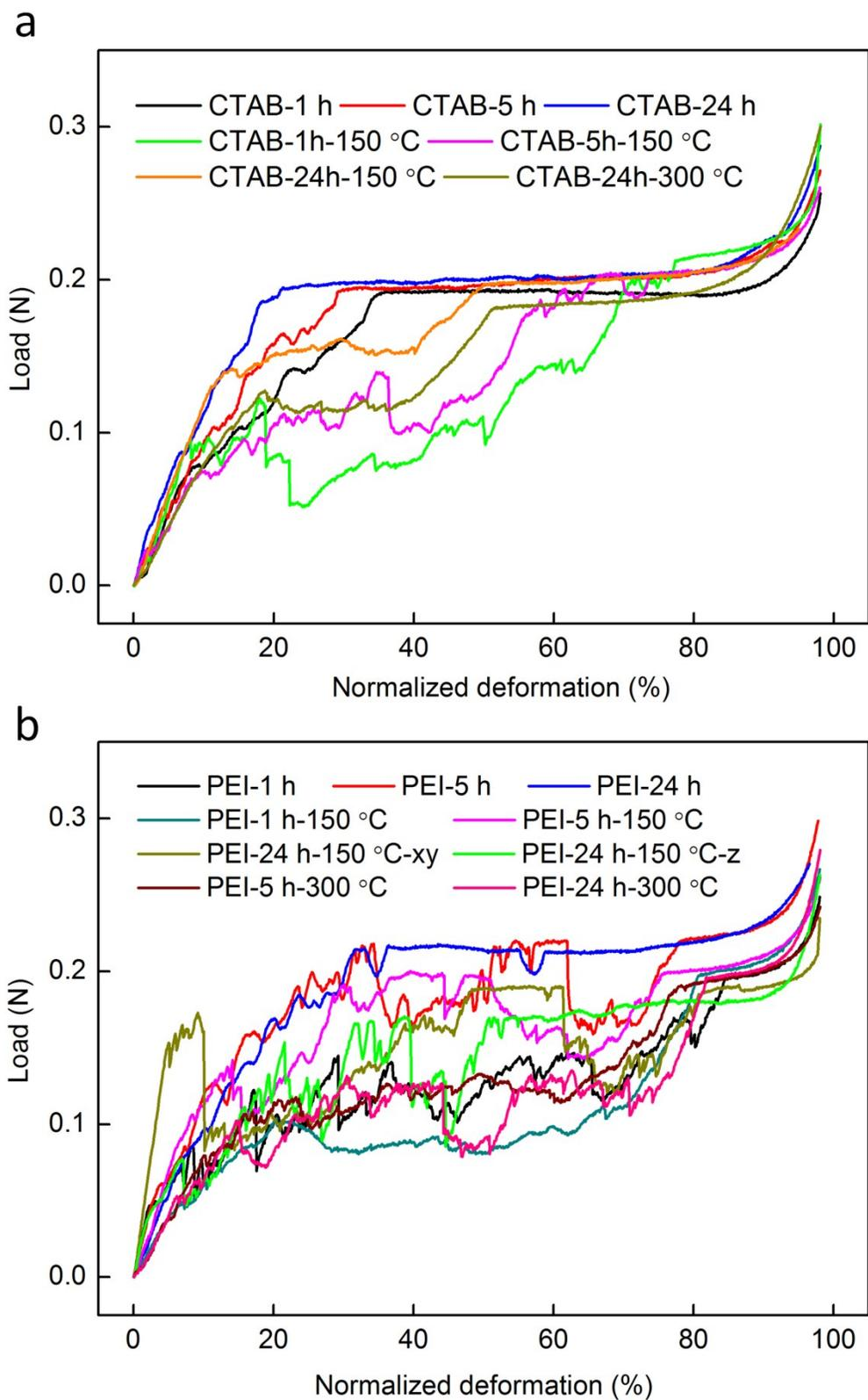
**Fig. S12.** Compression testing results of GO beads. (a) GO beads coagulated using CTAB bath. (b) GO beads coagulated using PEI bath.
