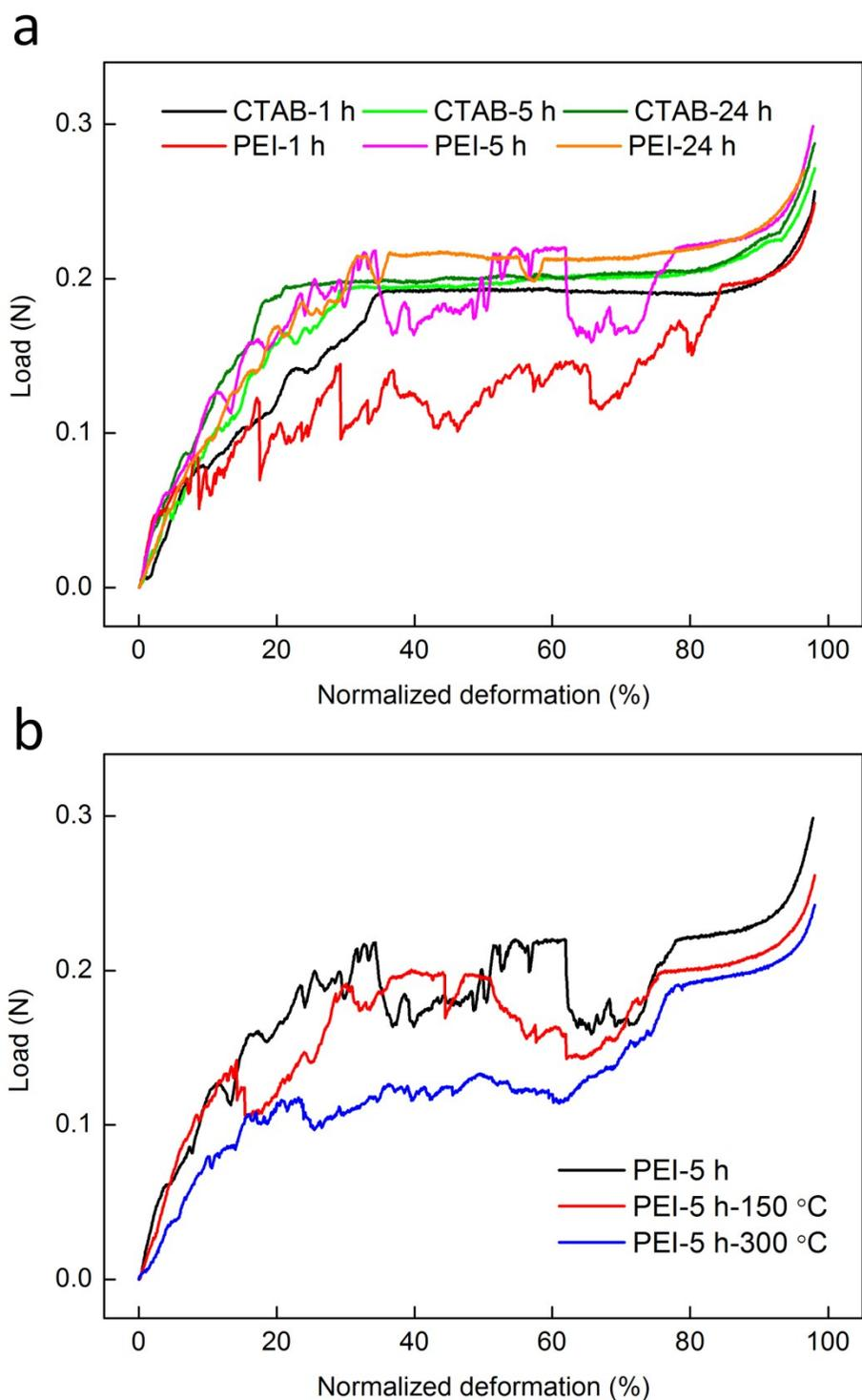
**Fig. S13.** Comparison between the compress properties of GO beads. (a) The GO beads coagulated in 1 wt.% PEI/water bath is more fragile than the GO beads coagulated using 1 wt.% CTAB/water bath, probably due to the reduction of GO caused by the ammine in PEI. (b) Comparison between the GO beads reduced at different temperatures.
