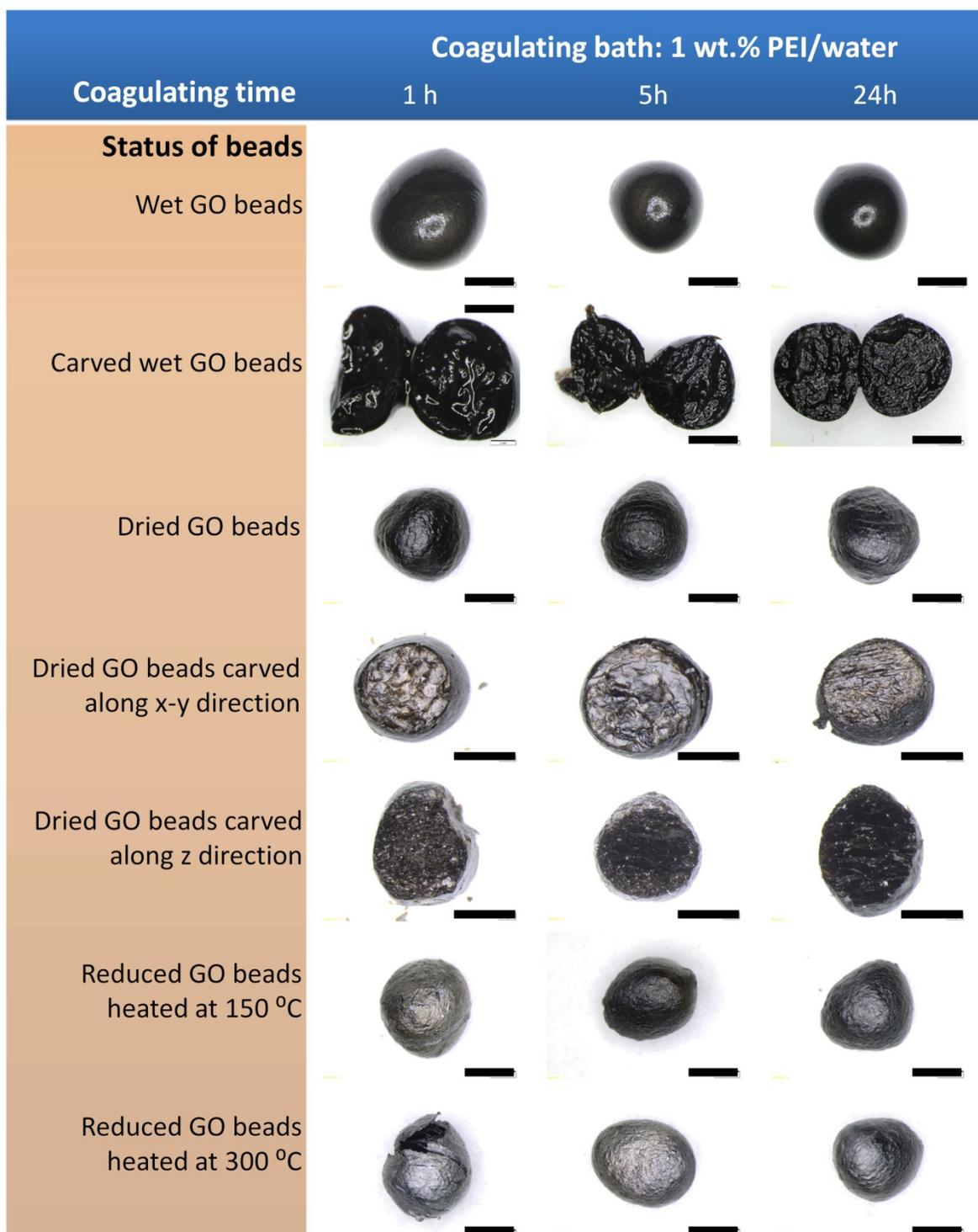
**Fig. S5.** Optical microscope images of the GO beads coagulated using 1 wt.% PEI/water bath. Scale bars 2 mm.
