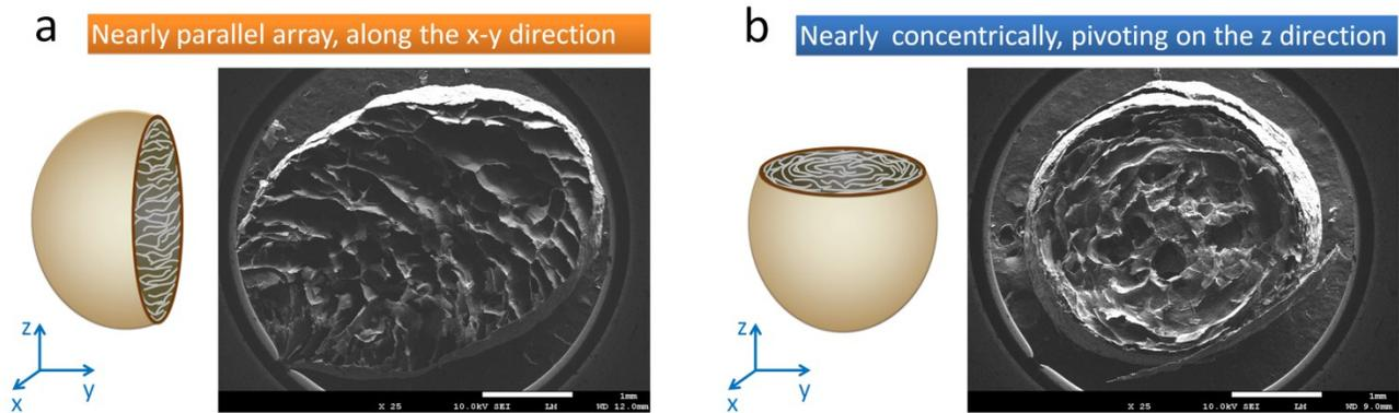
**Fig. S10.** SEM images of GO beads CTAB-5 h-150 °C. (a) The cross section parallel to z direction. (b) The cross section perpendicular to z direction. Scale bars 1mm.
