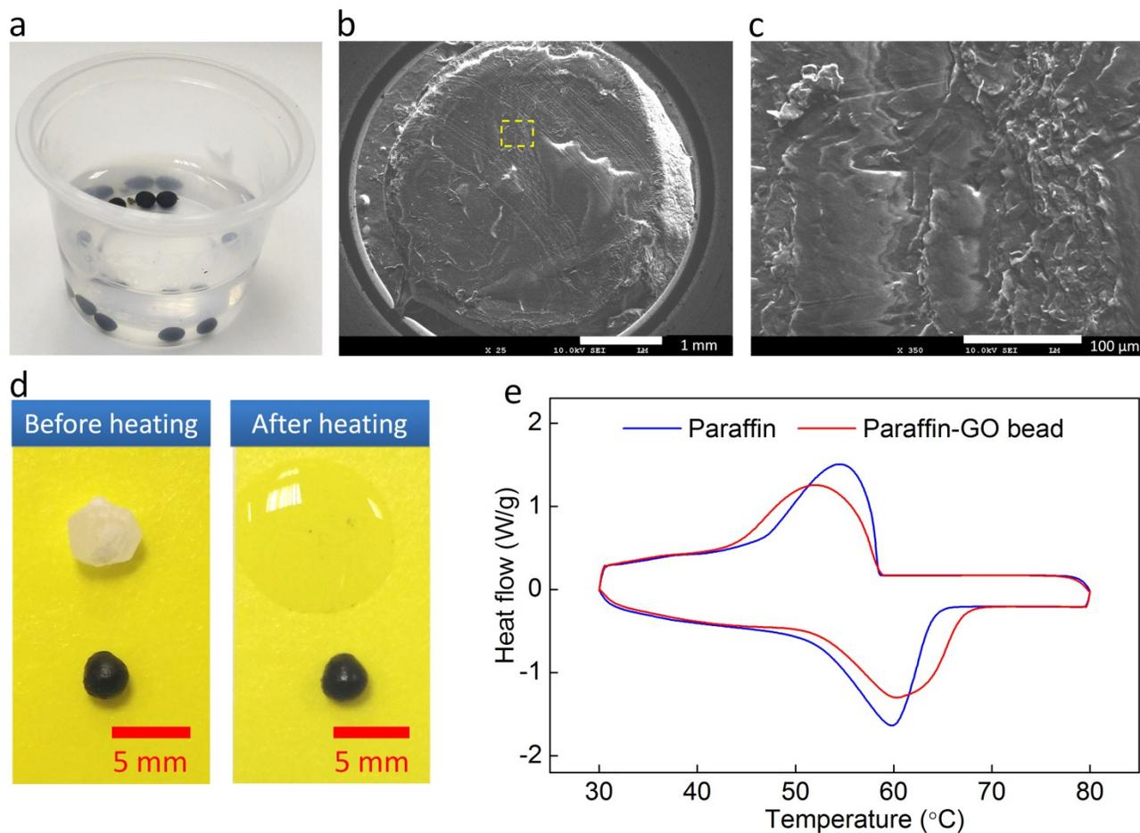
**Fig. S16.** GO beads for thermal energy storage applications. (a) GO beads depositing in melted paraffin. (b) SEM of the cross section of a paraffin-GO bead. (c) Enlarged area in the yellow frame in (b). (d) GO beads endow paraffin stable shape during heating and cooling cycles. (e) DSC curves of neat paraffin and paraffin-GO beads.
