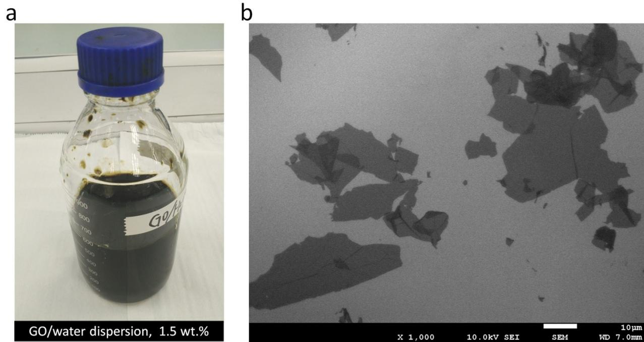
**Fig. S1.** The GO used in this work. (a) Photograph of GO/water dispersion (1.5 wt.%). (b) SEM of GO sheets on silicon substrate.
