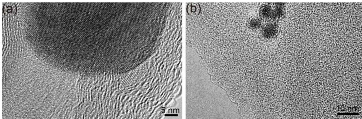
**Fig. S5** HRTEM images of a) CNT and b) GCS in Fe/Fe<sub>3</sub>C@N-C-NaCl.
