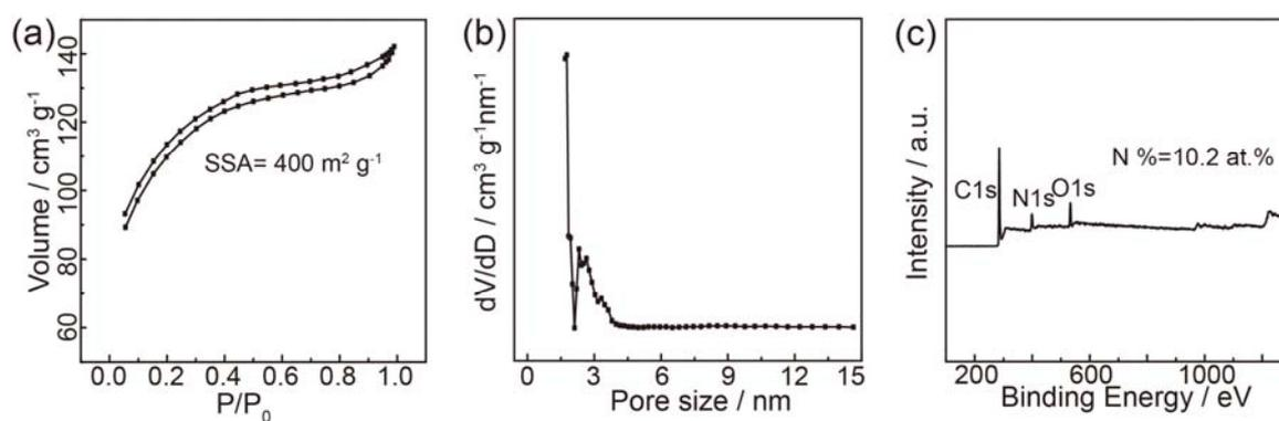
**Fig. S10** a)  $N_2$  adsorption/desorption isotherm, b) the corresponding pore size distribution curve, and c) wide-scan survey XPS spectrum of the sample prepared without iron.
