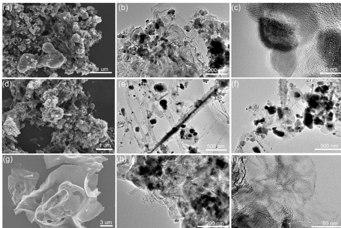
**Fig. S9** a) SEM and b-c) TEM images of the sample synthesized without melamine; d) SEM and e-f) TEM images of the sample synthesized without glucose; g) SEM and h-i) TEM images of the sample synthesized without iron.
