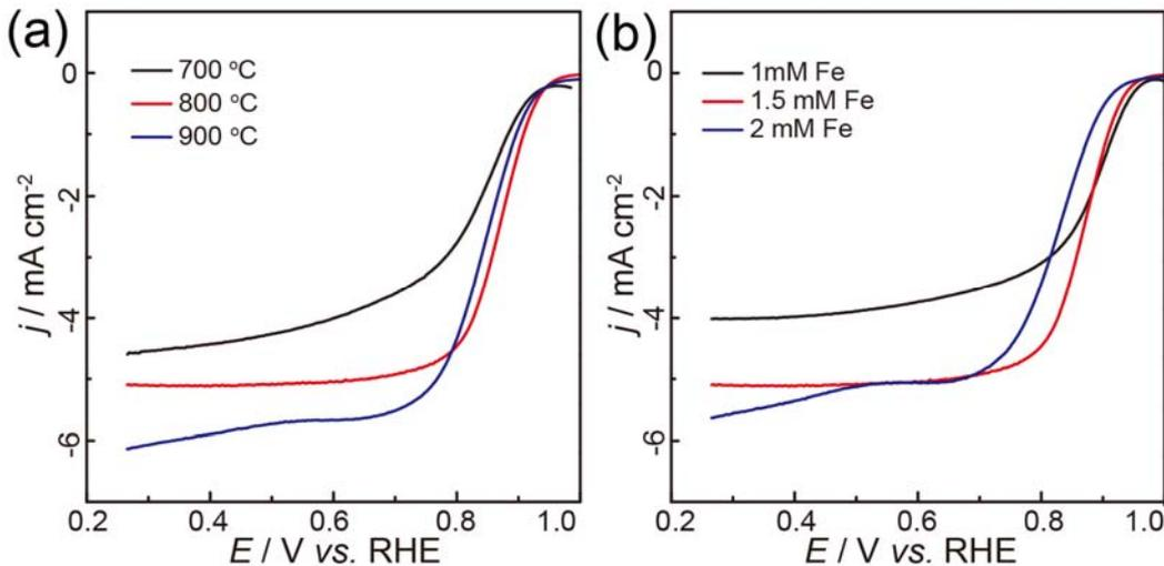
**Fig. S12** a) LSV curves of catalysts prepared at different pyrolysis temperature, and b) LSV curves of catalysts prepared with different iron content. All curves were recorded at a scan rate of  $10 \text{ mV s}^{-1}$  and a rotation speed of 1600 rpm in  $\text{O}_2$ -saturated 0.1 M KOH.
