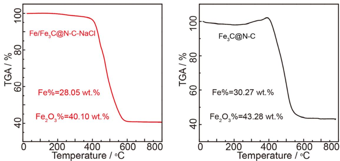
**Fig. S6** TGA profiles of Fe/Fe<sub>3</sub>C@N-C-NaCl and Fe<sub>3</sub>C@N-C measured under atmosphere.
