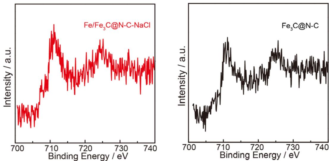
**Fig. S7** High-resolution Fe 2p signals in XPS spectra of Fe/Fe<sub>3</sub>C@N-C-NaCl and Fe<sub>3</sub>C@N-C.
