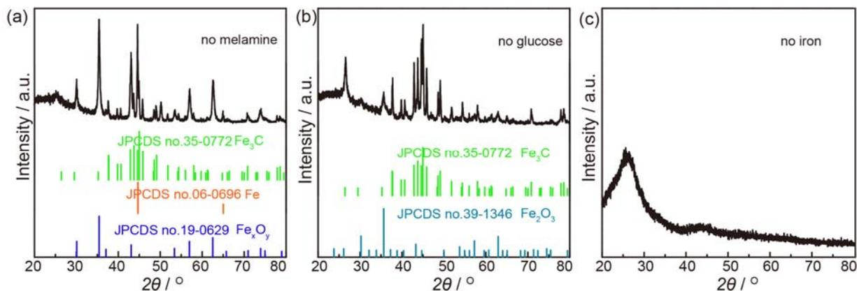
**Fig. S11** a-c) XRD patterns of the samples prepared without melamine, glucose, and iron, respectively.
