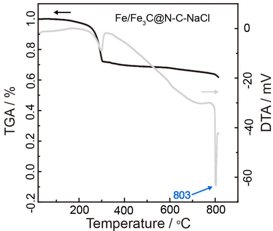
**Fig. S3** TGA-DTA curves measured under Ar flow for monitoring the preparation process of Fe/Fe<sub>3</sub>C@N-C-NaCl.
