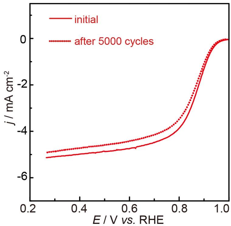
**Fig. S8** LSV curves for Fe/Fe<sub>3</sub>C@N-C-NaCl before and after 5000 potential cycles between 0.6 and 1.0 V (vs RHE) at a scanning rate of 50 mV s<sup>-1</sup>.
