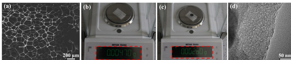
Fig. S1: (a) SEM of PUF. (b) the quality of Al current collector and (c) NCF current collector. (d) TEM of NCF.
