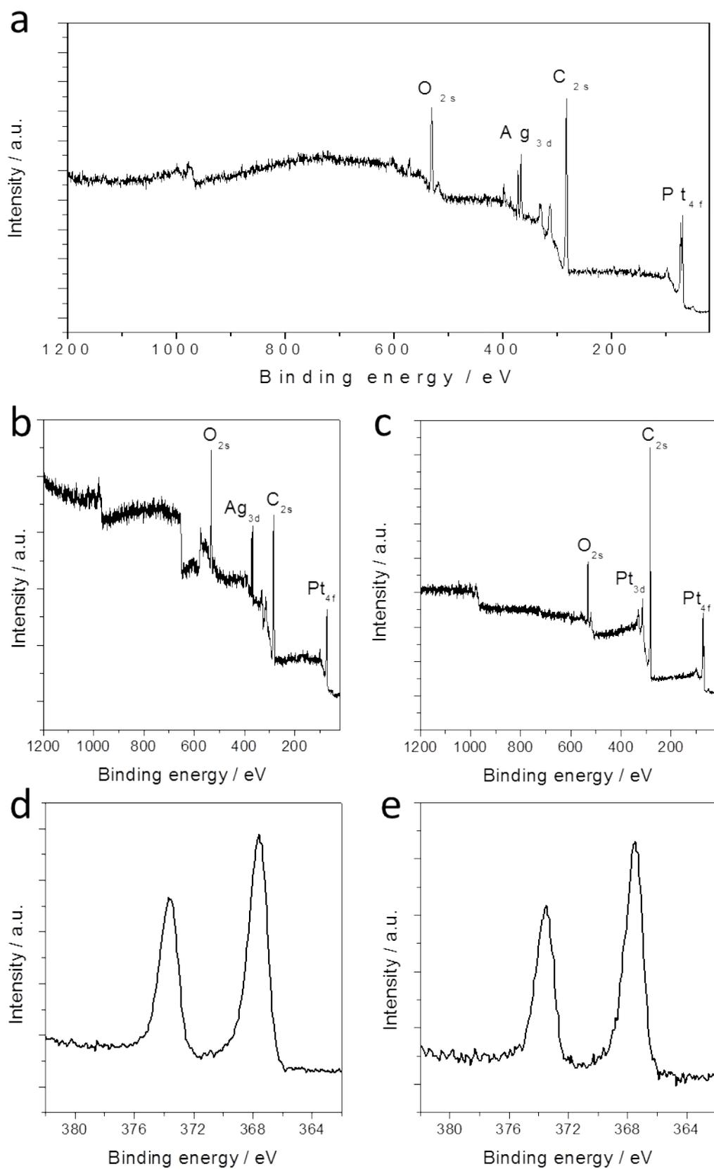
**Figure S4** XPS survey spectrum of HP-Ag/Pt (a), Ag@Pt (b) and Pt/C (c), and high-resolution Ag 3d spectra for Ag@Pt (d) and HP-Ag/Pt (e).
