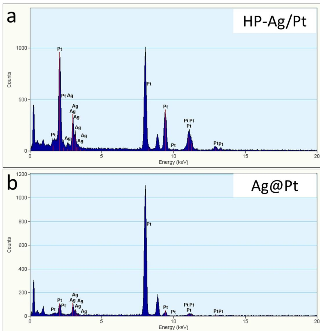
**Figure S3** Typical EDS spectra of the HP-Ag/Pt and Ag@Pt nanoparticles.
