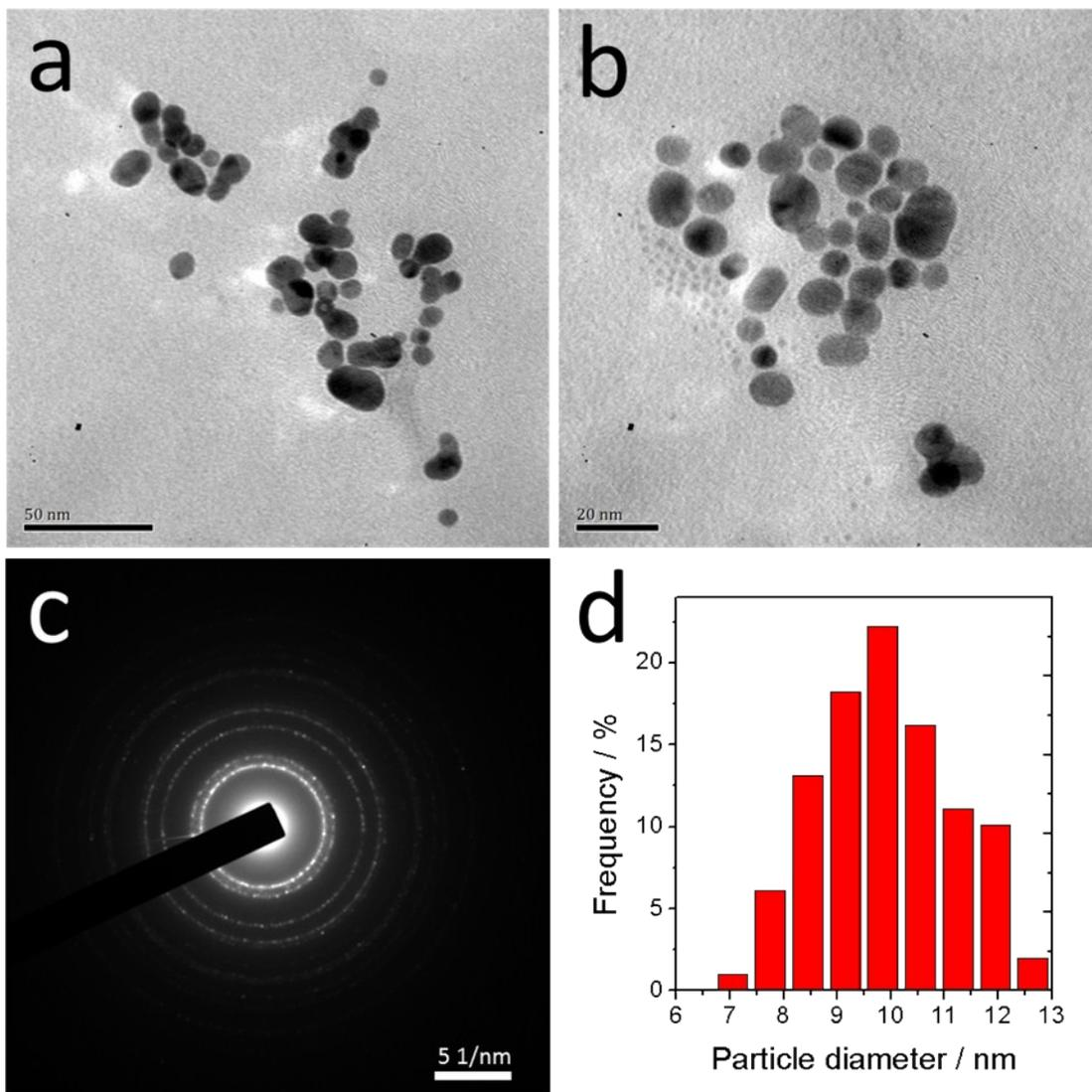
**Figure S2** Typical TEM images (a, b), SAED pattern (c) and size distribution histogram (d) of Ag nanoparticles.
