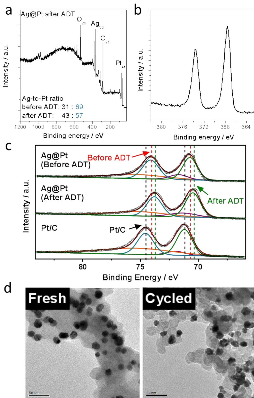
**Figure S7** XPS survey spectrum (a) and high-resolution Ag 3d spectra for Ag@Pt after accelerated durability test. The high-resolution Pt 4f spectra of fresh and after ADT Ag@Pt and Pt/C sample (c) and the TEM images of fresh and cycled Ag@Pt samples (d).
