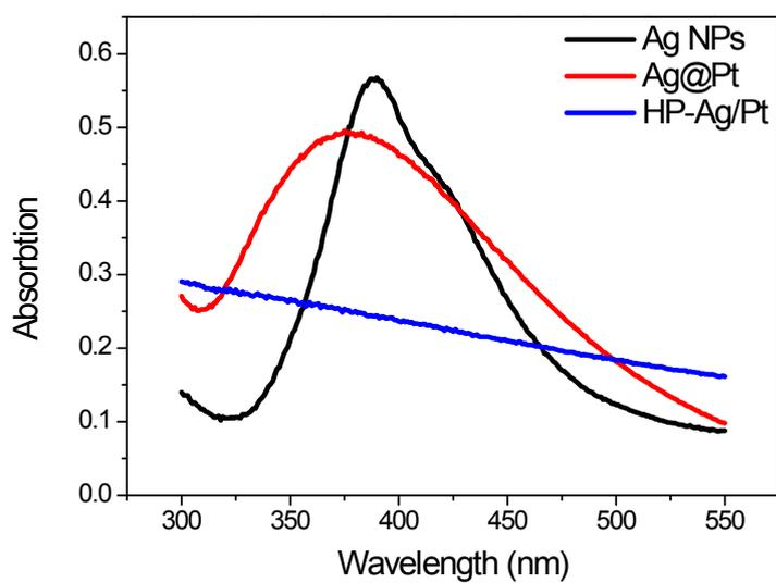
**Figure S1** UV-Vis absorption spectrum of Ag nanoparticles (Ag NPs), Ag@Pt, and HP-Ag/Pt.
