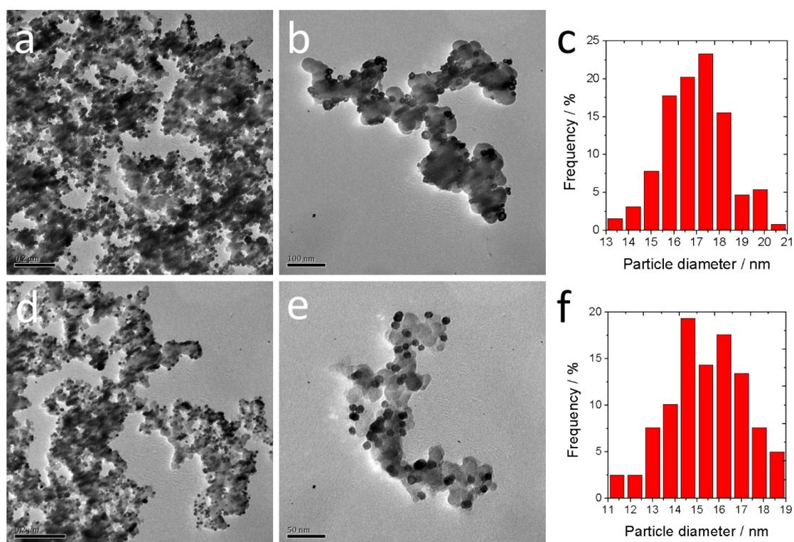
**Figure S5** Typical TEM images and size distribution histogram of the HP-Ag/Pt on VC-72R (a, b, c) and Ag@Pt on VC-72R (d, e, f).
