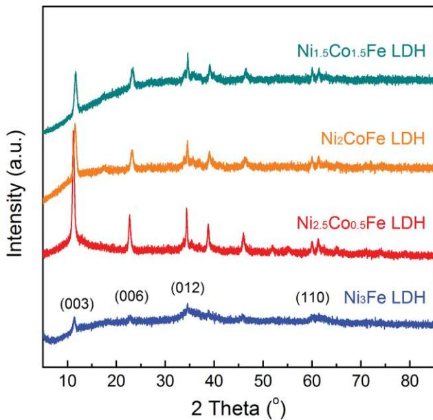
**Fig. S2** XRD patterns of NiCoFe LDH samples with different compositions prepared by hydrothermal method.
