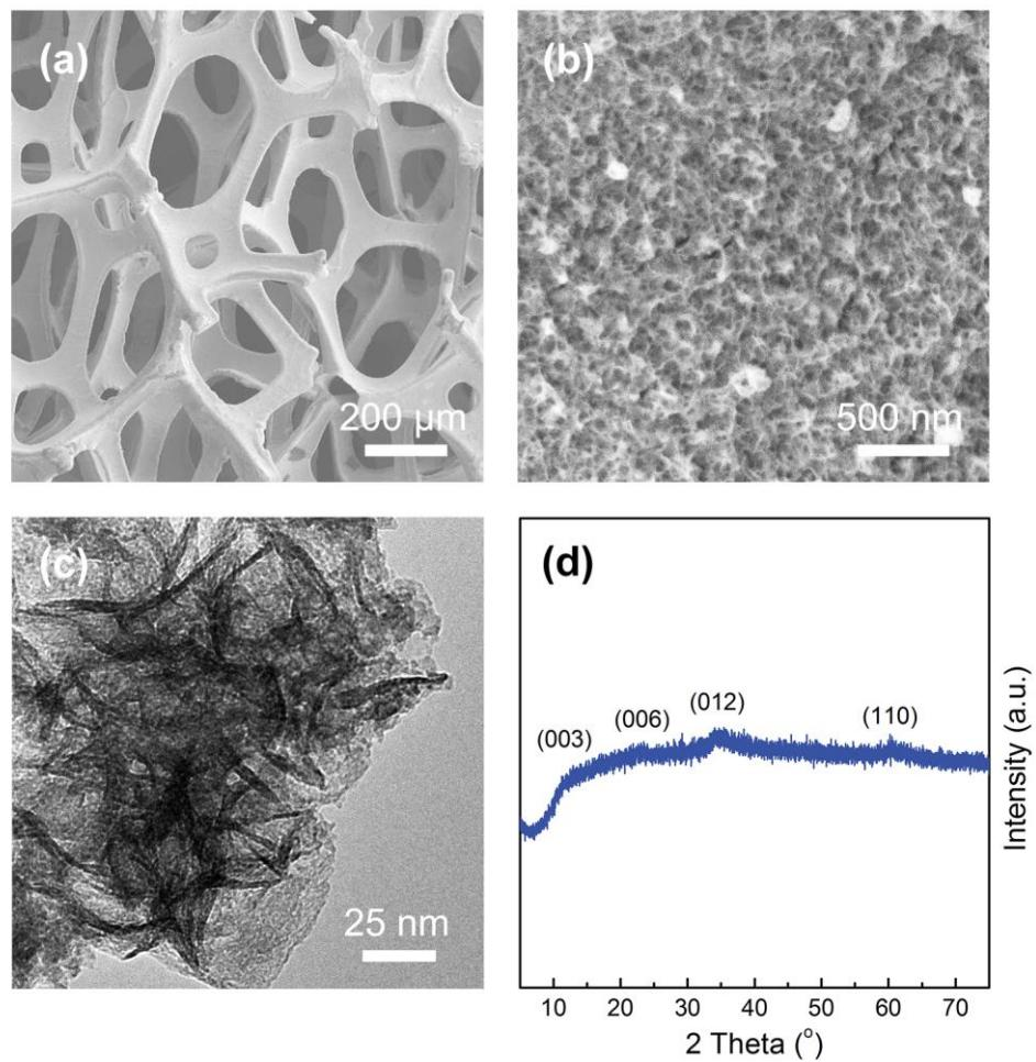
**Fig. S1** Morphology and structure characterizations of NiFe/NF electrode. (a,b) SEM images of the NiFe/NF electrode. (c) TEM image of the electrodeposited NiFe LDHs. (d) XRD pattern of NiFe LDHs.
