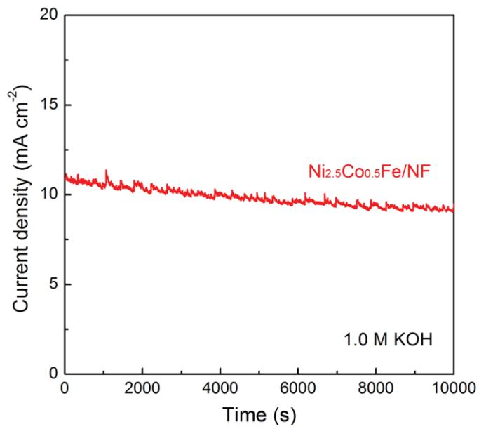
**Fig. S4** Stability of  $\text{Ni}_{2.5}\text{Co}_{0.5}\text{Fe}/\text{NF}$  electrodes for overall water splitting at an initial current density around  $10 \text{ mA cm}^{-2}$ .
