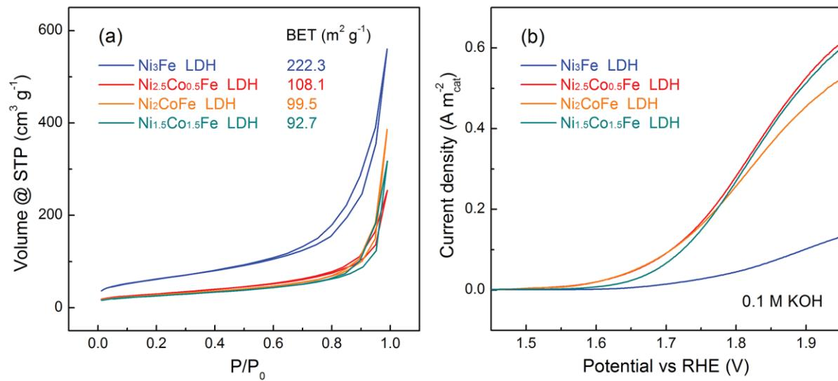
**Fig. S3** (a)  $\text{N}_2$  adsorption-desorption isotherms and BET specific surface areas of NiCoFe LDHs with different compositions. (b) OER activity respect to catalyst surface area in 0.10 M KOH electrolyte.
