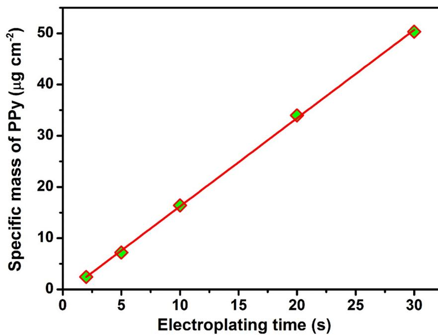
**Figure S5.** The plated mass of PPy films versus the electroplating time.
