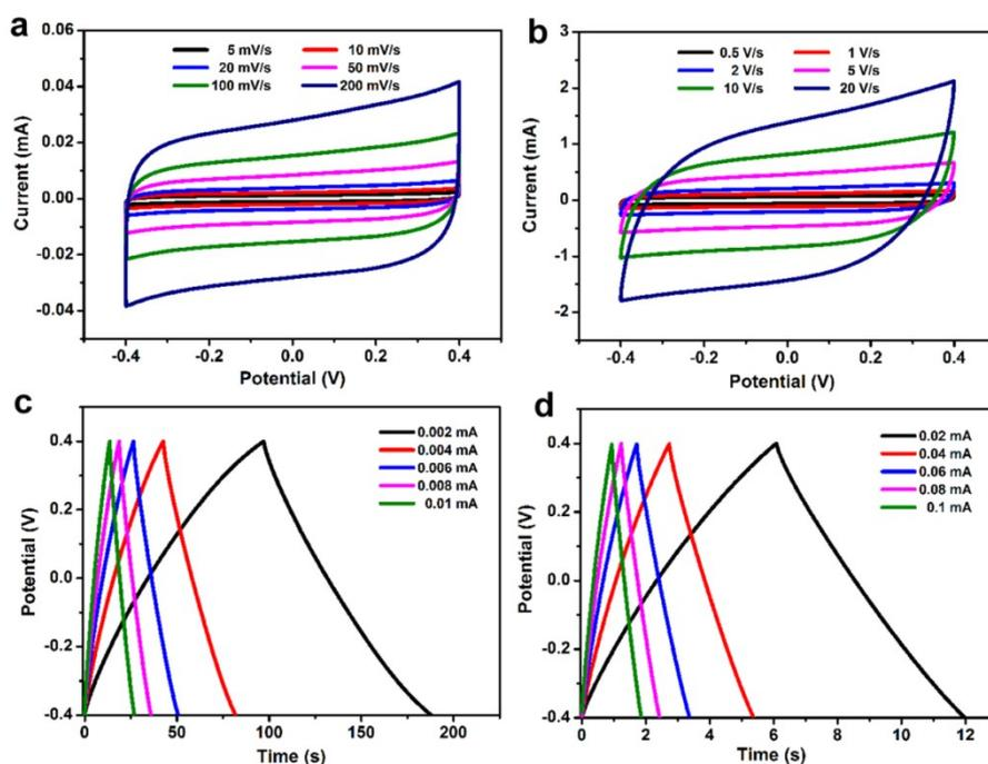
**Figure S9.** CV curves of NPG/MnO<sub>2</sub> MSC with the MnO<sub>2</sub> plating time of 5 min at scan rates ranging from (a) 5 to 200 mV s<sup>-1</sup>; (b) 0.5 to 20 V s<sup>-1</sup>. Galvanostatic charge/discharge curves of NPG/MnO<sub>2</sub> MSC with the MnO<sub>2</sub> plating time of 5 min at different current from (c) 0.002 to 0.01 mA; (d) 0.02 to 0.1 mA.
