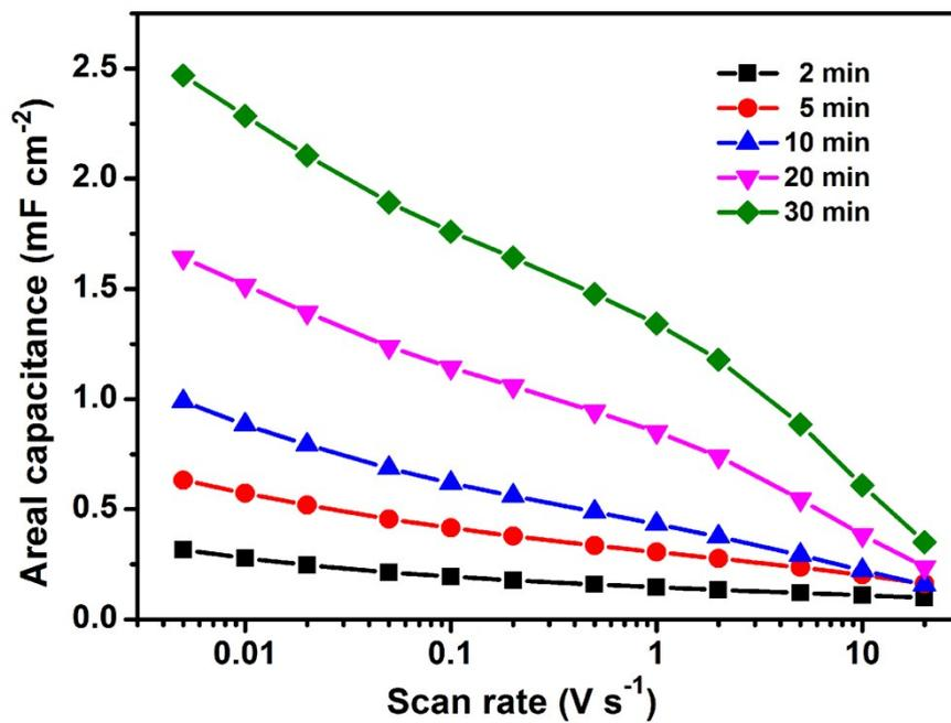
**Figure S13.** Evolution of the areal capacitance of MSC with various mass loadings of MnO<sub>2</sub> as a function of scan rate.
