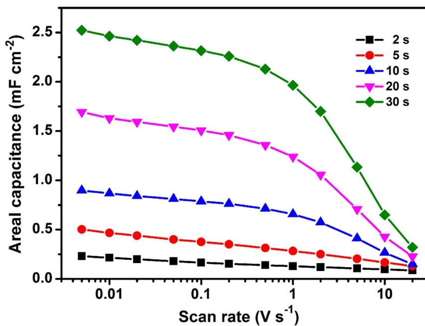
**Figure S15.** Evolution of the areal capacitance of MSC with various mass loadings of PPy as a function of scan rate.
