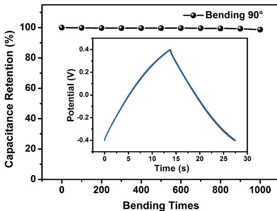
**Figure S22.** Capacitance retention of the flexible device after 1000 bending cycles with a bending angle of 90°. The inset is the galvanostatic charge/discharge curves of NPG/MnO<sub>2</sub> MSC after bending.
