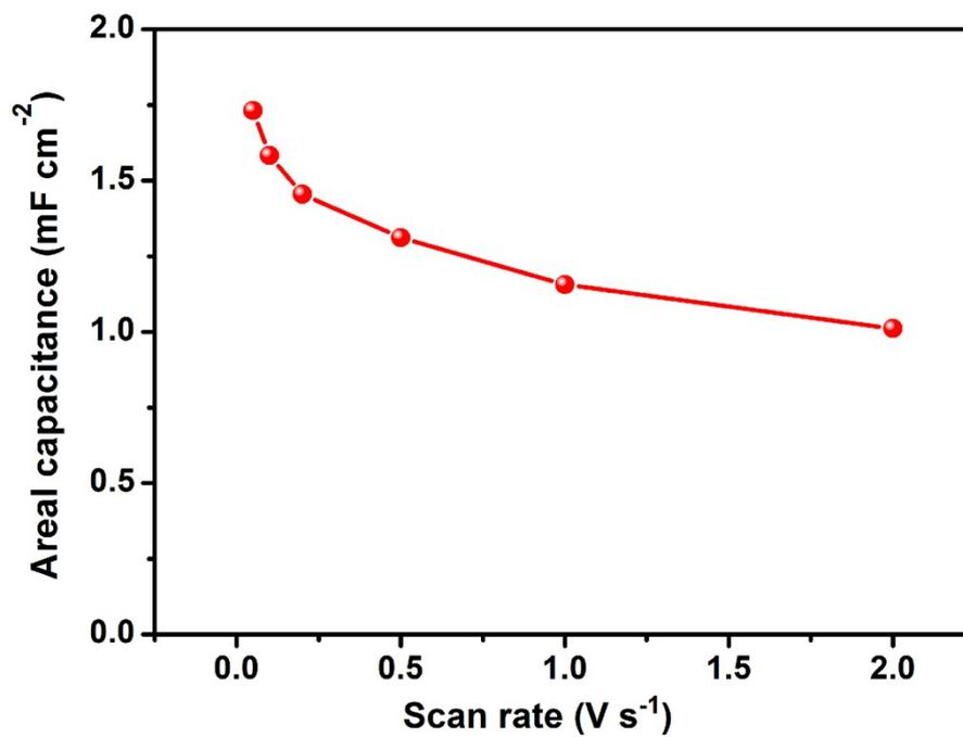
**Figure S23.** Areal capacitance of AMSC based 10 min MnO<sub>2</sub> plating and 10 s PPy plating as a function of scan rate.
