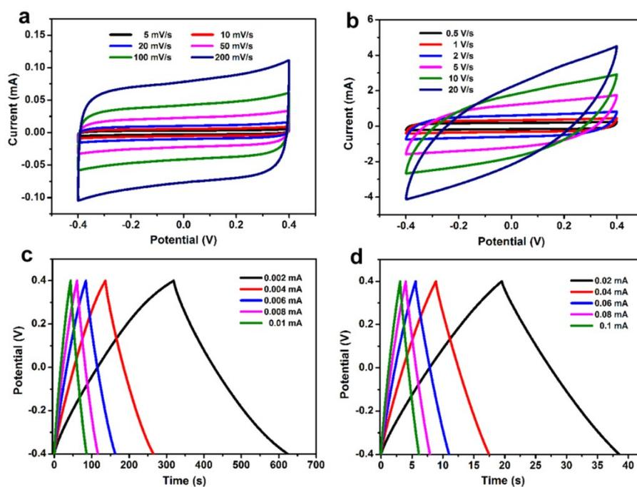
**Figure S11.** CV curves of NPG/MnO<sub>2</sub> MSC with the MnO<sub>2</sub> plating time of 20 min at scan rates ranging from (a) 5 to 200 mV s<sup>-1</sup>; (b) 0.5 to 20 V s<sup>-1</sup>. Galvanostatic charge/discharge curves of NPG/MnO<sub>2</sub> MSC with the MnO<sub>2</sub> plating time of 20 min at different current from (c) 0.002 to 0.01 mA; (d) 0.02 to 0.1 mA.
