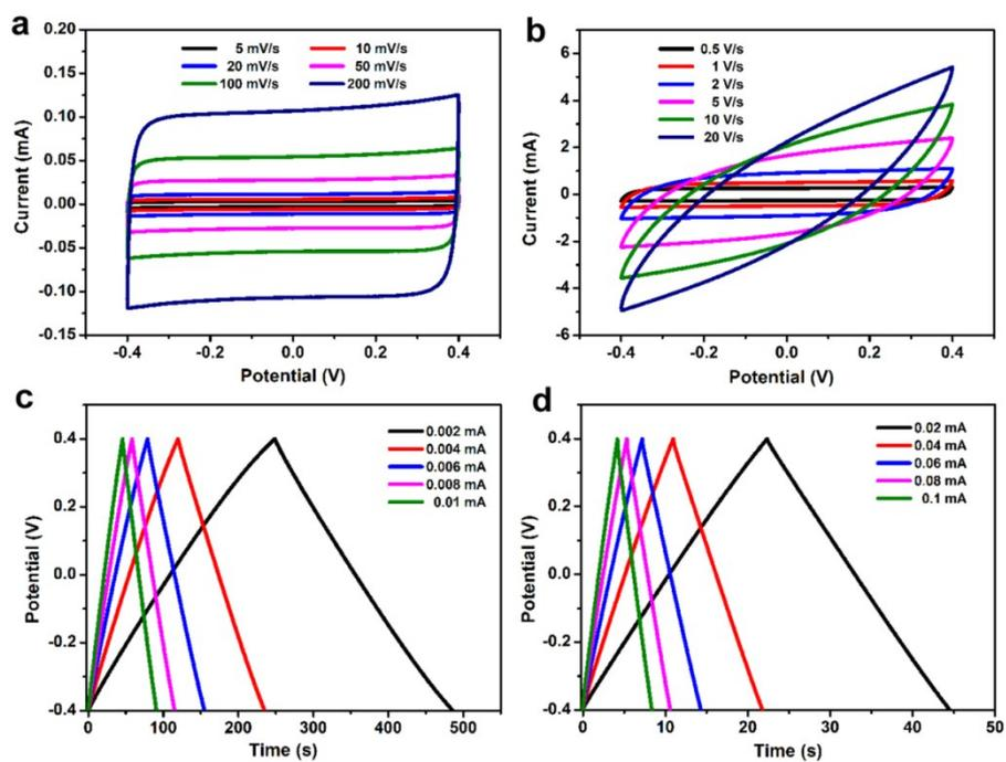
**Figure S19.** CV curves of NPG/PPy MSC with the PPy plating time of 20 s at scan rates ranging from (a) 5 to 200  $\text{mV s}^{-1}$ ; (b) 0.5 to 20  $\text{V s}^{-1}$ . Galvanostatic charge/discharge curves of NPG/PPy MSC with the PPy plating time of 20 s at different current from (c) 0.002 to 0.01 mA; (d) 0.02 to 0.1 mA.
