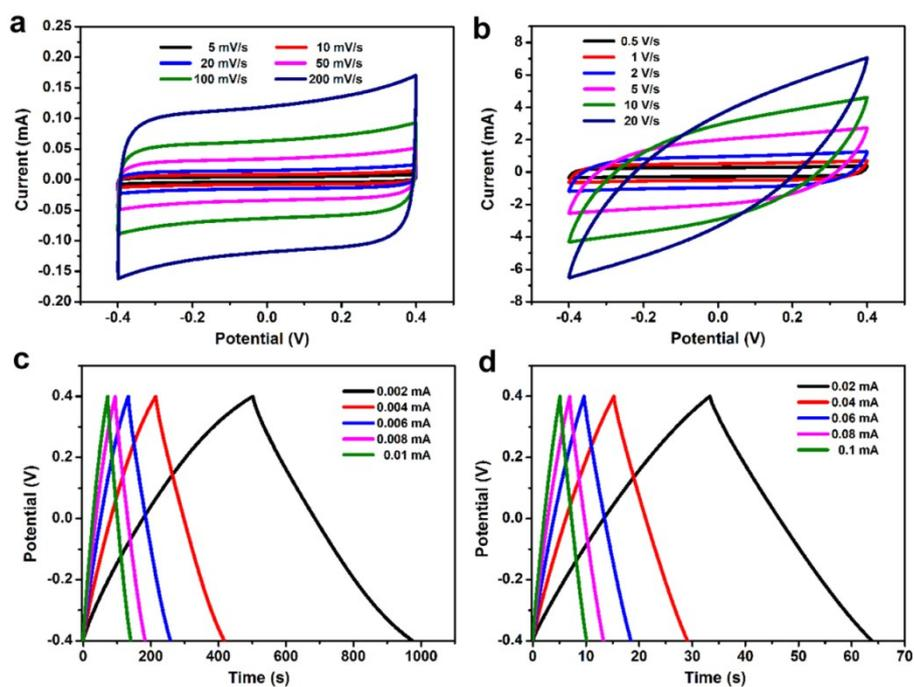
**Figure S12.** CV curves of NPG/MnO<sub>2</sub> MSC with the MnO<sub>2</sub> plating time of 30 min at scan rates ranging from (a) 5 to 200 mV s<sup>-1</sup>; (b) 0.5 to 20 V s<sup>-1</sup>. Galvanostatic charge/discharge curves of NPG/MnO<sub>2</sub> MSC with the MnO<sub>2</sub> plating time of 30 min at different current from (c) 0.002 to 0.01 mA; (d) 0.02 to 0.1 mA.
