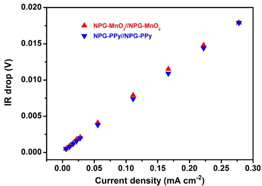
**Figure S21.** IR drop of NPG based MSC with the MnO<sub>2</sub> plating time of 10 min or the PPy plating time of 10 s at various current densities.
