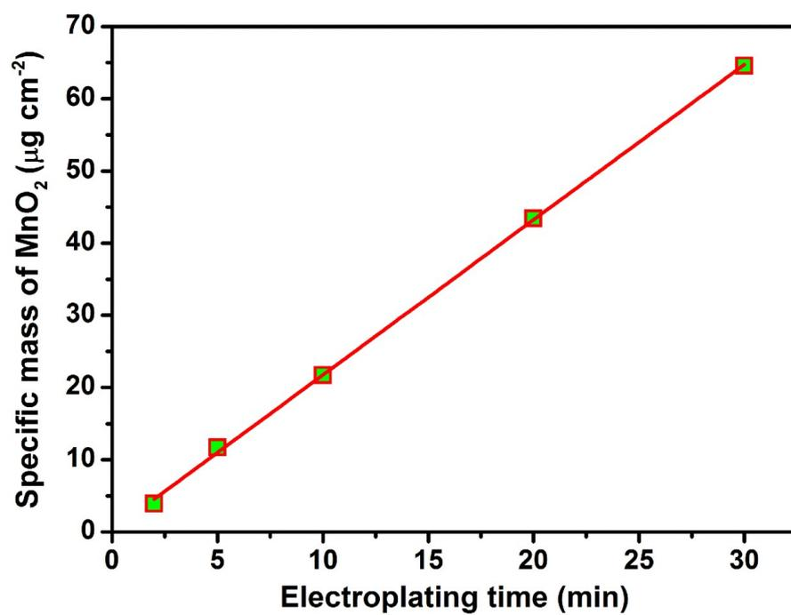
**Figure S2.** The plated mass of MnO<sub>2</sub> films versus the electroplating time.
