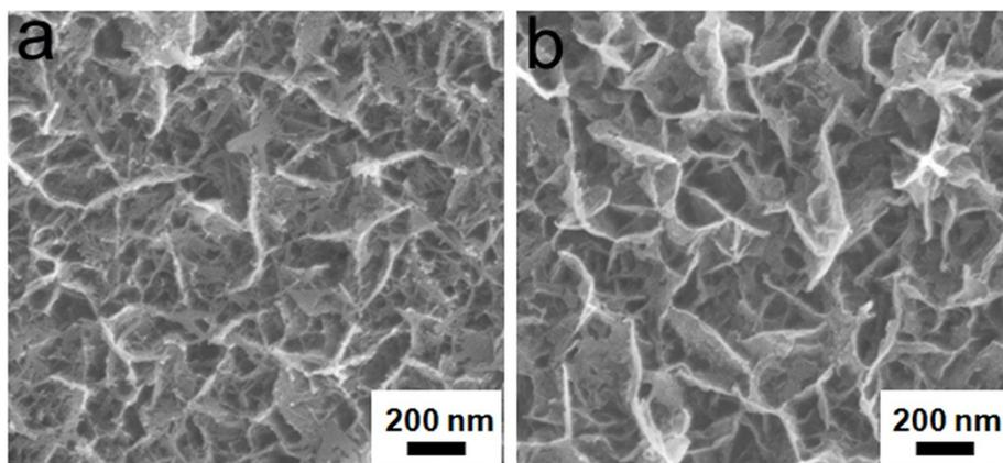
**Figure S1.** SEM images of NPG/MnO<sub>2</sub> composites with the MnO<sub>2</sub> plating time of (a) 20 min, (b) 30 min.
