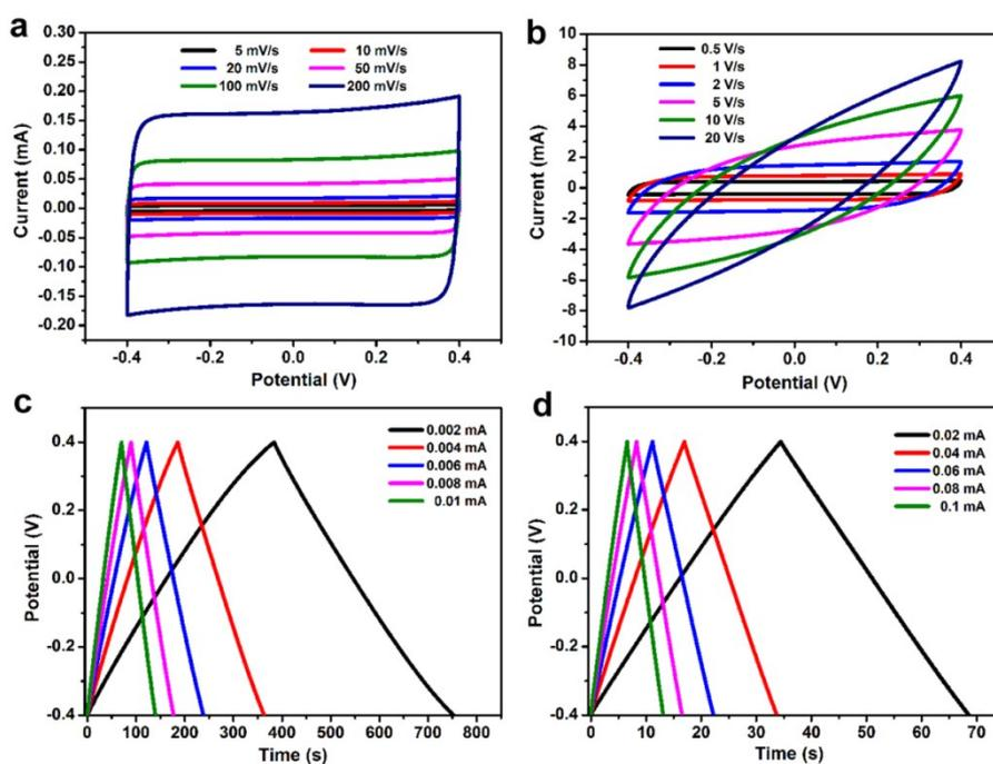
**Figure S20.** CV curves of NPG/PPy MSC with the PPy plating time of 30 s at scan rates ranging from (a) 5 to 200  $\text{mV s}^{-1}$ ; (b) 0.5 to 20  $\text{V s}^{-1}$ . Galvanostatic charge/discharge curves of NPG/PPy MSC with the PPy plating time of 30 s at different current from (c) 0.002 to 0.01 mA; (d) 0.02 to 0.1 mA.
