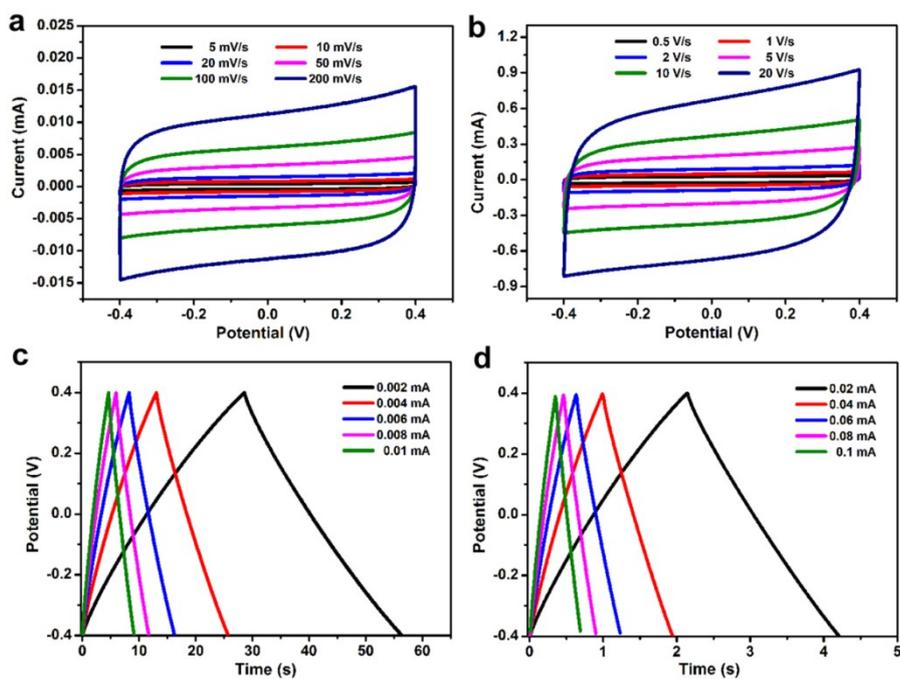
**Figure S16.** CV curves of NPG/PPy MSC with the PPy plating time of 2 s at scan rates ranging from (a) 5 to 200  $\text{mV s}^{-1}$ ; (b) 0.5 to 20  $\text{V s}^{-1}$ . Galvanostatic charge/discharge curves of NPG/PPy MSC with the PPy plating time of 2 s at different current from (c) 0.002 to 0.01 mA; (d) 0.02 to 0.1 mA.
