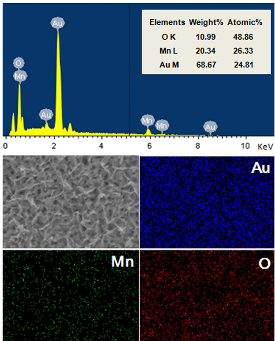
**Figure S3.** EDX spectrum and elemental mapping images of the NPG/MnO<sub>2</sub> composite.
