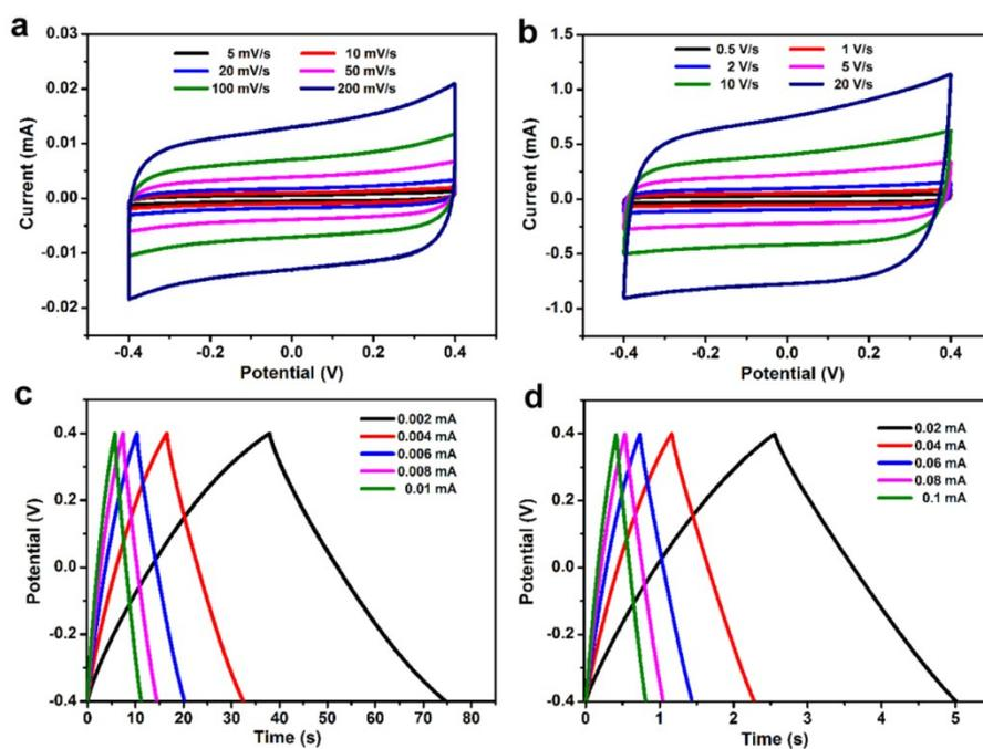
**Figure S8.** CV curves of NPG/MnO<sub>2</sub> MSC with the MnO<sub>2</sub> plating time of 2 min at scan rates ranging from (a) 5 to 200 mV s<sup>-1</sup>; (b) 0.5 to 20 V s<sup>-1</sup>. Galvanostatic charge/discharge curves of NPG/MnO<sub>2</sub> MSC with the MnO<sub>2</sub> plating time of 2 min at different current from (c) 0.002 to 0.01 mA; (d) 0.02 to 0.1 mA.
