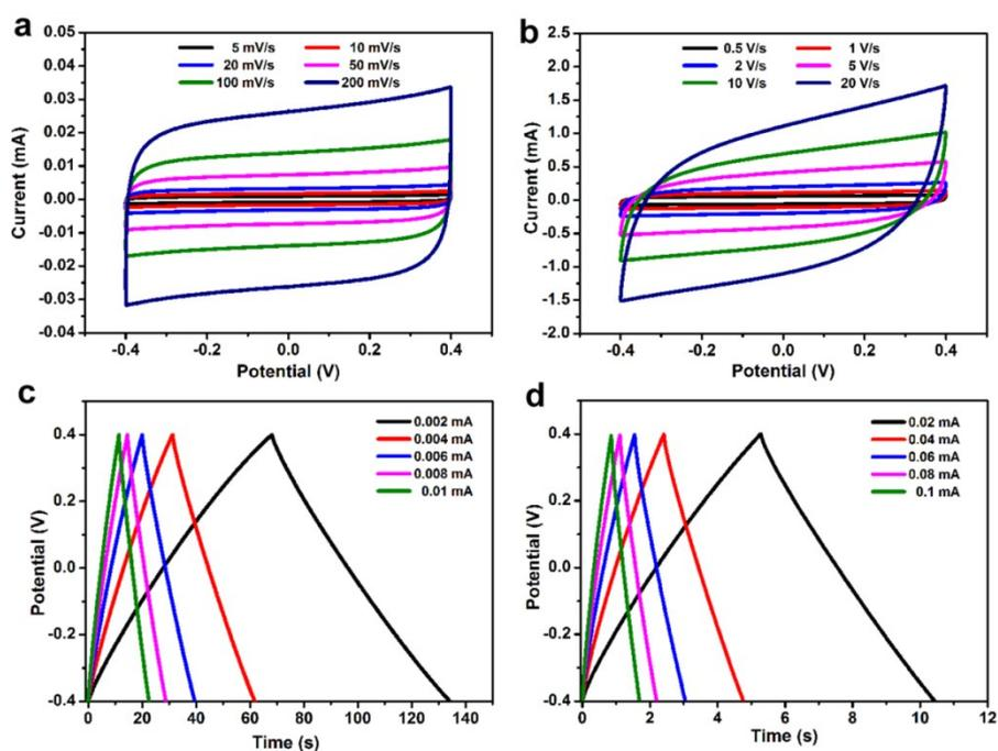
**Figure S17.** CV curves of NPG/PPy MSC with the PPy plating time of 5 s at scan rates ranging from (a) 5 to 200  $\text{mV s}^{-1}$ ; (b) 0.5 to 20  $\text{V s}^{-1}$ . Galvanostatic charge/discharge curves of NPG/PPy MSC with the PPy plating time of 5 s at different current from (c) 0.002 to 0.01 mA; (d) 0.02 to 0.1 mA.
