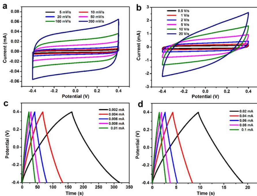
**Figure S10.** CV curves of NPG/MnO<sub>2</sub> MSC with the MnO<sub>2</sub> plating time of 10 min at scan rates ranging from (a) 5 to 200 mV s<sup>-1</sup>; (b) 0.5 to 20 V s<sup>-1</sup>. Galvanostatic charge/discharge curves of NPG/MnO<sub>2</sub> MSC with the MnO<sub>2</sub> plating time of 10 min at different current from (c) 0.002 to 0.01 mA; (d) 0.02 to 0.1 mA.
