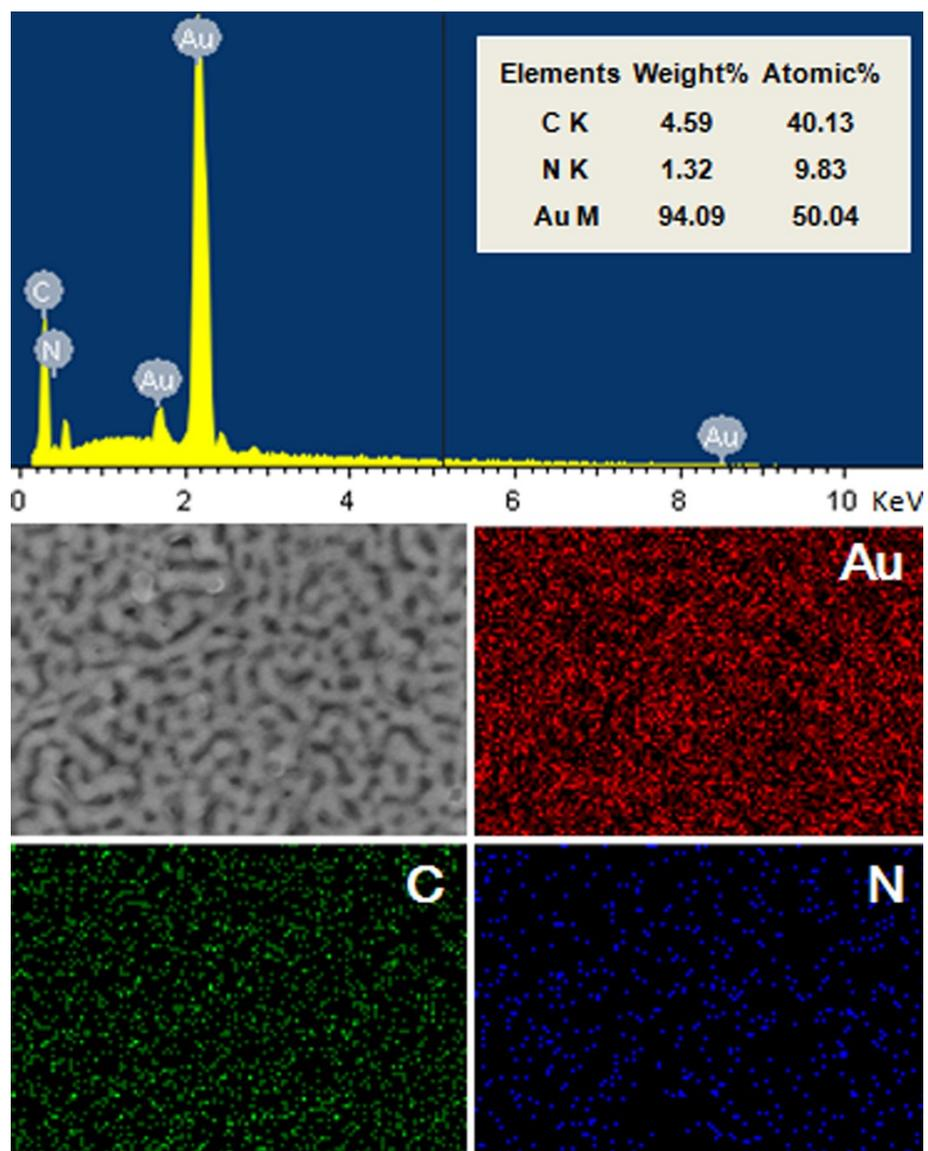
**Figure S6.** EDX spectrum and elemental mapping images of the NPG/PPy composite.
