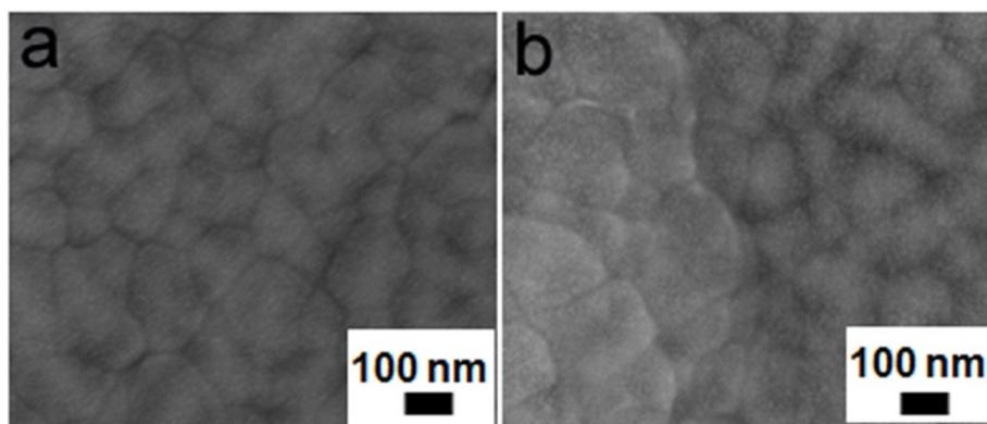
**Figure S4.** SEM images of NPG/PPy composites with the PPy plating time of (a) 20 s, (b) 30 s.
