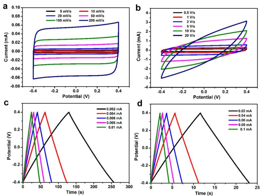
**Figure S18.** CV curves of NPG/PPy MSC with the PPy plating time of 10 s at scan rates ranging from (a) 5 to 200  $\text{mV s}^{-1}$ ; (b) 0.5 to 20  $\text{V s}^{-1}$ . Galvanostatic charge/discharge curves of NPG/PPy MSC with the PPy plating time of 10 s at different current from (c) 0.002 to 0.01 mA; (d) 0.02 to 0.1 mA.
