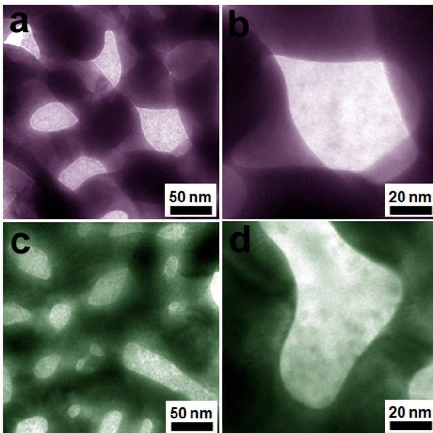
**Figure S7.** TEM images of NPG/MnO<sub>2</sub> (a) and NPG/PPy (c); High magnified TEM images of NPG/MnO<sub>2</sub> (b) and NPG/PPy (d).
