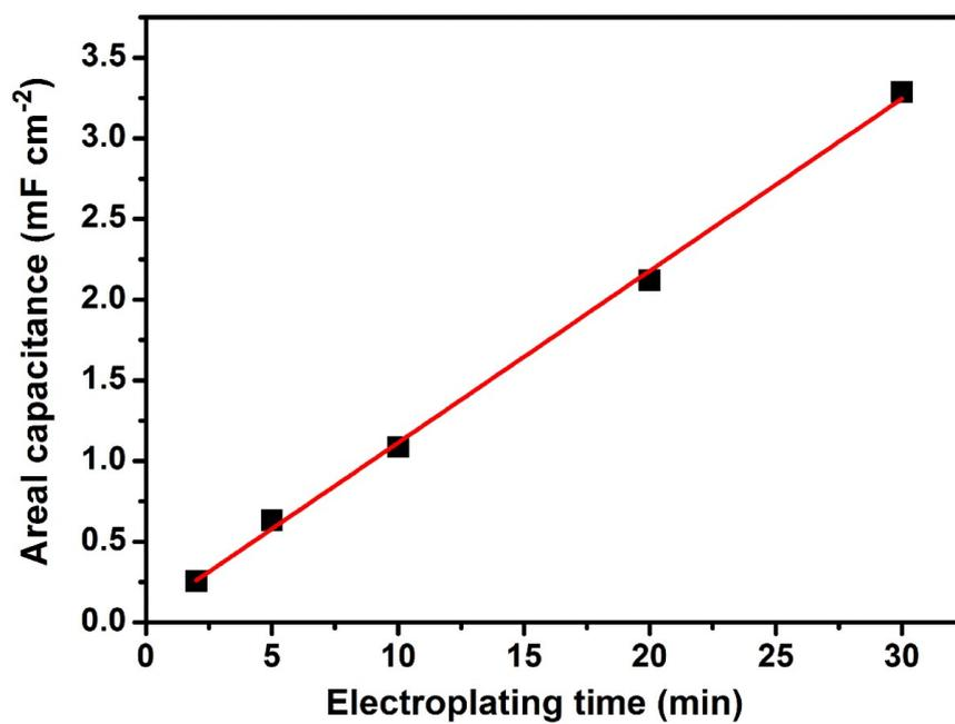
**Figure S14.** Areal capacitance of NPG/MnO<sub>2</sub> MSCs versus the MnO<sub>2</sub> plating time.
