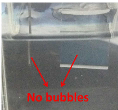
Fig. S21 Photographs of Pt wire cathode and ITO glass anode of the water-splitting cell driven by a 1.5 V AA battery.
