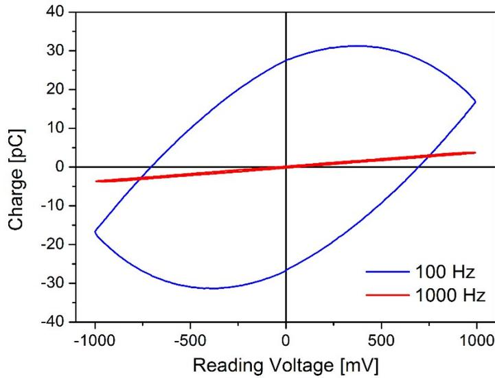
**Figure S4:** Charge/Voltage characteristic measured using triangle pulses at different frequencies: at low frequency (100 Hz, red line) the device shows a resistive behavior; increasing the frequency (1 KHz, blue line) a dielectric response is observed.
