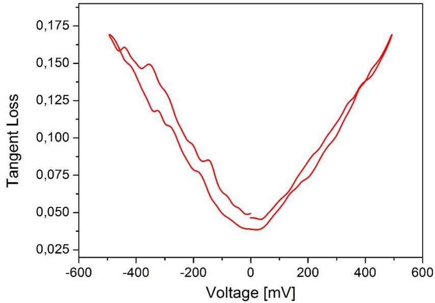
**Figure S5:**  $\tan(\delta)$  loss measured during the capacitance versus voltage measurement reported in Figure 3. The typical leakage-like trend is observed with little variation from the dielectric/capacitive regime.
