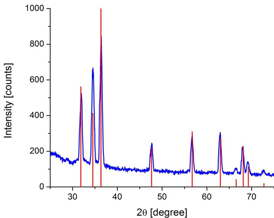
**Figure S2:** XRD pattern of as grown ZNR on CF is reported (blue), all peaks have been indexed as hexagonal ZnO (s.g. P63mc) according to JCPDS no. 79-0205 (red). Characterization is performed with a Thermo ARL X'tra diffractometer (Cu K $\alpha$  source,  $\Theta$ - $\Theta$  Bragg-Brentano geometry,  $10^{-4}$  degree accuracy).
