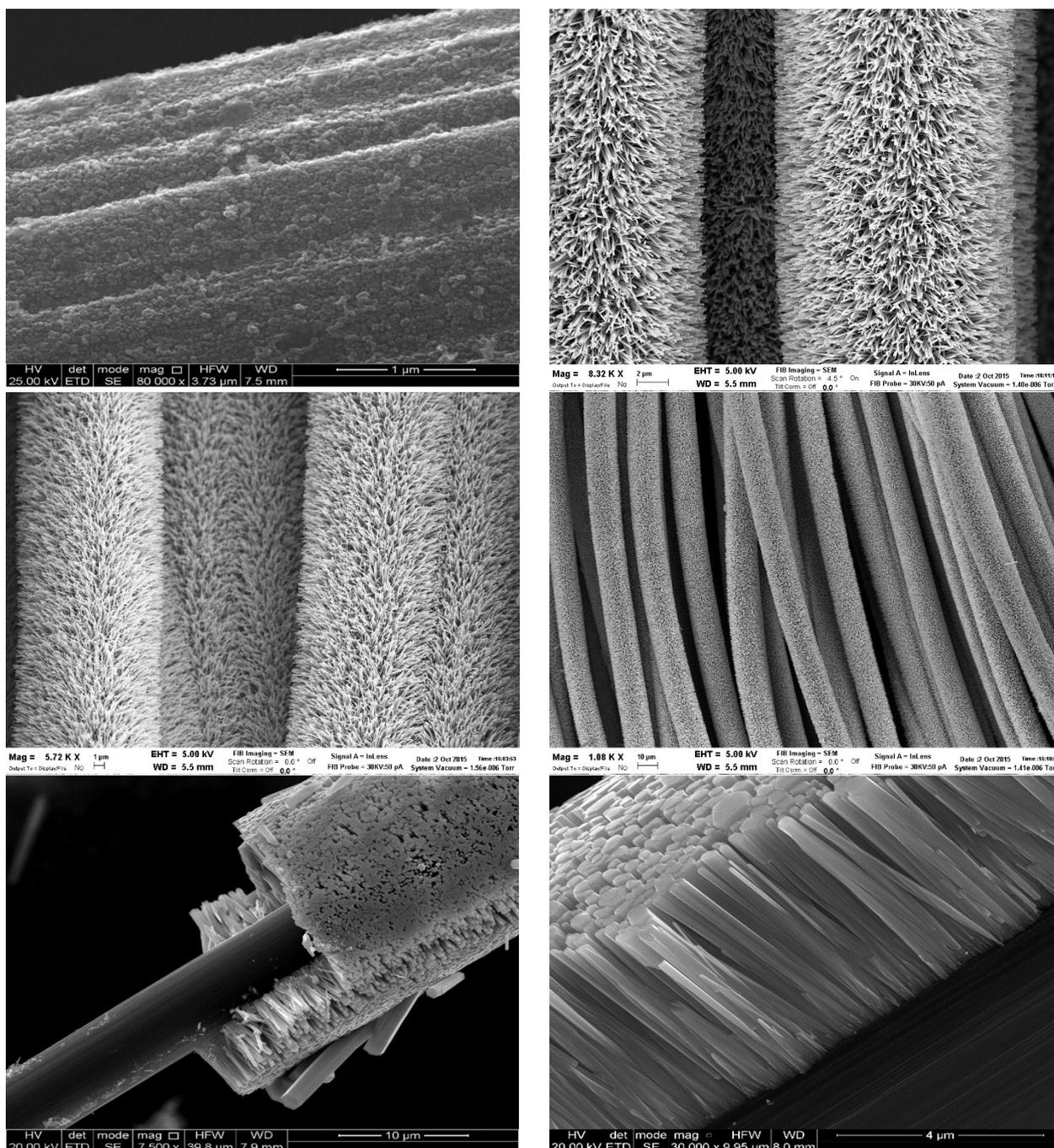
**Figure S1:** FE-SEM images of uniformly distributed seed layer deposited with SILAR technique (a); ZnO nanorods grown at different temperature / precursor concentration (b-f). Refer to methods section for further details.
