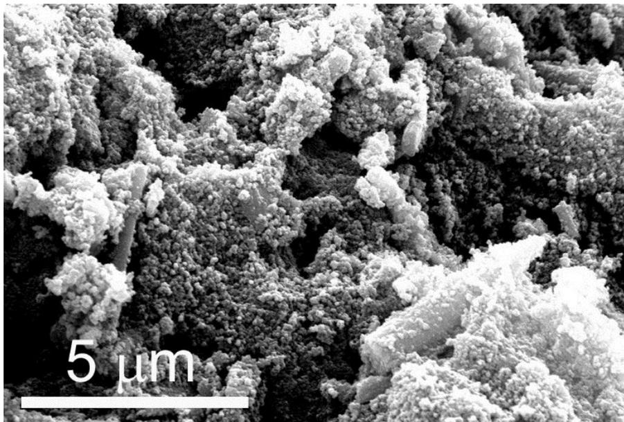
**Fig. S2** The cross-sectional SEM image of the composite photoanode film with 10 wt% CNCs.
