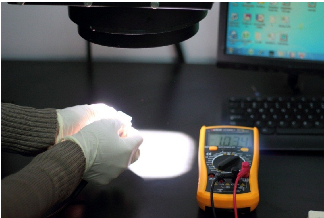
Fig. S8 Photograph of our testing result without metal mask for device I under AM1.5 solar light of 100 \text{ mW cm}^{-2} .
