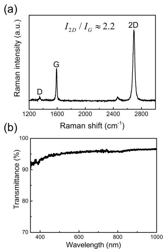
Figure S2. (a) Raman spectrum of monolayer Gr film measured on  $\text{SiO}_2/\text{Si}$  substrate and (b) light transmission spectrum of monolayer Gr film.
