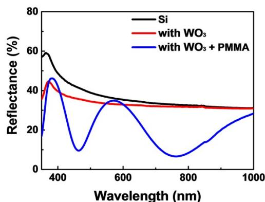
Figure S4. Reflectance spectra of Si, WO<sub>3</sub>/Si, and Gr/WO<sub>3</sub>/Si solar cell (PMMA/Gr/WO<sub>3</sub>/Si).
