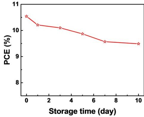
Figure S5. PCE of a Gr/WO<sub>3</sub>/Si solar cell exposed under ambient conditions.
