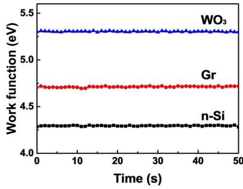
Figure S1. Work function of  $\text{WO}_3$ ,  $\text{Gr}$  and  $n\text{-Si}$  measured by a Kelvin probe under ambient conditions.
