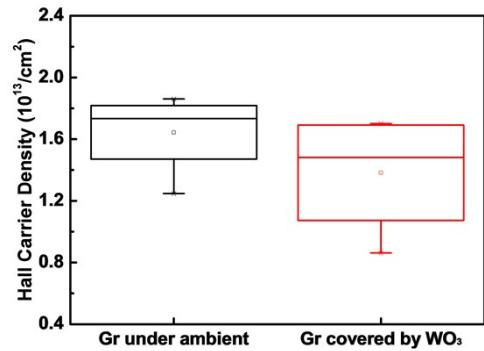
Figure S6. Carrier density of Gr under ambient condition and covered by WO<sub>3</sub> thin film measured by Hall Effect.
