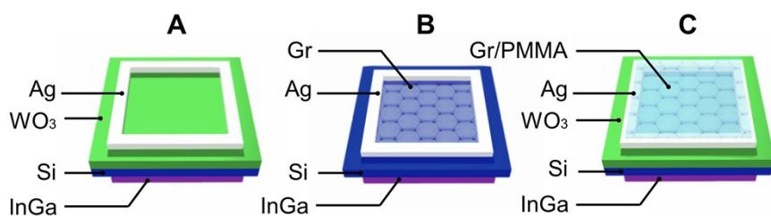
Figure S3. Schematic device structures of  $\text{WO}_3/\text{Si}$  solar cells (A),  $\text{Gr/Si}$  solar cells without (B) and with (C) a  $\text{WO}_3$  interlayer.
