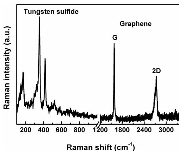
**Figure S1.** A typical Raman spectrum of WS<sub>2</sub> catalysts grown on graphene/Ni foam
