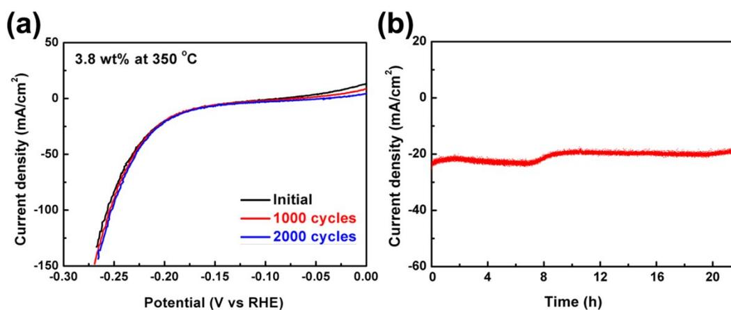
**Figure S4.** The stability test of WS<sub>2</sub> catalysts grown on three-dimensional graphene/Ni foam at 350 °C with the precursor concentration of 3.8 wt% in DMF. (a) Cyclability test with a scanning rate of 80 mV/s. (b) Time dependence of cathodic current density during electrolysis under a static overpotential of 200 mV for this sample.
