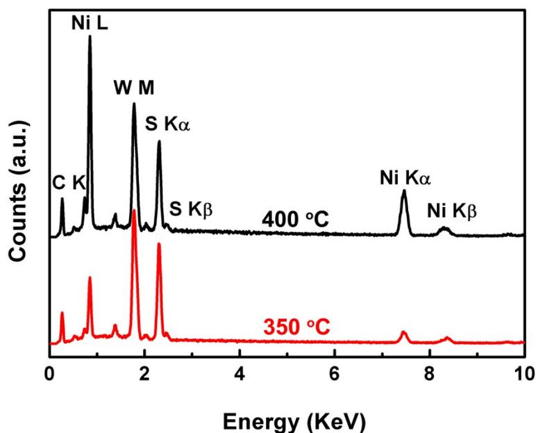
**Figure S2.** EDS analysis on the chemical composition of as-prepared WS<sub>2</sub> catalysts on three-dimensional graphene/Ni foam at different temperatures.
