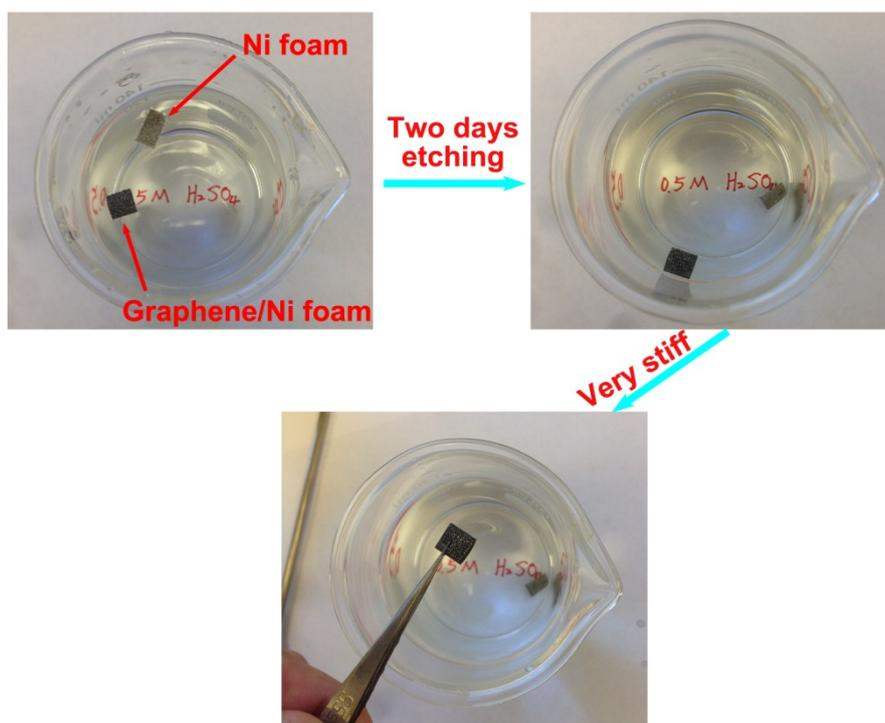
**Figure S3.** The protection of Ni foam from electrochemical erosion in 0.5 M H<sub>2</sub>SO<sub>4</sub> solution. After two days etching, it is obvious that not only Ni foam, but also graphene-covered Ni foam are still there
