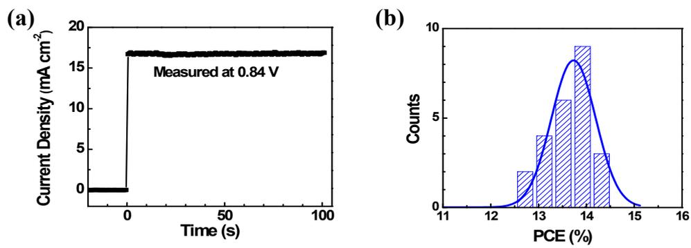
**Figure S9** (a) Steady-state photocurrent output at the maximum power point (0.84 V) for the flexible perovskite solar cells based on N-PDI (b) Histogram of PCE for the flexible devices based on N-PDI.
