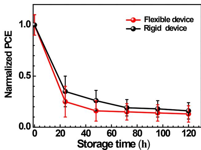
**Figure S10** Normalized cell efficiency plotted as a function of storage time for the PVSCs based on rigid and flexible substrates, the devices without encapsulation were stored under ambient conditions (relative humidity ca. 50%; temperature ca. 28 °C).
