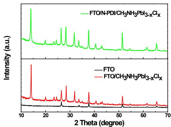
**Figure S1** XRD pattern of  $\text{MAPbI}_{3-x}\text{Cl}_x$  thin film on FTO and FTO/N-PDI. There is no distinct peaks at  $2\theta = 12.56^\circ$ , corresponding to the absence of typical diffractions of (001) planes for the unconverted  $\text{PbI}_2$ .
