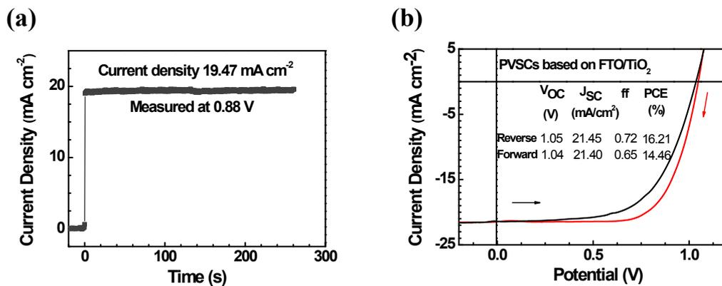
**Figure S7** (a) Steady-state photocurrent output at the maximum power point (0.88 V) for the N-PDI based devices (b) J-V curves of the perovskite solar cells based on FTO/TiO<sub>2</sub> with different scan directions.
