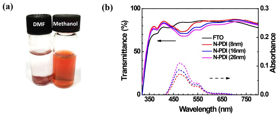
**Figure S3.** (a) Photograph of N-PDI in N, N-Dimethyl-formamide and methanol, showing the solubility of this material in different solvents. (b) Absorption (right ordinate) and transmittance (left ordinate) spectra of the FTO deposited with N-PDI interlayer by varying the thickness.
