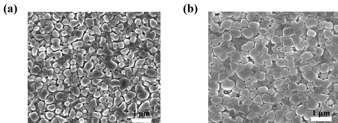
**Figure S6** Top-view SEM images of the  $\text{MAPbI}_{3-x}\text{Cl}_x$  films on (a) the FTO, and (b) the FTO/N-PDI substrates.
