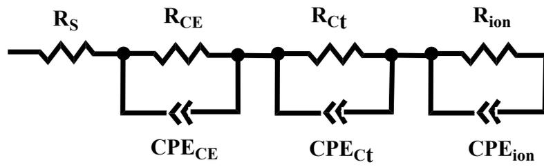
**Figure S8** The equivalent circuit with 3 lumped RC-circuits in series for fitting the impedance spectroscopy data obtained from the perovskite solar cells in this study.
