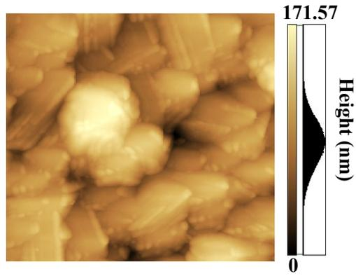
**Figure S4.** AFM image (size:  $2 \times 2 \mu\text{m}$ ) of the FTO substrate, showing a roughness of 17.16 nm.
