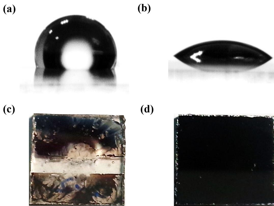
**Figure S2.** The contact angle of water on (a) FTO/C-PDI substrate, and (b) FTO/N-PDI substrate. Photograph of MAPbI<sub>3-x</sub>Cl<sub>x</sub> film on (c) FTO/C-PDI and (d) FTO/N-PDI substrates, respectively.
