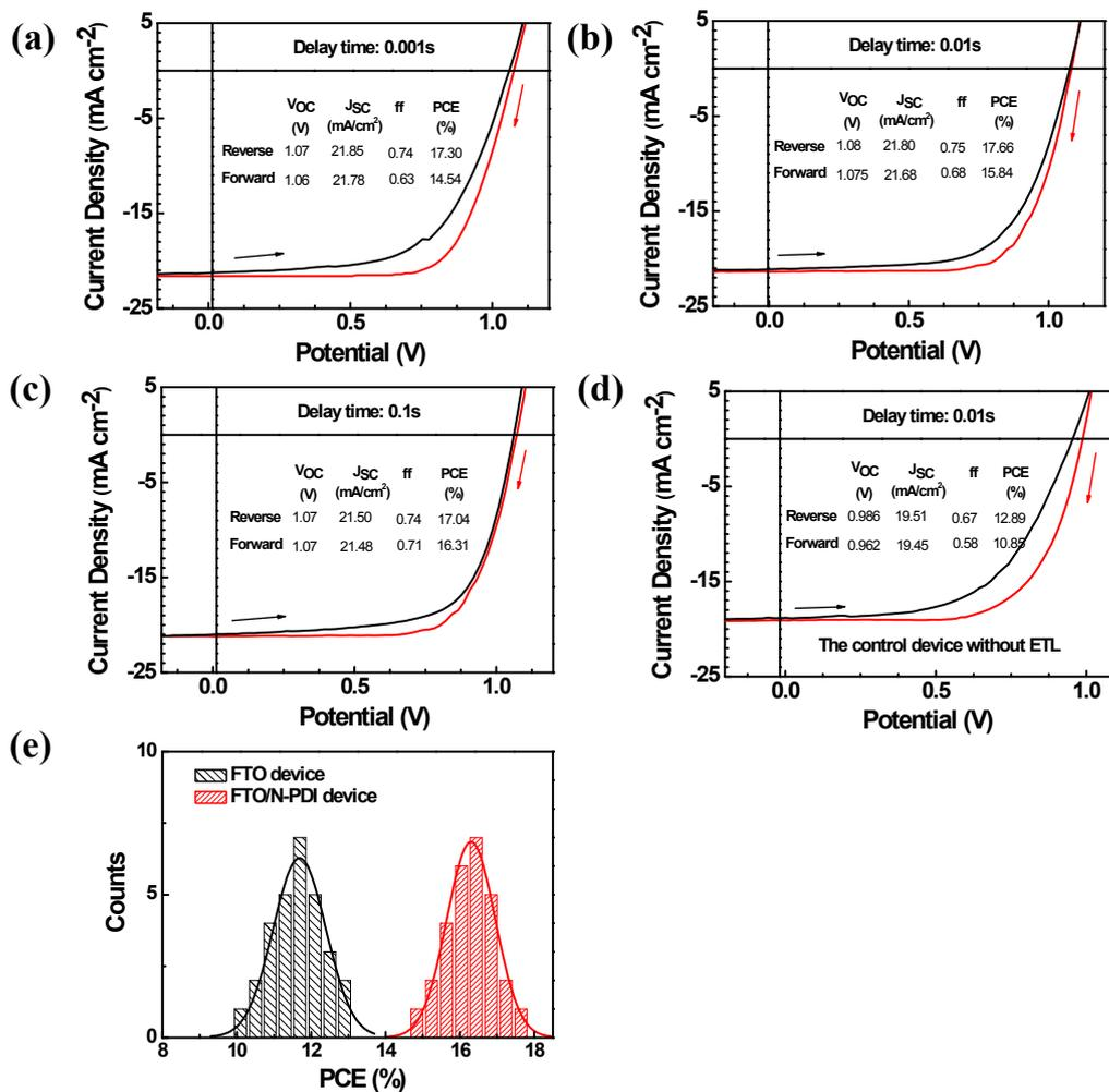
**Figure S5.** (a-c) Influence of scan rates on the current-voltage characteristics for the device based on FTO/N-PDI substrate (d) Current-voltage curves for the control device measured by forward and reverse scans at 20 mV per step with a delay time of 10 ms (e) Histogram of PCE for perovskite solar cells based on the FTO and FTO/N-PDI substrates.
