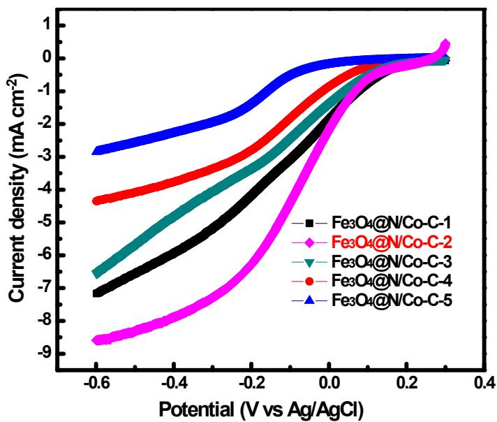
Fig. S11 LSV of  $\text{Fe}_3\text{O}_4@\text{N/Co-C}$  with different Fe/Co ratio at 1600 rpm  $\text{min}^{-1}$  in  $\text{O}_2$ -Saturated PBS solution.
