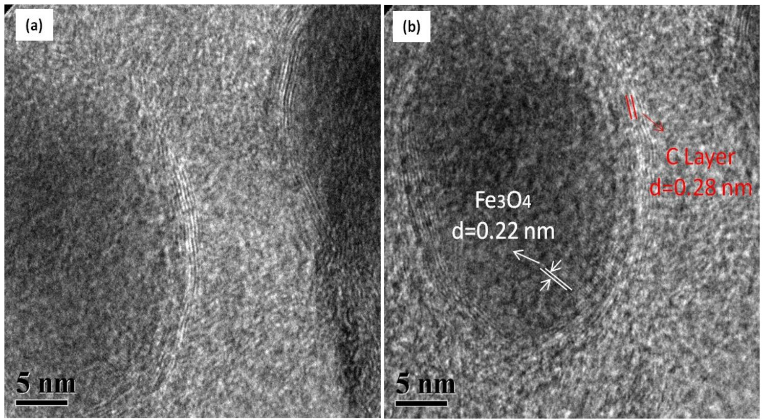
Fig. S4 The high-resolution TEM images of  $\text{Fe}_3\text{O}_4@\text{N/Co-C}$
