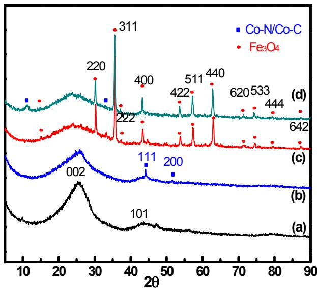
Fig. S5 The XRD patterns of (a) N-C, (b) N/Co-C, (c) Fe<sub>3</sub>O<sub>4</sub>@N-C and (d) Fe<sub>3</sub>O<sub>4</sub>@N/Co-C.
