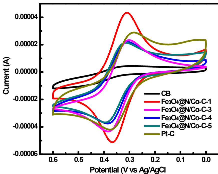
Fig. S9 Electrochemical BET: CV measured in ferrocyanide solution with different catalysts modified glass carbon electrodes.
