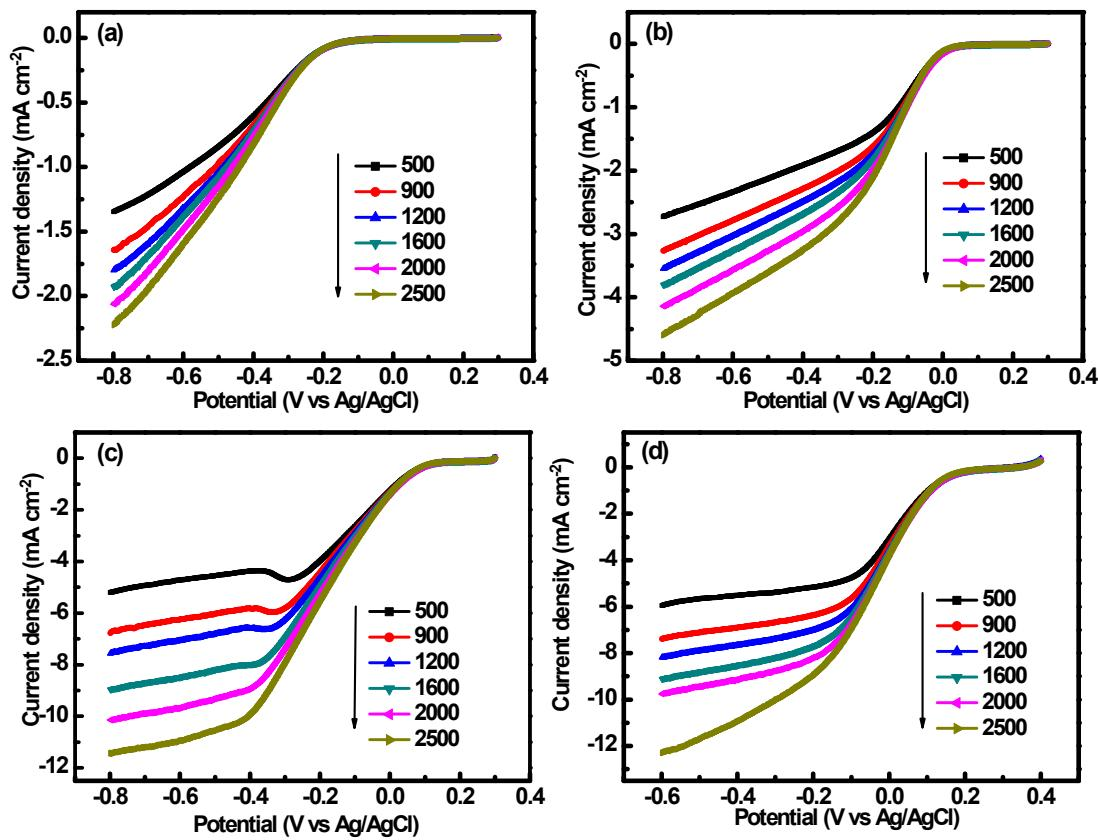
Fig. S7 LSV of N-C, N/Co-C, Fe<sub>3</sub>O<sub>4</sub>@N-C and Pt/C at different rotation speed from 500 to 2500  $\text{rpm min}^{-1}$  in PBS solution.
