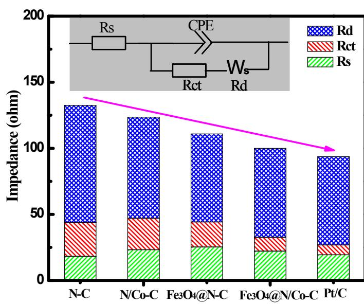
Fig. S13 The resistance composition of different catalysts (insert picture: characteristic equivalent electrocircuit).
