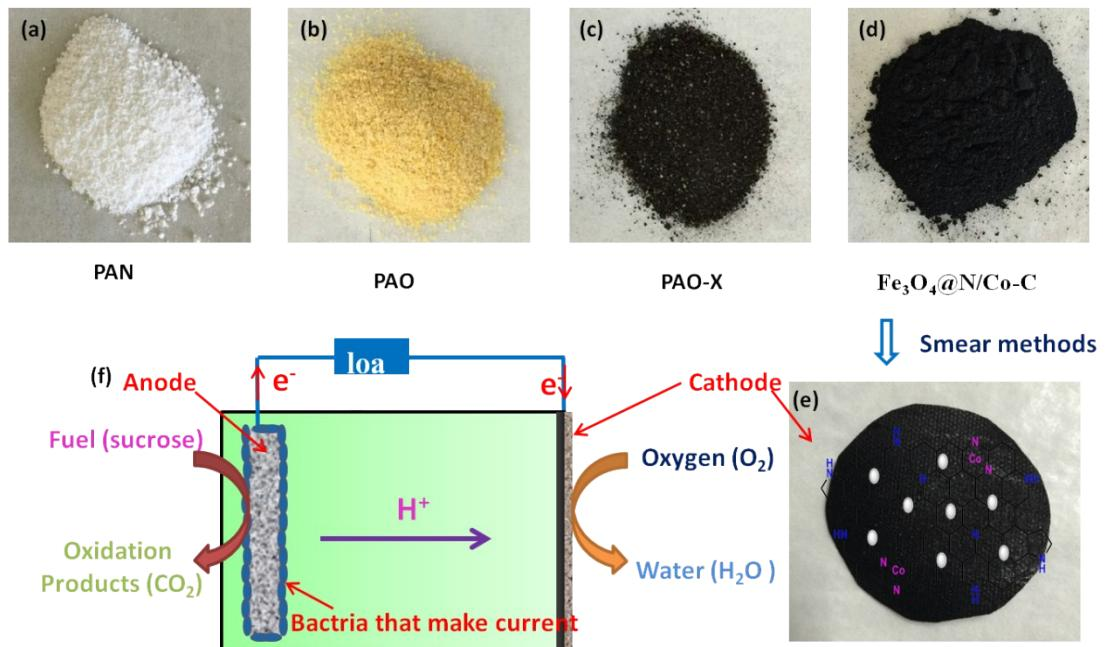
Fig.S1 (a) Polyacrylonitrile (PAN), (b) Polyacrylamidoxime (PAO), (c) metal-polymeric frameworks (PAO-X, X=Fe or Co), (d)  $\text{Fe}_3\text{O}_4@\text{N/Co-C}$ , (e) air-cathode of MFCs and (f) the configuration and working principles of MFCs.
