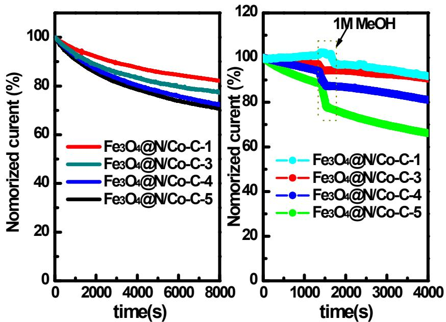
Fig. S12 The i-t curves (a) and the anti-toxic ability (b) of Fe<sub>3</sub>O<sub>4</sub>@N/Co-C with different Fe/Co ratio in O<sub>2</sub>-Saturated PBS solution.
