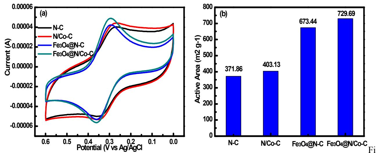
g. S6 Eletrochemical BET: (a) CV measured in ferrocyanide solution with different catalysts modified glass carbon electrodes; (b) eletrochemical active area calculated by Matsuda's equation
