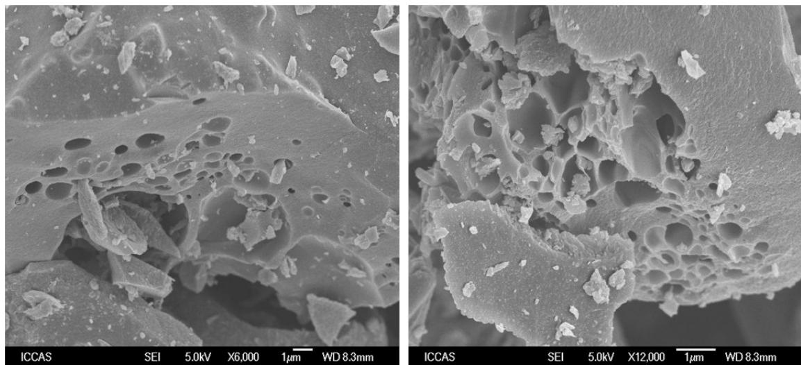
Fig.S2 The SEM images of carbon derived from PAN by carbonization
