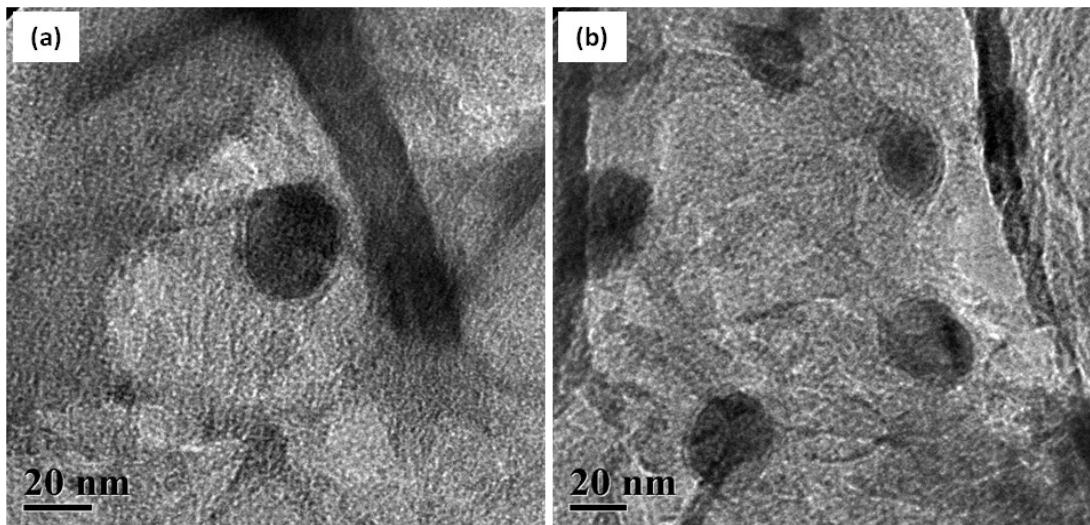
Fig.S3 The TEM images of  $\text{Fe}_3\text{O}_4@\text{N-C}$  (a) and  $\text{Fe}_3\text{O}_4@\text{N/Co-C}$  (b).
