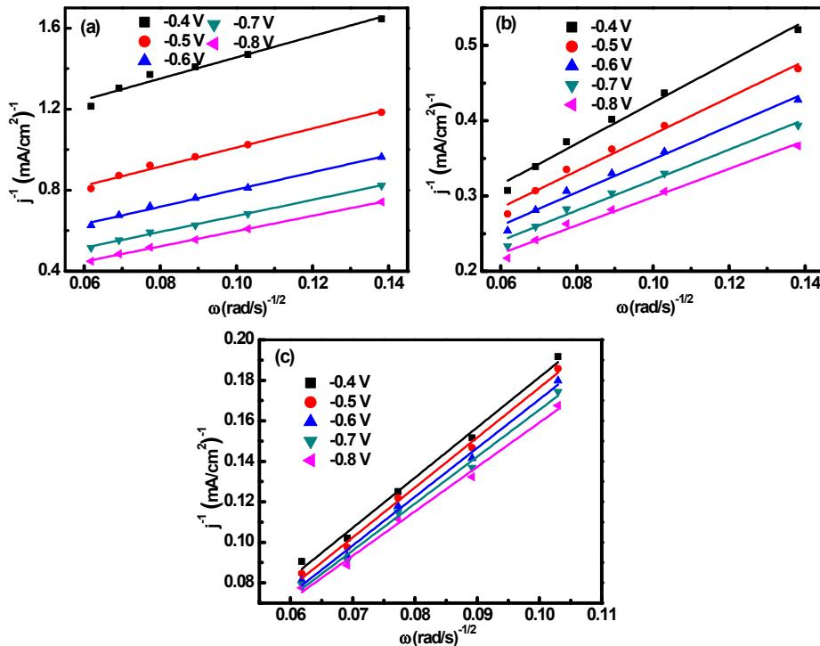
Fig. S8 The Koutecky–Levich plots measured by rotating disc electrode (RDE) in O<sub>2</sub>-saturated PBS solution: N-C (a), N/Co-C (b) and Fe<sub>3</sub>O<sub>4</sub>@N-C (c).
