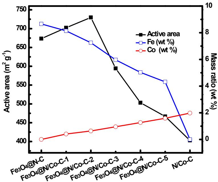
Fig. S10 The effect of Fe/Co ratio on the electrochemical active area.
