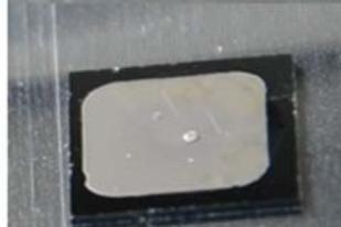
**Fig. S11** Re-absorption, after annealing at 250 °C for 5 minutes of the [70/30]/33 ionogel, of the IL, subsequent to its thermal expansion : photographs taken immediately (0 s) at the exit of the oven, and after 15 s and 30s.
