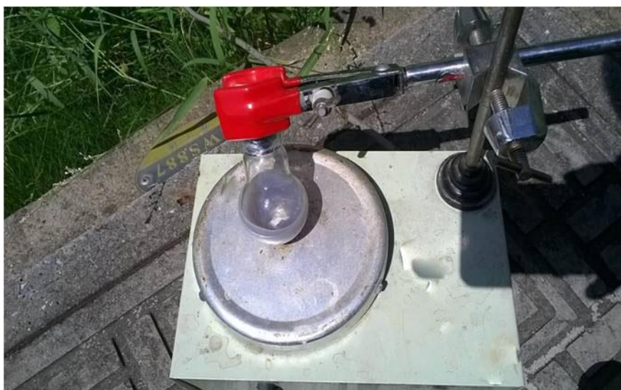
Figure S5. The photograph of outdoor equipment of sunlight-driven water splitting by Ni-7.4wt%/g-C 3 N 4 system in Wuxi city on June. 12, 2015. Outdoor temperature: 24~33°C, time: 09:30-17:00.
