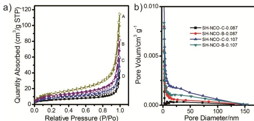
**Fig. S3** (a)  $N_2$ -sorption data of thiourethane bridged silsesquioxane aerogels: (A) SH-NCO-C-0.107, (B) SH-NCO-B-0.107, (C) SH-NCO-B-0.087, (D) SH-NCO-C-0.087. (b) Pore size distributions of the thiourethane bridged silsesquioxane aerogels.
