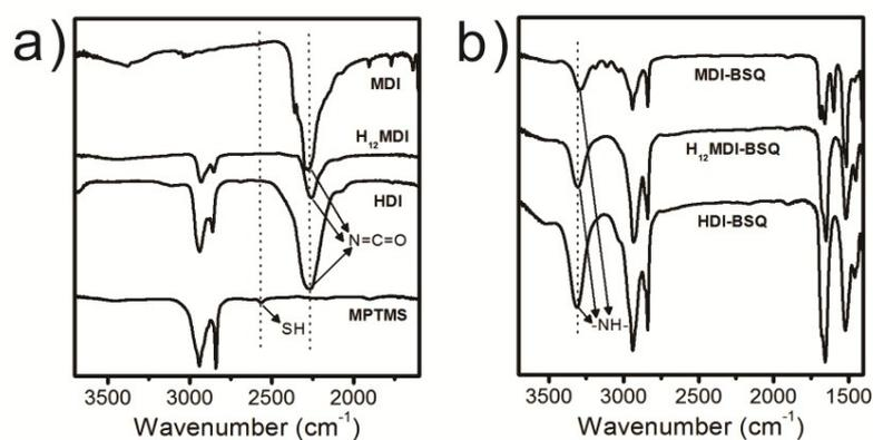
**Fig. S2** (a) FTIR spectra of MPTMS, HDI,  $\text{H}_{12}\text{MDI}$  and MDI. (b) FTIR spectra of HDI-BSQ,  $\text{H}_{12}\text{MDI-BSQ}$  and MDI-BSQ.
