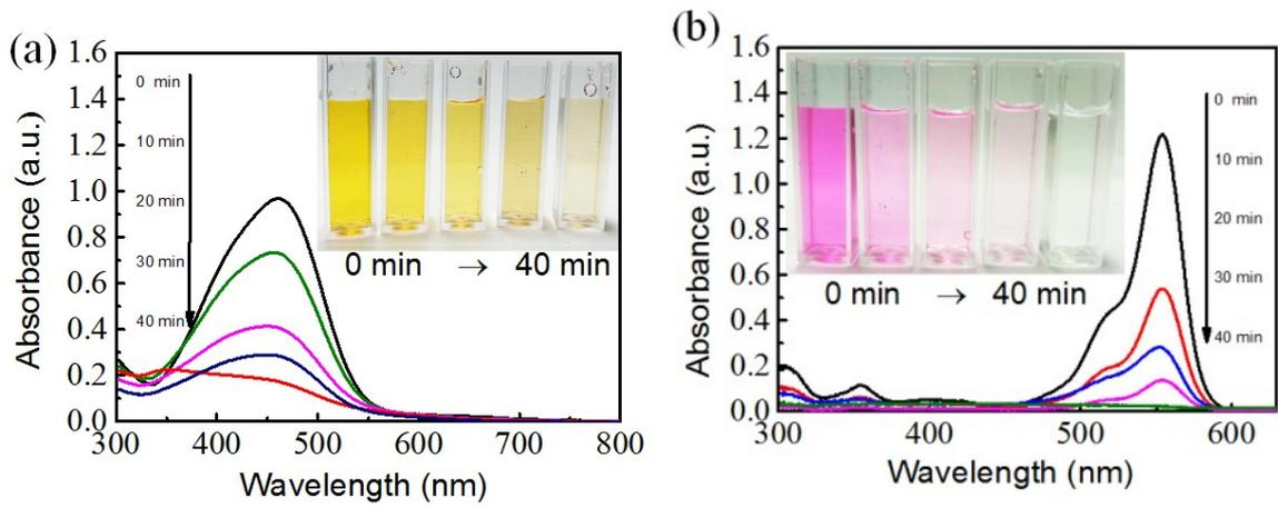
**Figure S2.** UV-Visible absorbance spectra for the photodegradation of (a) MO and (b) RhB under visible light over  $\text{Ag}_{10}\text{Si}_4\text{O}_{13}$  recorded after different degradation times. The insets shows the color changes of the MB (a) and RhB (b) solutions corresponding to the five degradation times from 0 min to 40 min.
