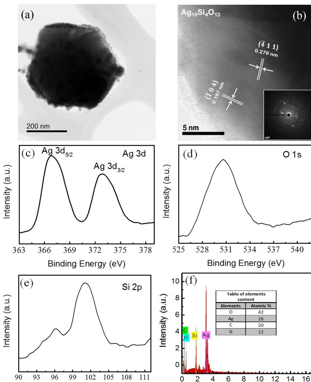
**Figure S1.** (a) TEM image and (b) HETEM image and inset SAED pattern. XPS spectra of  $\text{Ag}_{10}\text{Si}_4\text{O}_{13}$ : (c) Ag 3d, (d) O 1s, (e) Si 2p. The spectra demonstrate that the main peaks correspond to Ag  $3d_{5/2}$  and Ag  $3d_{3/2}$ , O 1s, and Si 2p orbitals for the  $\text{Ag}_{10}\text{Si}_4\text{O}_{13}$ ; (f) EDS spectrum of elements and the inset is a table of elements content percentage corresponding to the  $\text{Ag}_{10}\text{Si}_4\text{O}_{13}$ .
