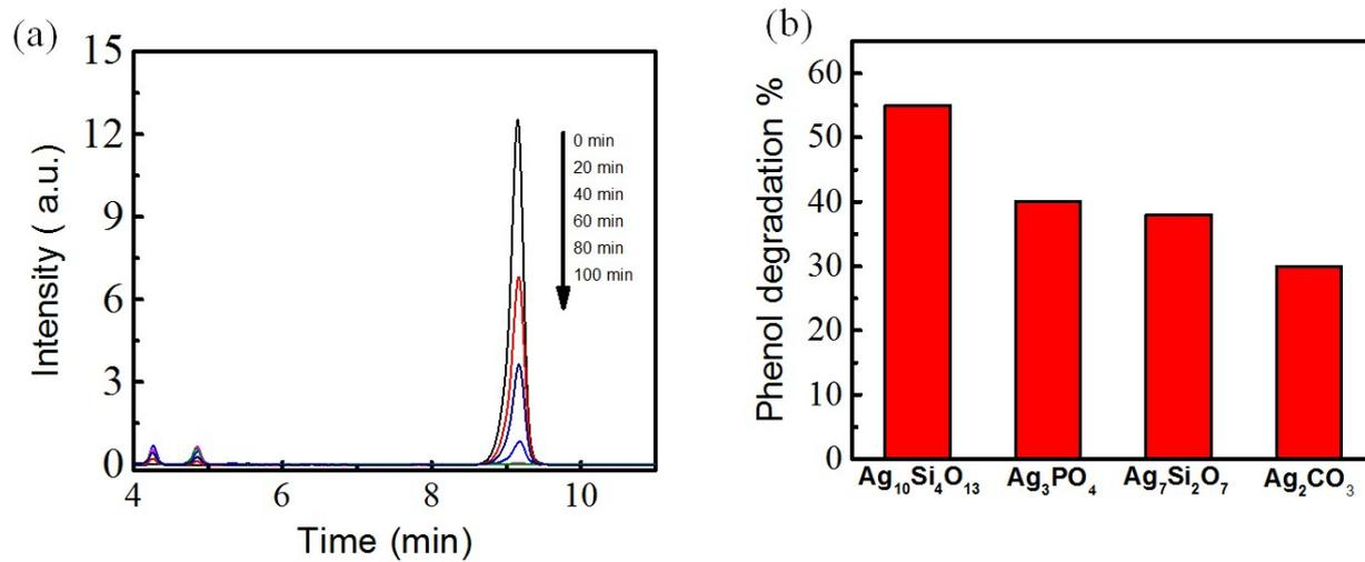
**Figure S4.** (a) High performance liquid chromatography (HPLC) spectra of phenol under visible light over  $\text{Ag}_{10}\text{Si}_4\text{O}_{13}$  (b) Photodegradation of phenol within 20 min over different Ag-incorporated p-block photocatalysts. References :  $\text{Ag}_2\text{CO}_3$ <sup>1</sup>,  $\text{Ag}_3\text{PO}_4$ <sup>2</sup>,  $\text{Ag}_7\text{Si}_2\text{O}_7$ <sup>3</sup>,  $\text{Ag}_{10}\text{Si}_4\text{O}_{13}$  our work
