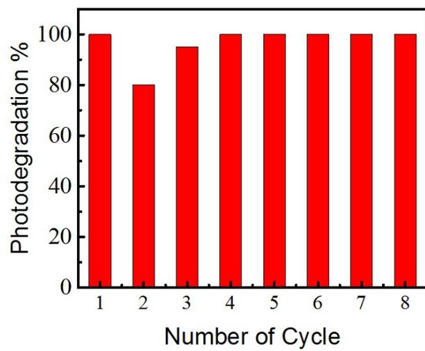
**Figure S3.** Cycling runs in the photodegradation of RhB over  $\text{Ag}_{10}\text{Si}_4\text{O}_{13}$ .
