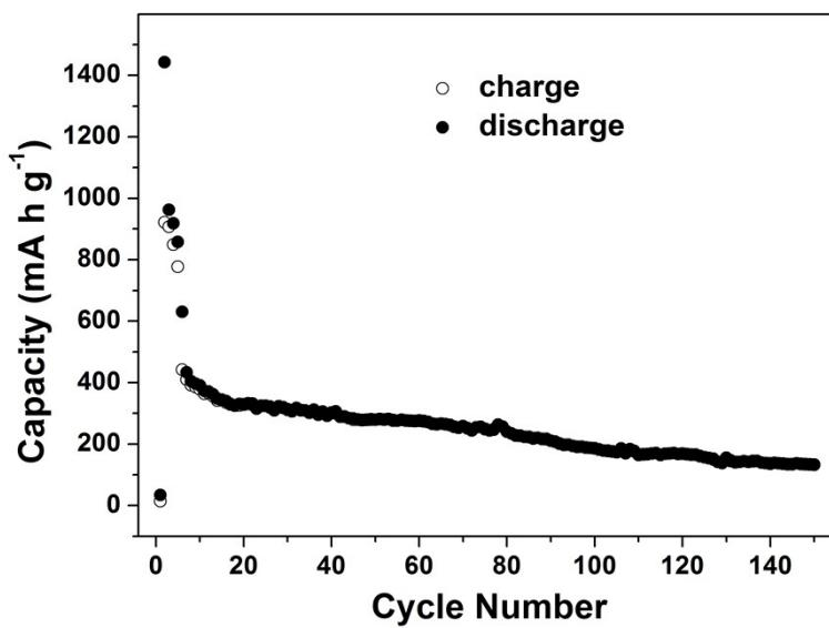
**Figure S5.** Cycling performance of the pure  $\text{SnS}_2$  electrode for LIBs at  $0.8 \text{ A g}^{-1}$ , being cycled at  $0.2 \text{ A g}^{-1}$  for the first five cycles.
