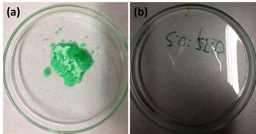
**Figure S10.** Photos of (a)  $[\text{Ni}(\text{H}_2\text{O})_6](\text{NO}_3)_2$  and (b) F127 in oven set at 80 °C after 12 h.
