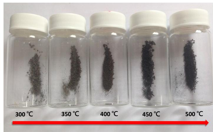
**Figure S7.** Photos of NiO/Ni prepared at calcination temperatures from 300 to 500 °C.
