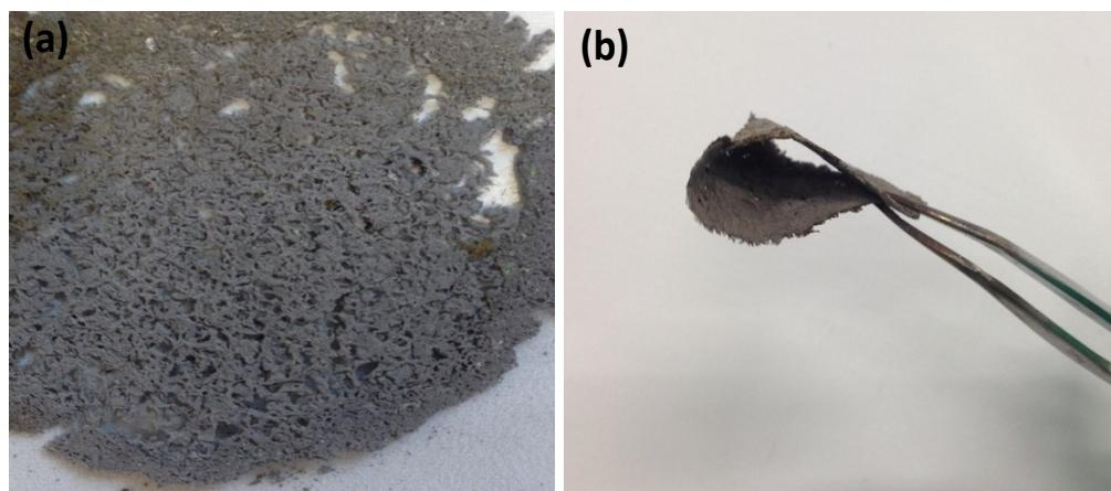
**Figure S4.** Photos of Ni foam (a) after being compressed into a disk and (b) the disk being further bent.
