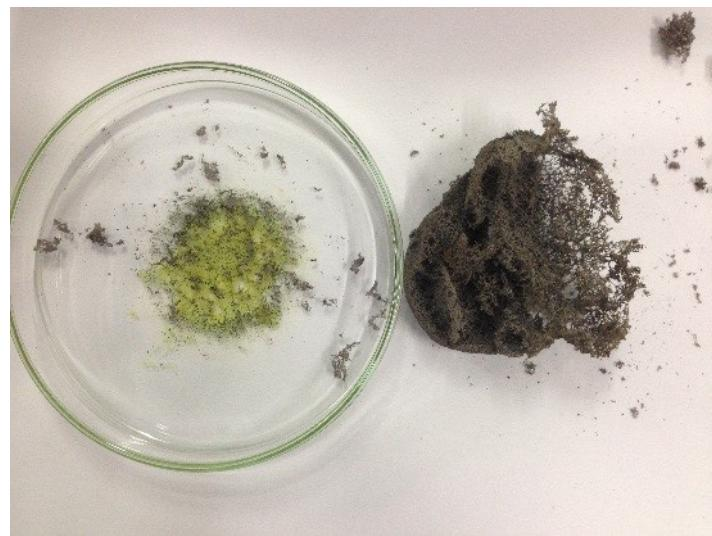
**Figure S2.** Photo of Ni foam and green residues on Petri dish obtained through calcination of  $[\text{Ni}(\text{H}_2\text{O})_{6-x}](\text{NO}_3)_2/\text{F}127$  dough at 200 °C for 1 h in air.
