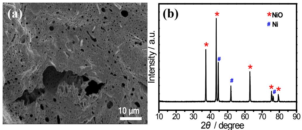
**Figure S6.** (a) SEM image and XRD pattern of Ni foam prepared at precursor composition of 0.5 g F127 and 2.9 g  $[\text{Ni}(\text{H}_2\text{O})_6](\text{NO}_3)_2$ .
