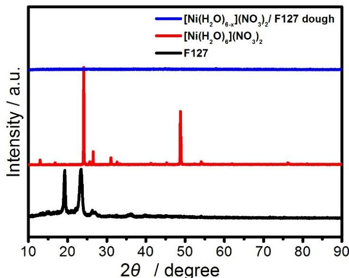
**Figure S1.** XRD patterns of F127,  $[Ni(H_2O)_6](NO_3)_2$ , and  $[Ni(H_2O)_{6-x}](NO_3)_2$ /F127 dough.
