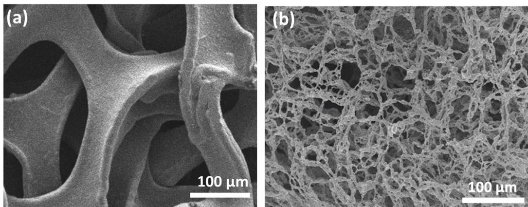
**Figure S5.** SEM images of (a) commercial Ni foam and (b) as-prepared Ni foam.
