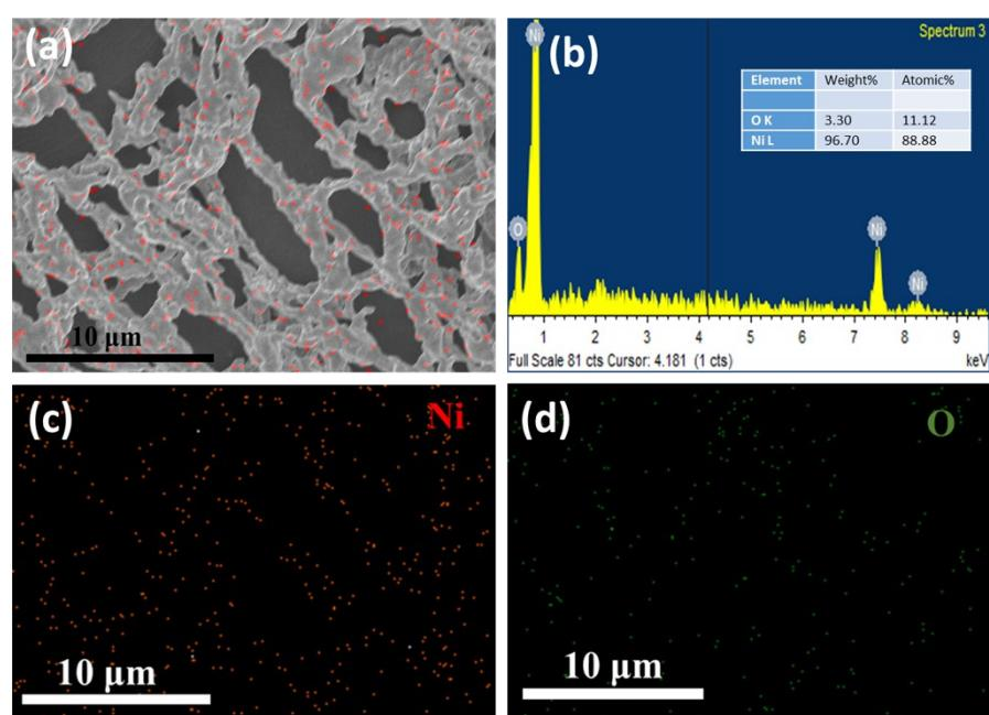
**Figure S3.** (a) SEM image of Ni foam, (b) EDX spectrum of Ni foam and elemental mapping images of (c) Ni and (d) O.
