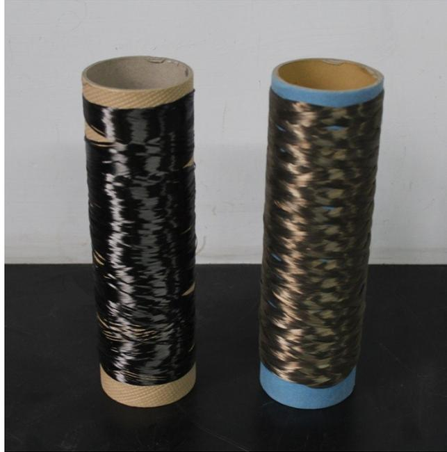
**Figure S1.** Photograph of CF (left) and CF@Ni (right).
