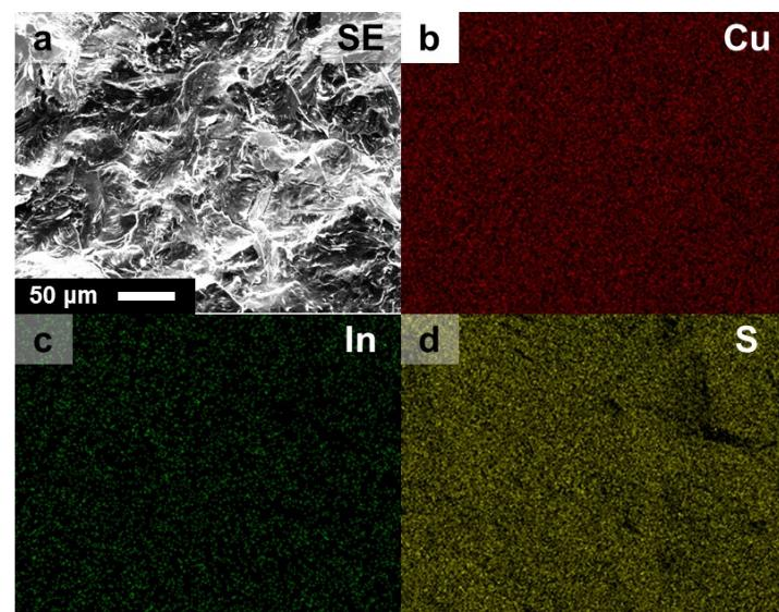
**Supplementary Figure S2.** EDX elemental maps of  $\text{Cu}_2\text{S}-1\%\text{In}_2\text{S}_3$ . **a.** SE. **b.** Cu. **c.** In. **d.** S.
