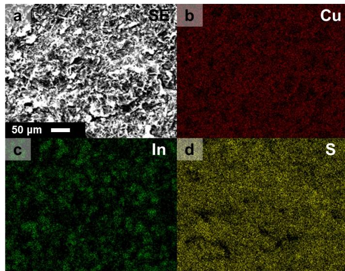
**Supplementary Figure S5.** EDX elemental maps of Cu<sub>2</sub>S-10%In<sub>2</sub>S<sub>3</sub>. **a.** SE. **b.** Cu. **c.** In. **d.** S.
