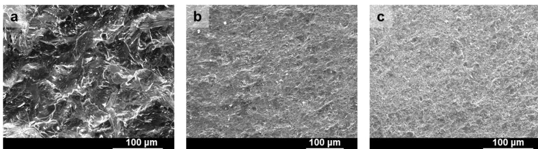
**Supplementary Figure S1.** SEM images of  $\text{Cu}_2\text{S}-x\%\text{In}_2\text{S}_3$  ( $x=1, 5$  and  $10$ ). **a.**  $\text{Cu}_2\text{S}-1\%\text{In}_2\text{S}_3$ . **b.**  $\text{Cu}_2\text{S}-5\%\text{In}_2\text{S}_3$ . **c.**  $\text{Cu}_2\text{S}-10\%\text{In}_2\text{S}_3$ .
