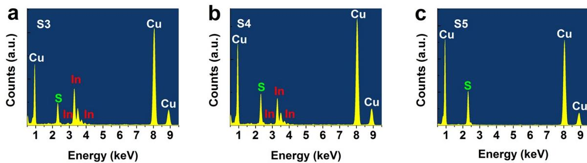
**Supplementary Figure S6.** EDX spectra of  $\text{Cu}_2\text{S}-2\%\text{In}_2\text{S}_3$  for different spots. **a.** Spot3 (S3). **b.** Spot4 (S4). **c.** Spot5 (S5).
