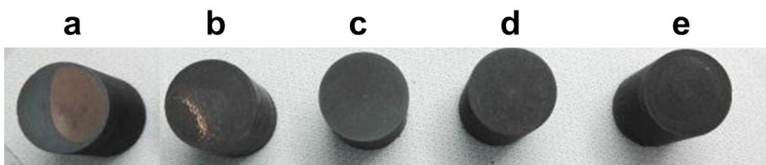
**Supplementary Figure S7.** Images of sintered  $\text{Cu}_2\text{S}-x\%\text{In}_2\text{S}_3$  ( $x=0, 1, 2, 5$  and  $10$ ) columns by SPS. **a.**  $\text{Cu}_2\text{S}$ . **b.**  $\text{Cu}_2\text{S}-1\%\text{In}_2\text{S}_3$ . **c.**  $\text{Cu}_2\text{S}-2\%\text{In}_2\text{S}_3$ . **d.**  $\text{Cu}_2\text{S}-5\%\text{In}_2\text{S}_3$ . **e.**  $\text{Cu}_2\text{S}-10\%\text{In}_2\text{S}_3$ .
