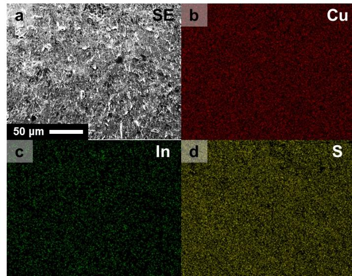
**Supplementary Figure S3.** EDX elemental maps of  $\text{Cu}_2\text{S}-2\%\text{In}_2\text{S}_3$ . **a.** SE. **b.** Cu. **c.** In **d.** S.
