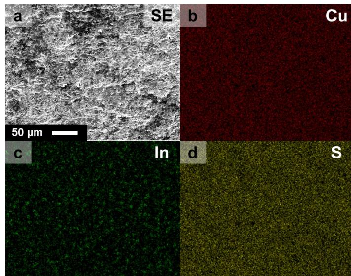
**Supplementary Figure S4.** EDX elemental maps of Cu<sub>2</sub>S-5%In<sub>2</sub>S<sub>3</sub>. **a.** SE. **b.** Cu. **c.** In. **d.** S.
