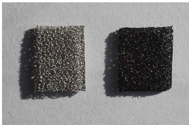
Fig. S1 Optical photographs of the NF substrate (left) and the \text{CoO}_x\text{-CoSe/NF} film on NF (right).
