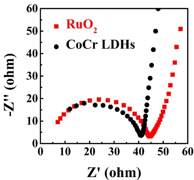
**Figure S4.** Nyquist plots of CoCr LDH and  $\text{RuO}_2$ .
