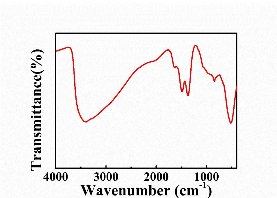
**Figure S9.** The FTIR pattern of amorphous Cr hydroxide.
