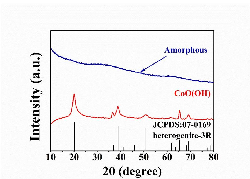
**Figure S8.** The XRD patterns of Co and Cr hydroxide.
