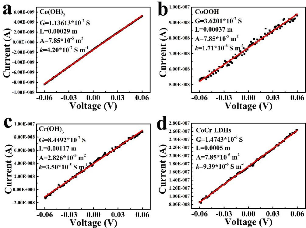
**Figure S5.** The I-U curve by LSV measurements of (a)  $\text{Co}(\text{OH})_2$ , (b)  $\text{CoOOH}$ , (c)  $\text{Cr}(\text{OH})_3$  and (d) CoCr LDH.
