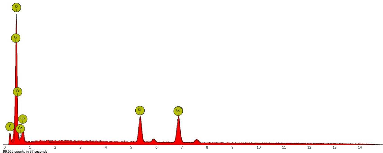
**Figure S1.** Energy dispersive X-ray spectrum of CoCr LDH powder (2:1).
