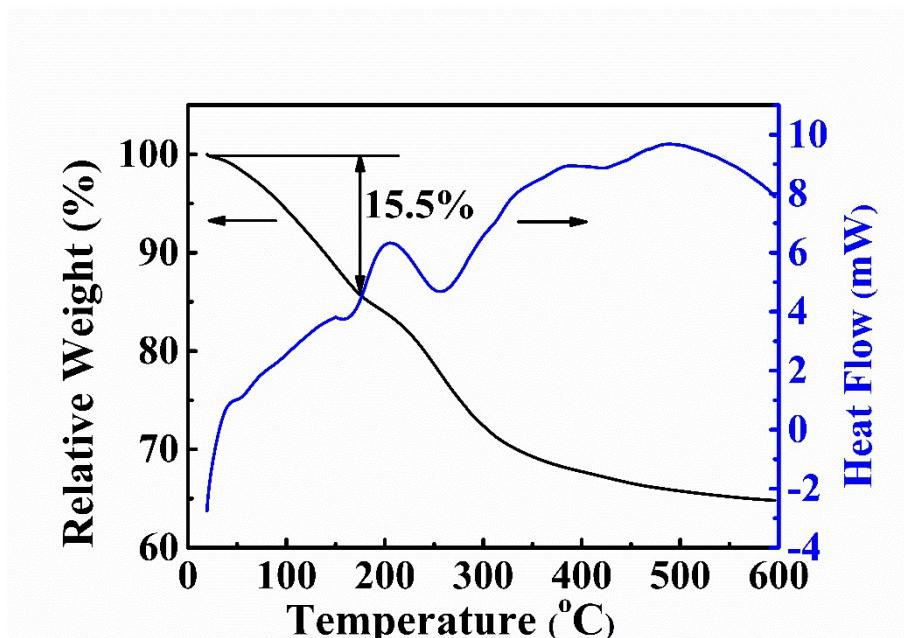
**Figure S2.** The TG/DSC curves of CoCr LDH (2:1)
