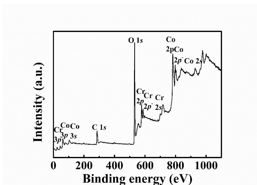
**Figure S3.** The XPS survey of CoCr LDH (2:1)
