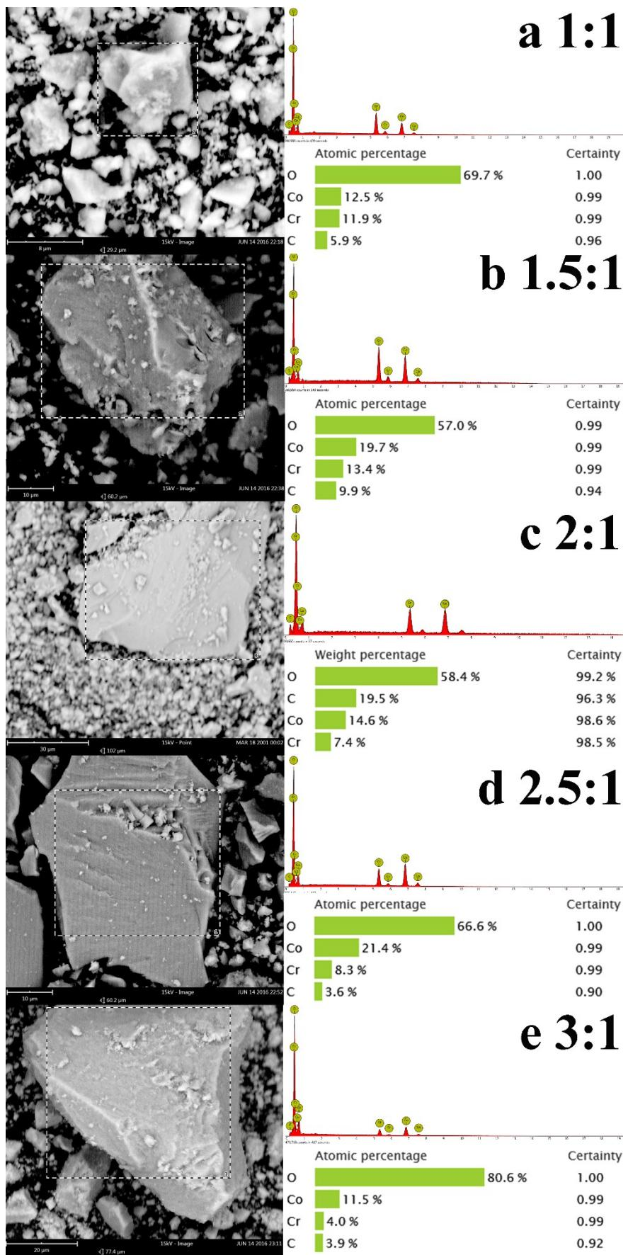
**Figure S7.** The SEM-EDX patterns of CoCr LDH with different ratios of Co to Cr.
