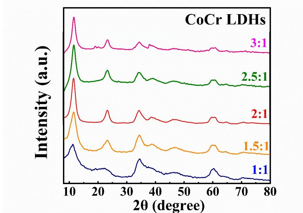
**Figure S6.** The XRD patterns of CoCr LDH with different ratios of Co to Cr.
