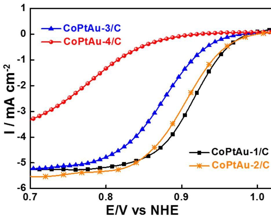
**Figure S6.** The LSV results of various CoPtAu/C samples recorded in 0.5 M HClO<sub>4</sub> saturated with O<sub>2</sub>.
