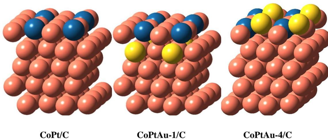
**Figure S1.** Surface models of CoPt/C, CoPtAu-1/C and CoPtAu-4/C electrodes. Blue, yellow and orange spheres are represented as Pt, Au and Co atoms, respectively.
