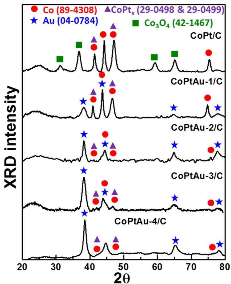
**Figure S2.** XRD patterns of CoPt/C and CoPtAu/C samples catalysts. Besides the peak of C support located at around  $25^\circ$ , characteristic peaks of  $\text{Co}_3\text{O}_4$  (JCPDS 42-1467) noted at  $31.3$ ,  $36.9$ ,  $59.4$ , and  $65.2^\circ$  are attributed to the diffractions of (220), (311), (511), and (440), respectively. When Au is added, strong Au peaks are noted at  $38.2$ ,  $44.4$ ,  $64.6$ , and  $77.5^\circ$  (04-0784).
