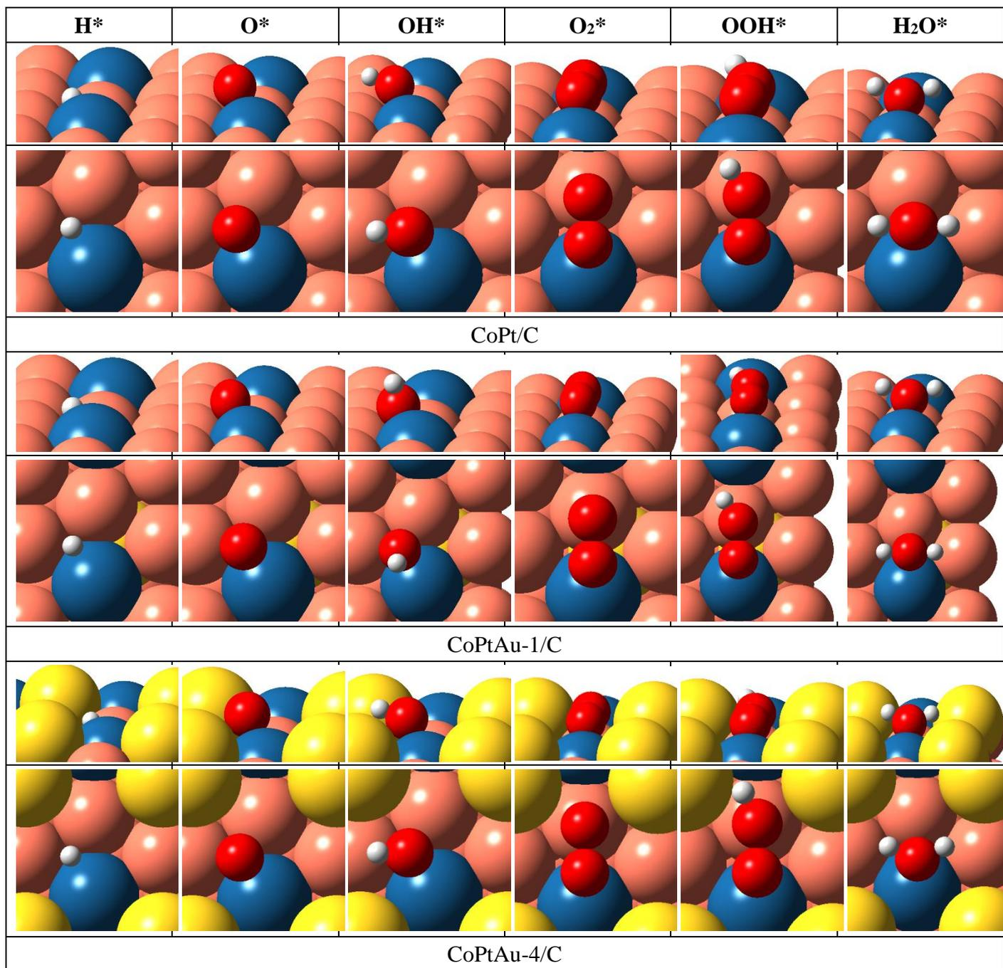
**Figure S4.** Optimized structures for H\*, O\*, OH\*, O<sub>2</sub>\*, OOH\* and H<sub>2</sub>O\* on CoPt/C, CoPtAu-1/C and CoPtAu-4/C. The corresponding  $E_{ads}$  are listed in Table S2. Blue, yellow, orange, red and white spheres are represented as Pt, Au, Co, O and H atoms, respectively.
