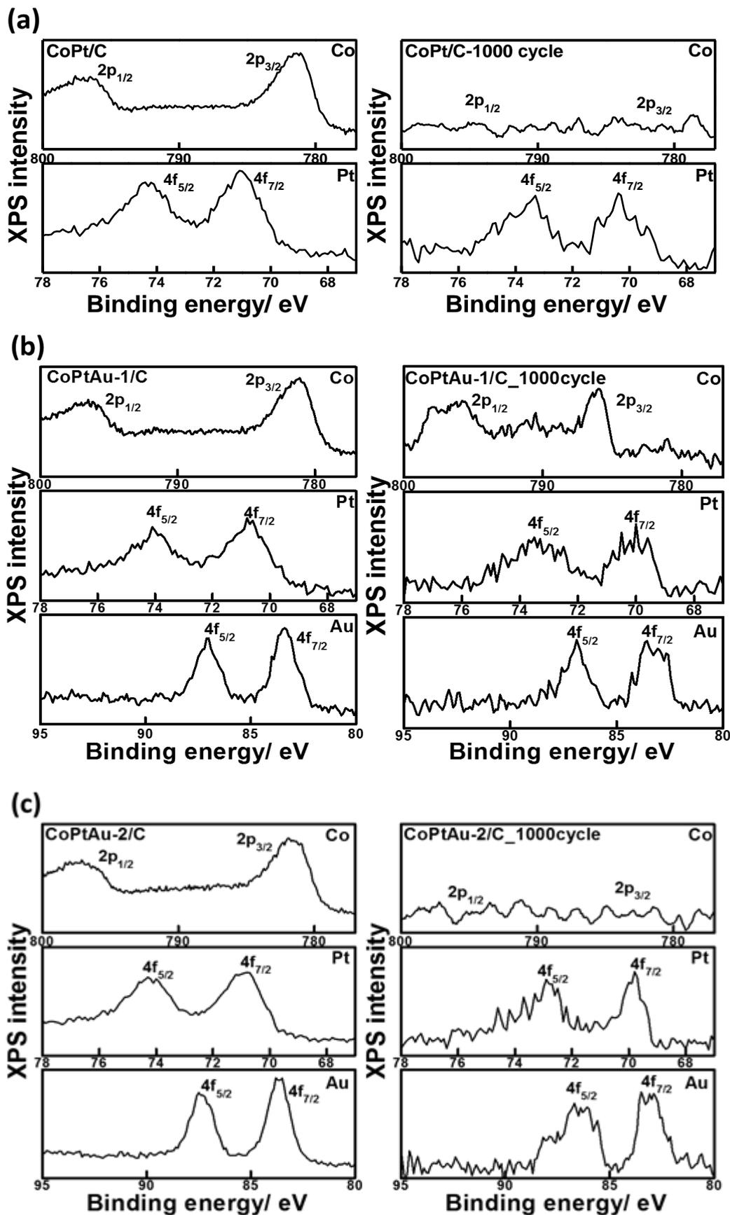
**Figure S3.** The XPS spectra of (a)CoPt/C, (b) CoPtAu-1/C, and (c) CoPtAu-2/C samples before and after ADT.
