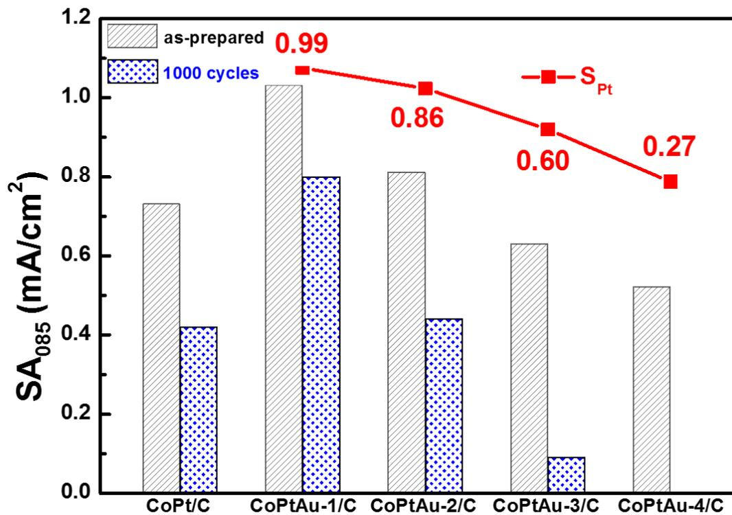
**Figure S7** The SA before and after ADT and  $S_{Pt}$  of CoPt/C and CoPtAu/C samples.
