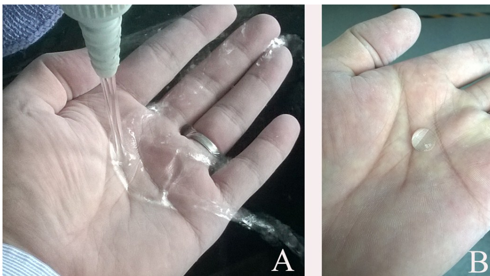
Figure S13. Photo images of (A) invisible glove washed by running water, and (B) after 15 min washing, the invisible glove is still works as the formation of water droplet on the hand.
