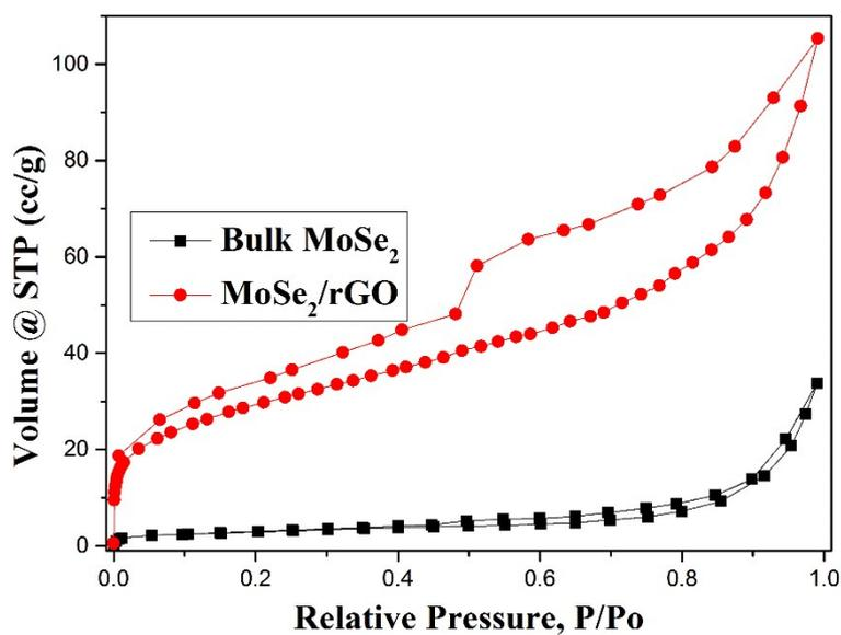
**Figure S6.** Nitrogen adsorption-desorption isotherms of MoSe<sub>2</sub> and MoSe<sub>2</sub>/rGO.
