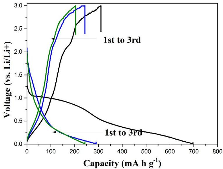
**Figure S3.** Charge-discharge curves of the first three cycles of bulk MoSe<sub>2</sub> at 100 mA g<sup>-1</sup>.
