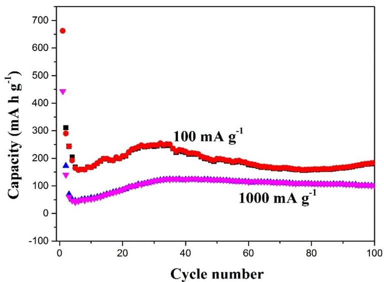
**Figure S4.** Cycling performance and coulombic efficiency of bulk MoSe<sub>2</sub>.
