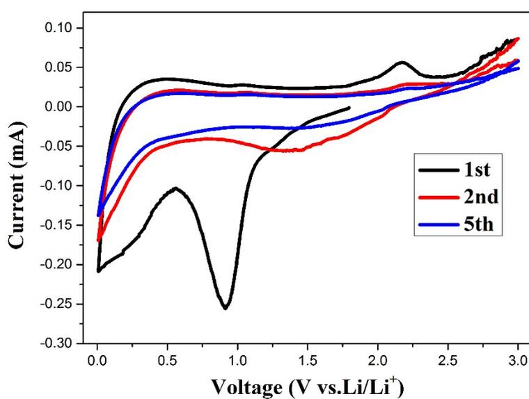
**Figure S2.** The cyclic voltammetry (CV) curves of the selected cycles for bulk  $\text{MoSe}_2$  at a scan rate of  $0.1 \text{ mV s}^{-1}$ .
