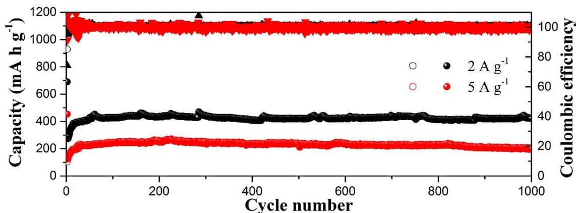
**Figure S5.** Cycling performance and coulombic efficiency of MoSe<sub>2</sub>/rGO hybrids at 2 and 5 A g<sup>-1</sup>.
