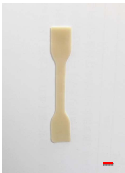
Figure S8. Dumbbell-shaped specimen for underwater tensile test. The scale bar represents 4 mm in length.
