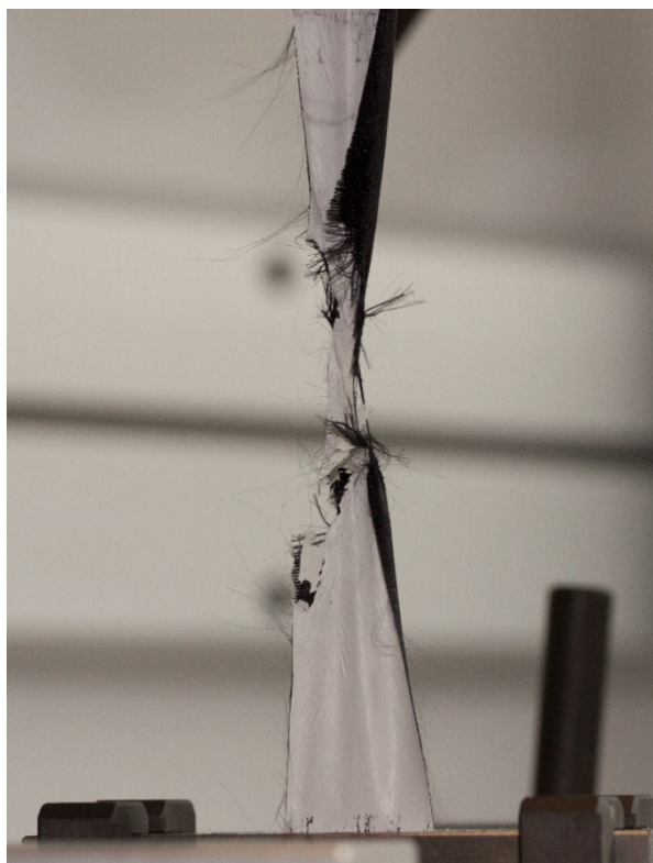
Figure S4. Laminate of nylon fabric, polymer adhesive and membrane (produced with coated template particles), which was ripped in a tensile test.
