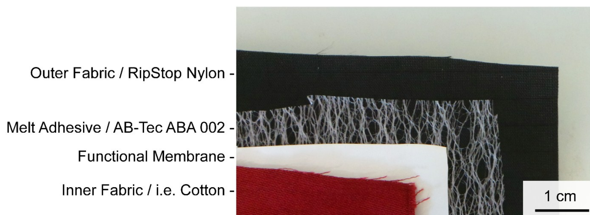
Figure S1. A typical built-up of a 3 layer laminate. The shown materials are exemplary, many variations are used.
