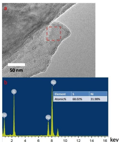
Figure S2 HRTEM of amorphous NiS<sub>2</sub> (a) and EDS of the marked position in figure S3a (b).
