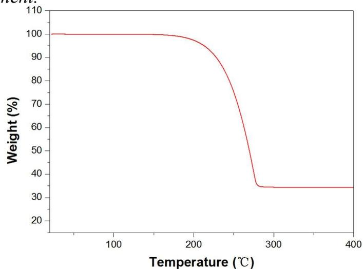
Figure S4 TGA curve of the S@a-NiS<sub>2</sub> composite measured in a nitrogen environment.
