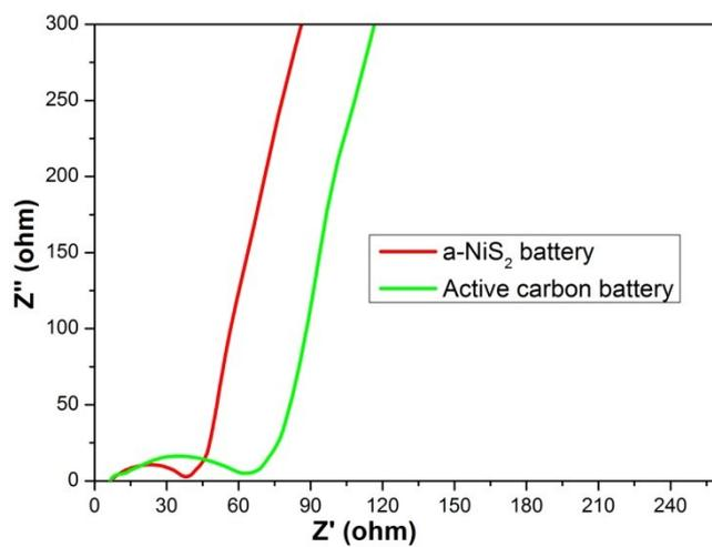
Figure S8 Electrochemical impedance of a-NiS<sub>2</sub> battery and active carbon battery.
