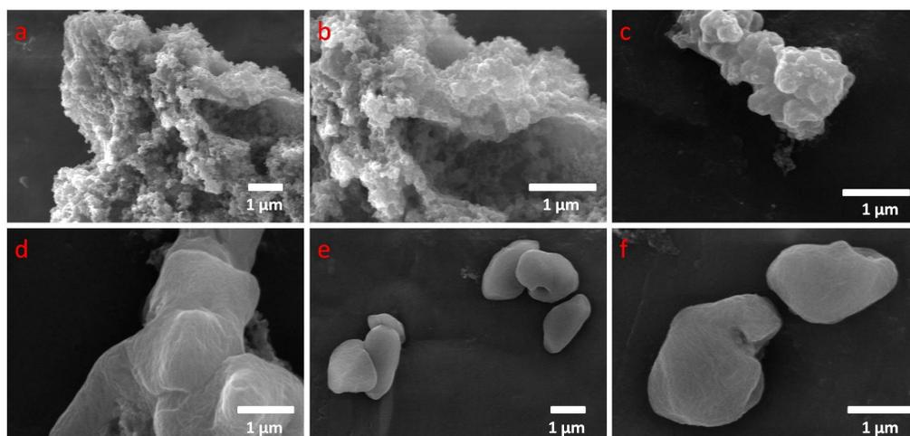
Figure S3 SEM of the S@NiS<sub>2</sub> composite (a, b), amorphous NiS<sub>2</sub> (c, d) and crystal NiS<sub>2</sub> (e, f).
