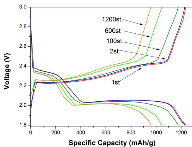
Figure S6 The voltage profiles during the 1200 cycles (Fig. 5a), containing 1st, 2nd, 100th, 600th, and 1200th.
