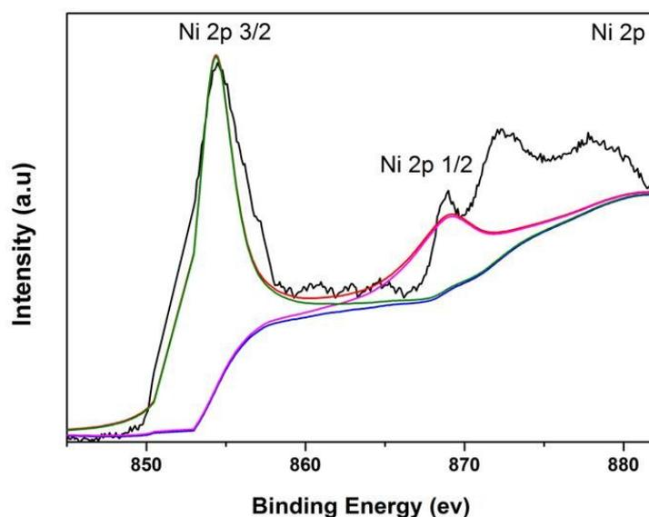
Figure S1 The Ni 2p core-level XPS spectrum.
