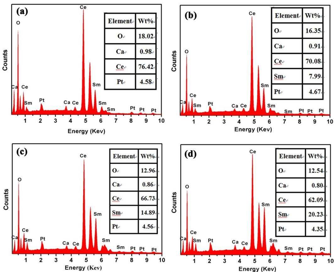
Fig. S1 The EDS spectra of Sm and Ca co-doping ceria with different Sm contents.
