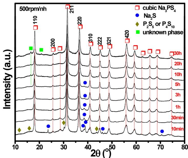
**SI Figure S1.** Powder XRD patterns of 75Na<sub>2</sub>S-25P<sub>2</sub>S<sub>5</sub> samples synthesized by ball milling at rotation speed of 500 rpm for different milling time.
