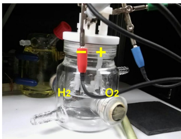
Figure S11 Photograph of two-electrode electrochemical cell for overall water splitting
